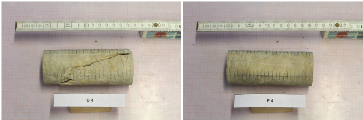
Fig. 4.6: Comparison of fracture pattern of untreated (left picture) and treated (VCM with KSE 300E, right picture) specimen after uniaxial compression test
