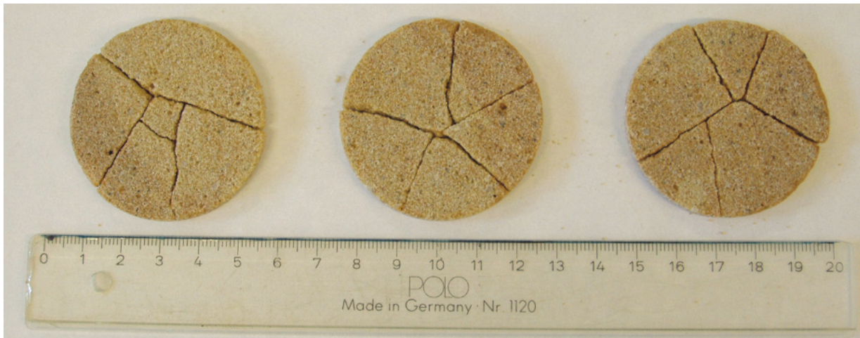
Fig. 4.7: Typical fracture pattern of specimen after biaxial flexural test
