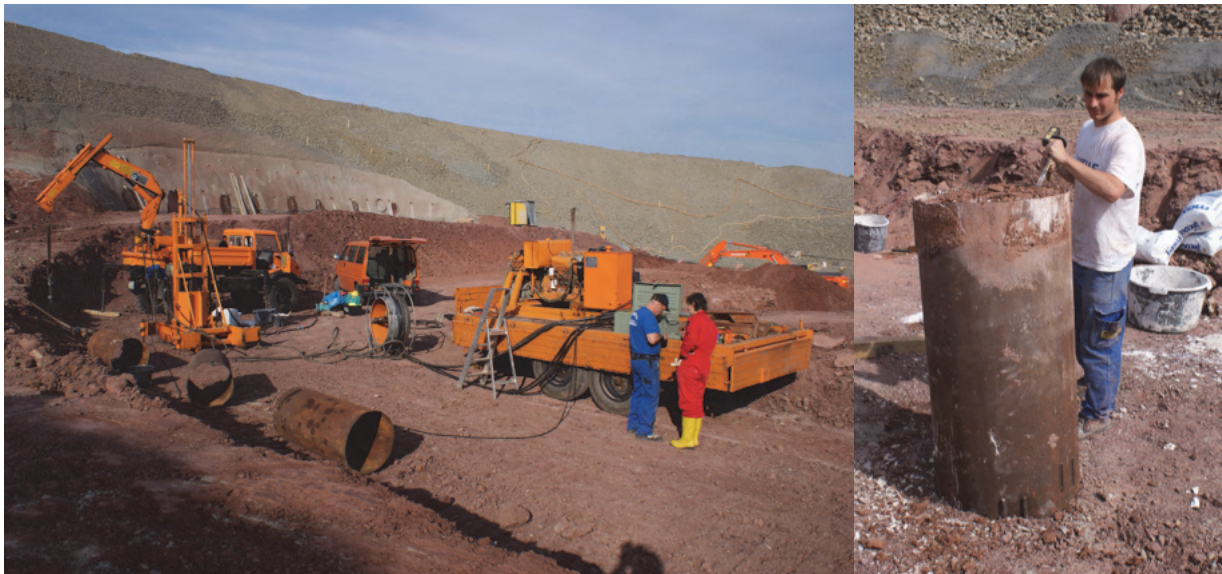
Fig. 1.1: Sampling equipment (left), flattening of the bottom of the sample (right)
