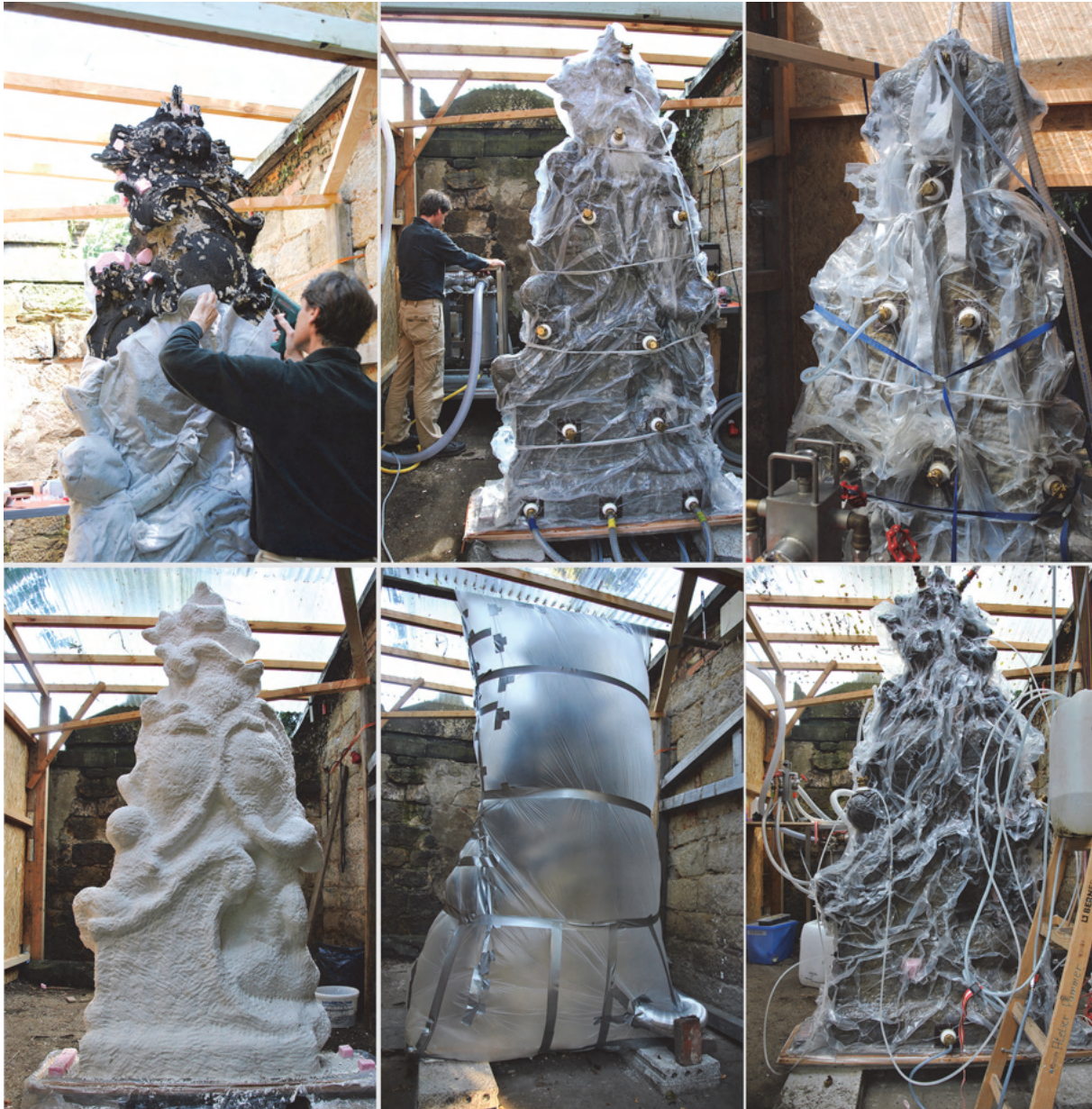
Fig. 3.2: Treatment of the tombstone with VCM from upper left to lower right: Covering with fleece for protection, desalting by flushing water through the tombstone; covering with a compress for final desalting; drying; consolidation.
