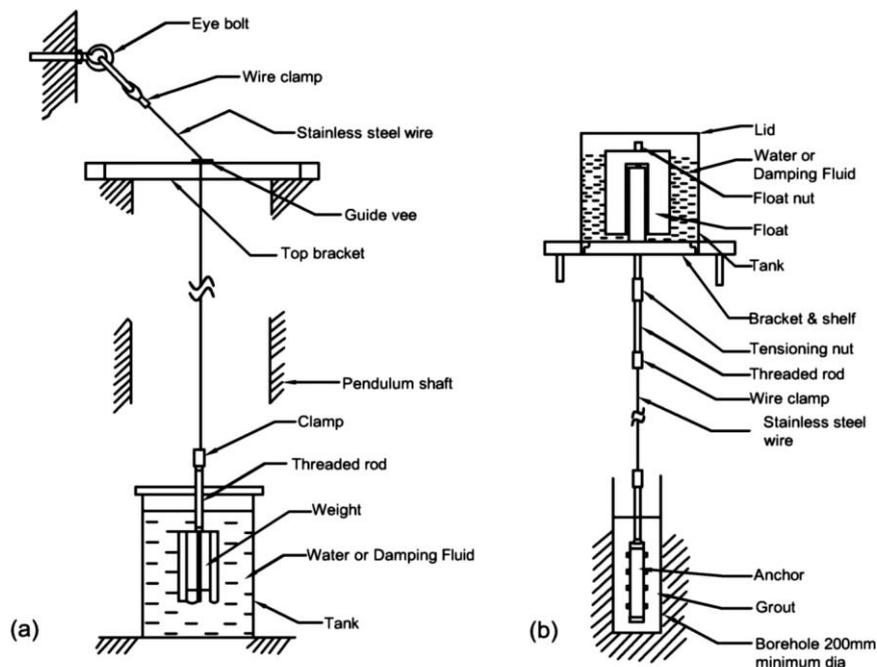
**Fig. 7.1:** Weighted plumbline (left) and float-supported plumbline (right) (CWC, 2018)
