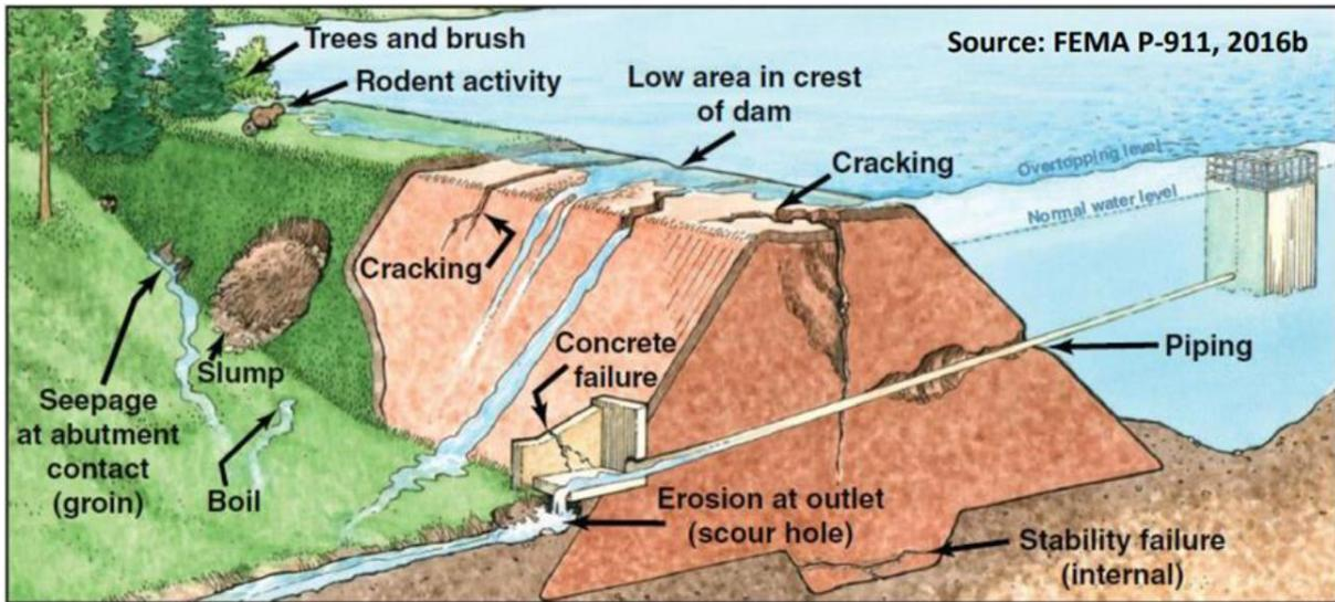
Fig. 8.1: Illustration of typical modes of water dam failures (CRS, 2019)
