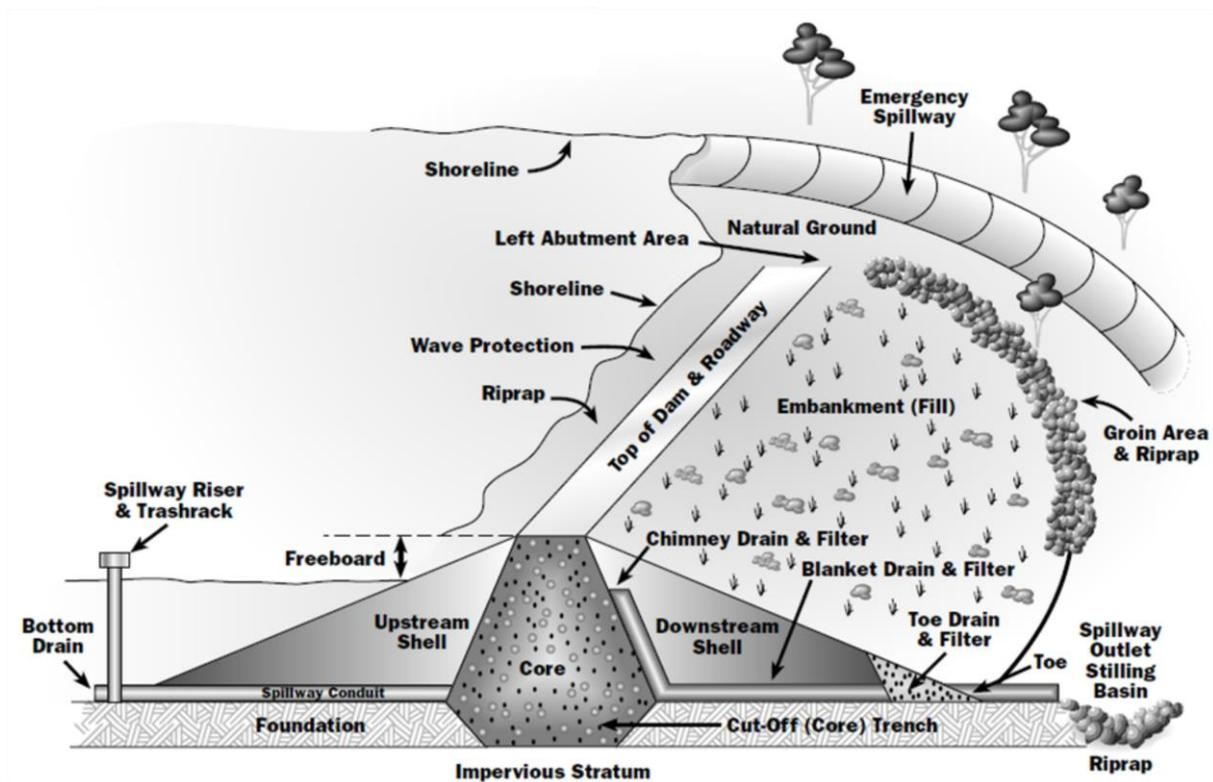
Fig. 1.4: Dams: basic construction and technical terms (TCEQ, 2011)
