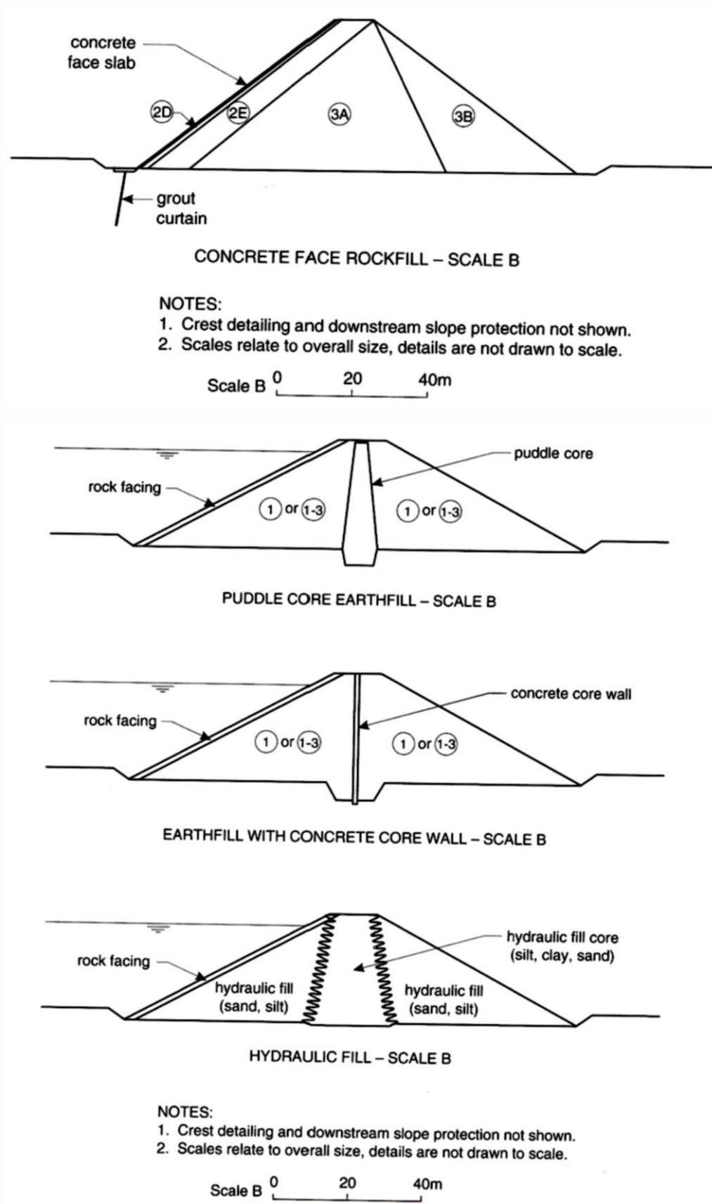
Fig. 4.2 (III): Typical embankment dam structures (Fell et al., 2015)
