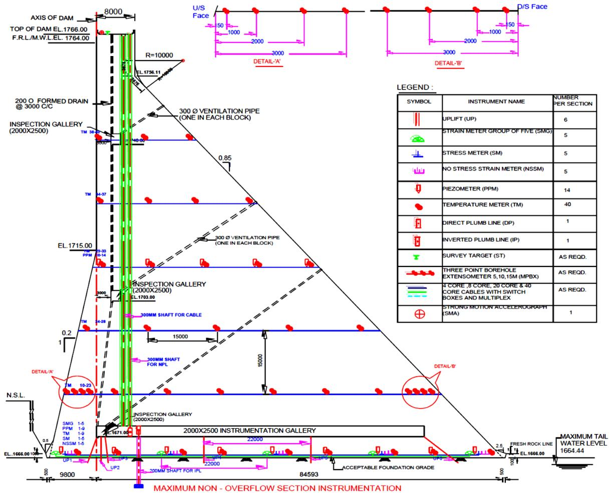
Fig. 7.6: Illustration of a typical monitoring system for a concrete or masonry dam (2) (CWC, 2018)
