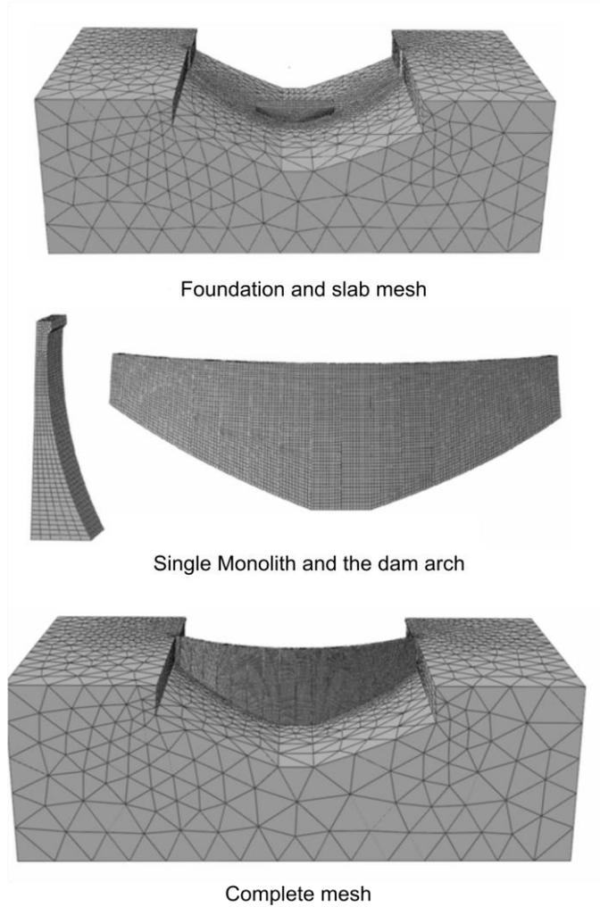
Fig. 5.2: Exemplary 3D numerical dam model (modified after Andersson & Seppälä, 2015)
