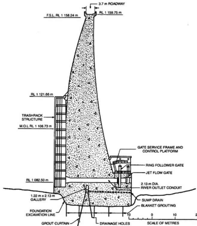
Fig. 3.4: Typical arch dam plan (Fell et al., 2015)
