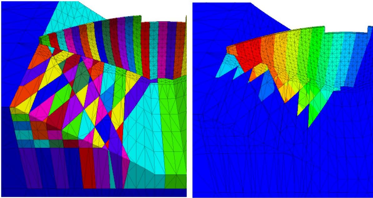
**Fig. 5.3:** Exemplary: 3D numerical dam model with explicit consideration of rock joint pattern using Discrete Element Method (Lemos, 2012)
