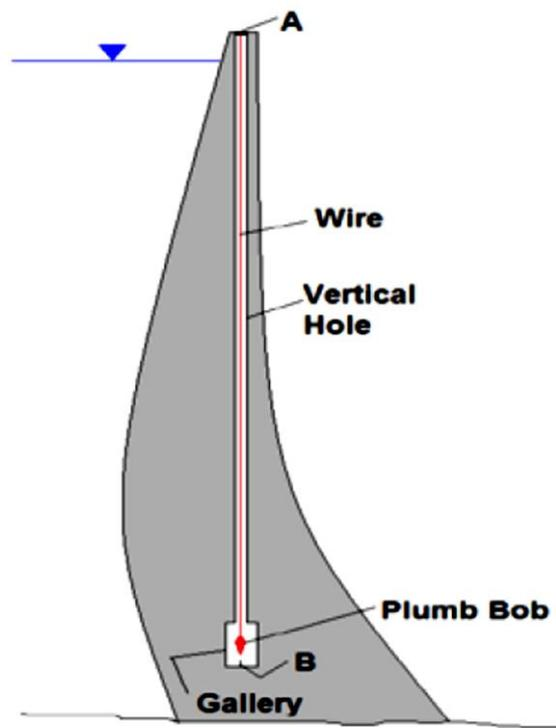
Fig. 7.2: Plumbline installed in an arch dam (FERC, 2018)
