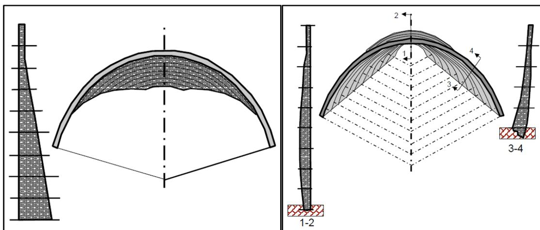
Fig. 3.2: Sketch illustrating different types of arch dams (Yurtal, 2020)
