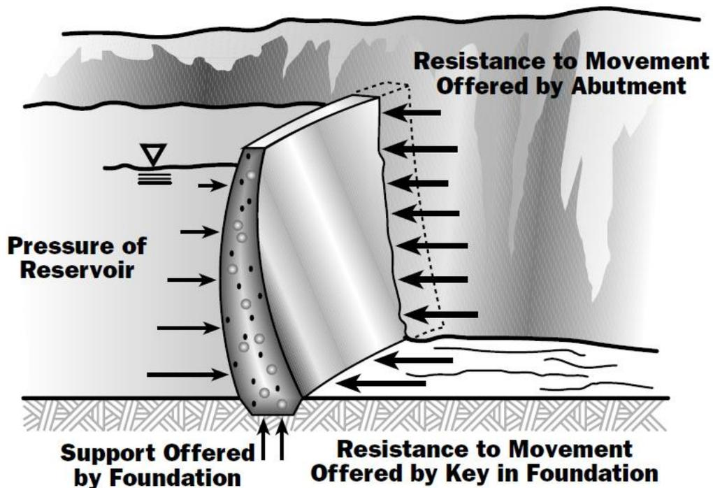
Fig. 3.3: Simplified sketch to illustrate the force situation for an arch dam (TCEQ, 2011)
