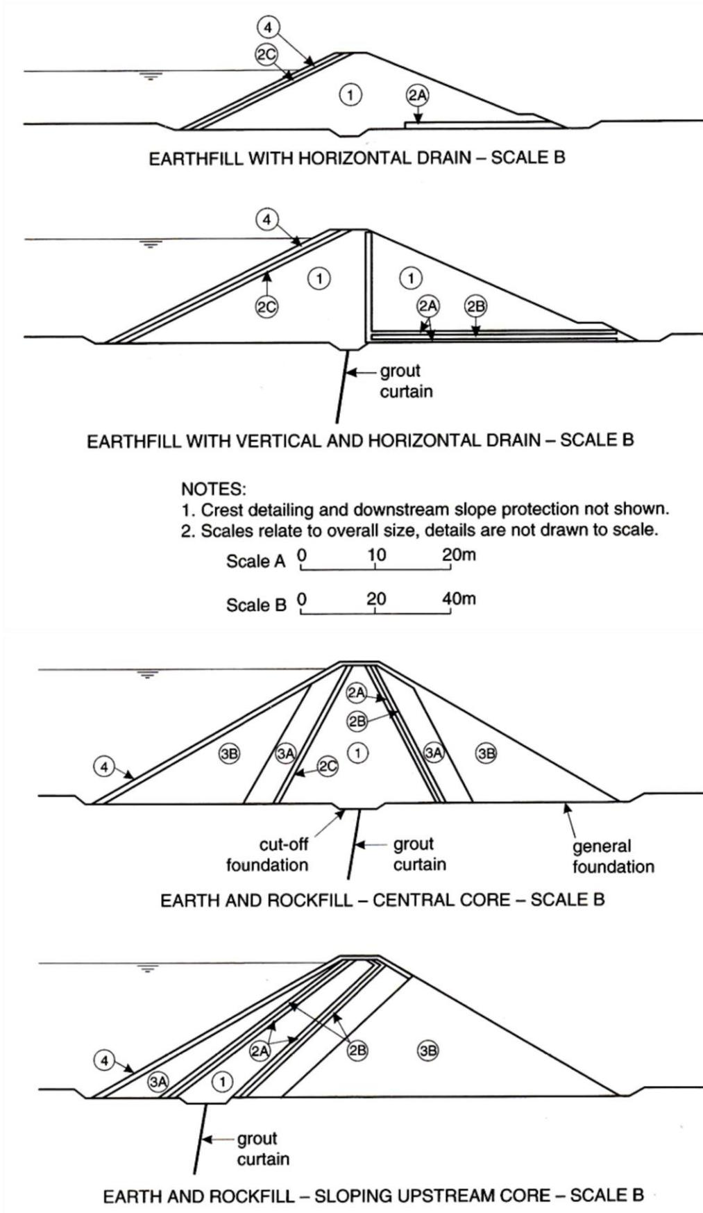
Fig. 4.2 (II): Typical embankment dam structures (Fell et al., 2015)
