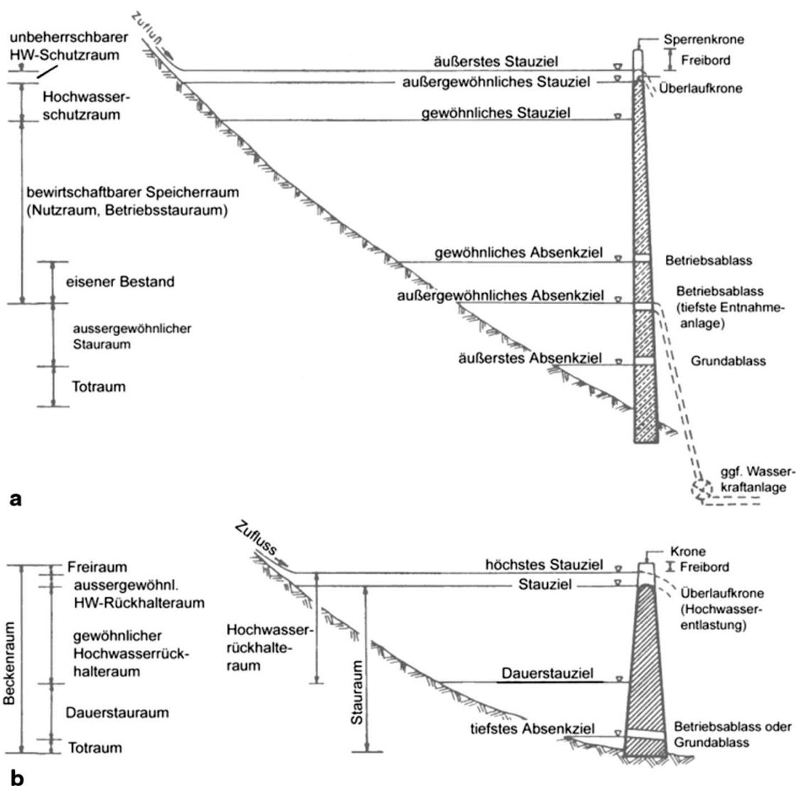
**Fig. 6.1:** Devision of reservoir space and operation levels according to German regulations (Maniak, 2016)
