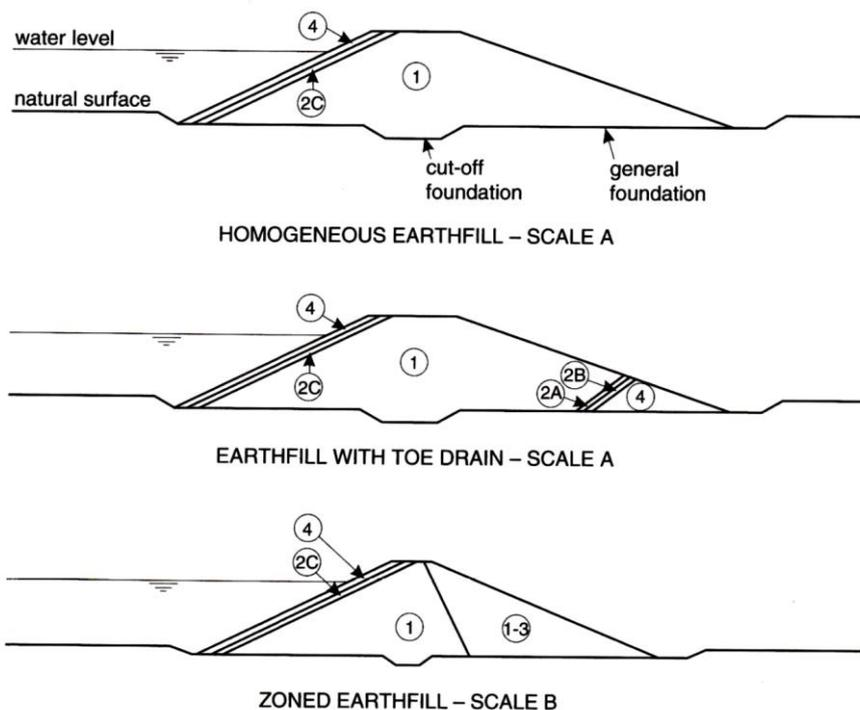
**Fig. 4.2 (I):** Typical embankment dam structures (Fell et al., 2015)
