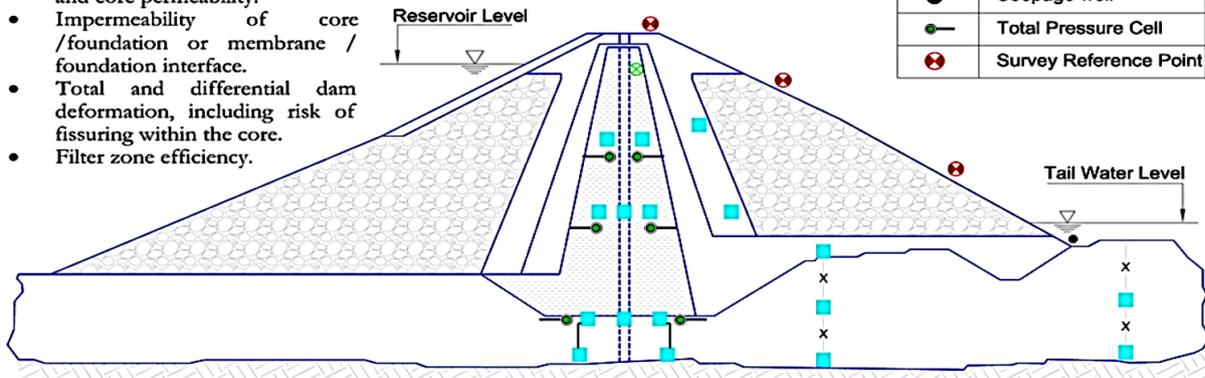
**Fig. 7.4:** Illustration of a typical monitoring system for an embankment dam (CWC, 2018)
