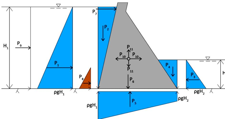
1. Hydrostatic pressure (P1-P2) – depends on the water level in the dam
