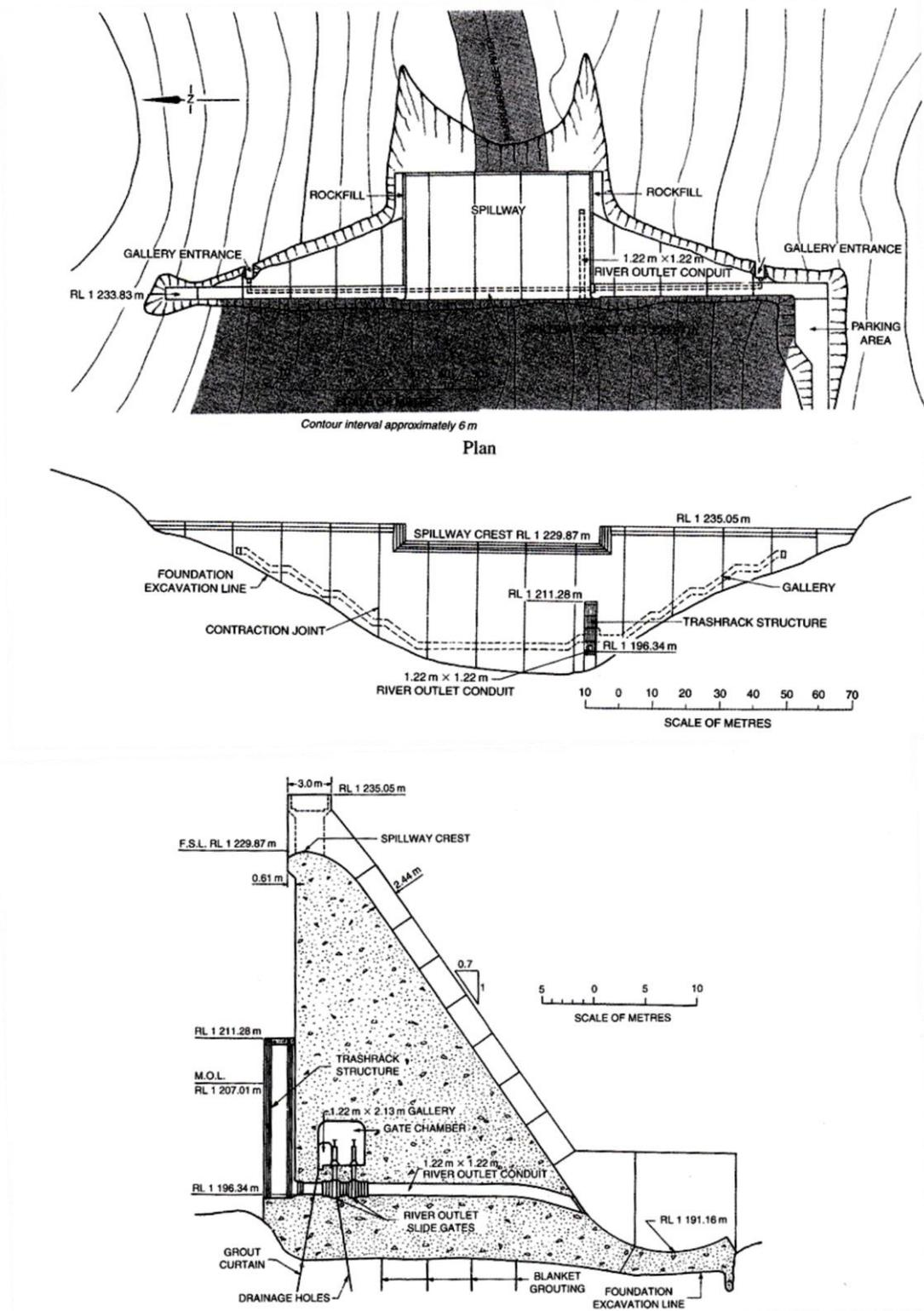
Fig. 2.2: Typical concrete gravity dam plan (Fell et al., 2015)
