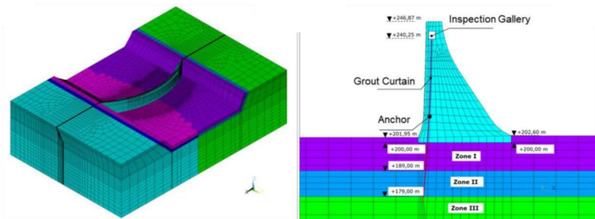
Fig. 5.3: Exemplary 3D numerical dam model (Schlegel et al., 2017)
