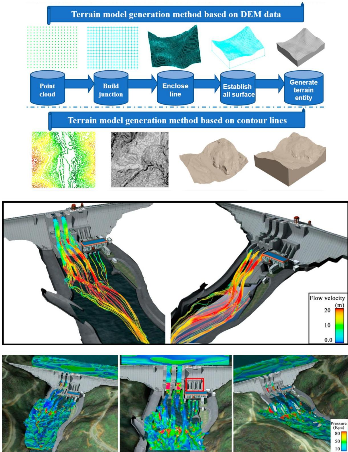
**Fig. 5.6:** Exemplary: Set-up of Digital Elevation Model (top); Local flow pattern in terms in flow velocity (middle) and water pressure (bottom) (Rong et al., 2019)
