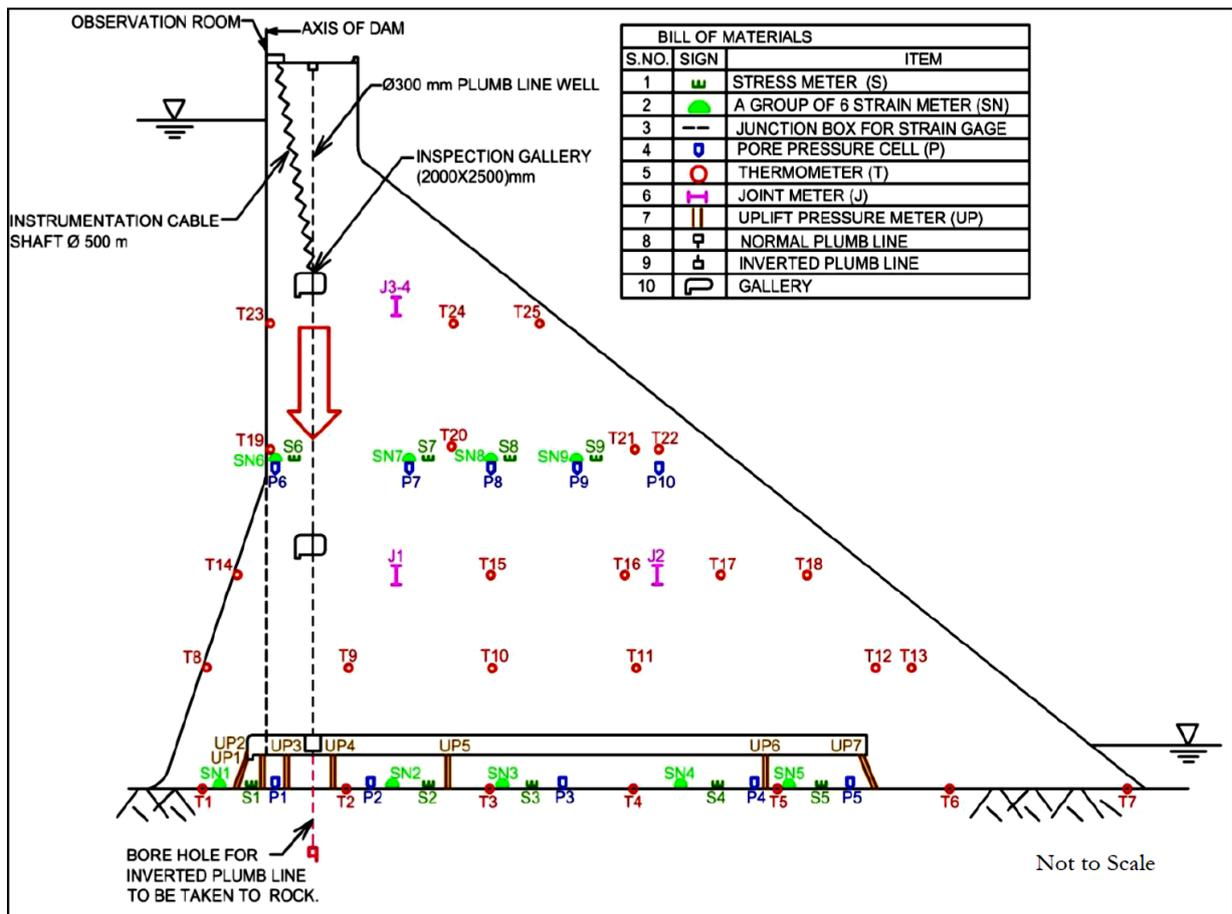
**Fig. 7.5:** Illustration of typical a monitoring system for a concrete or masonry dam (CWC, 2018)
