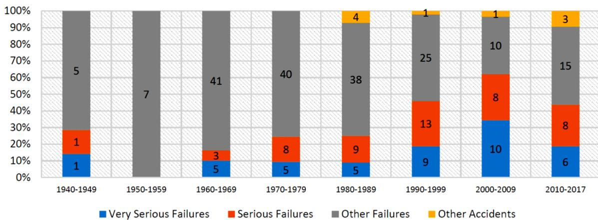
Fig. 8.2: Time-line and severity of global reported tailing dam failures (STINGS, 2018)
