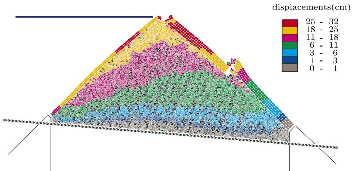
**Fig. 5.4:** Exemplary: 2D numerical model to simulate failure of rockfill dam using particle based Discrete Element Method (Deluzarche & Cambou,2006)
