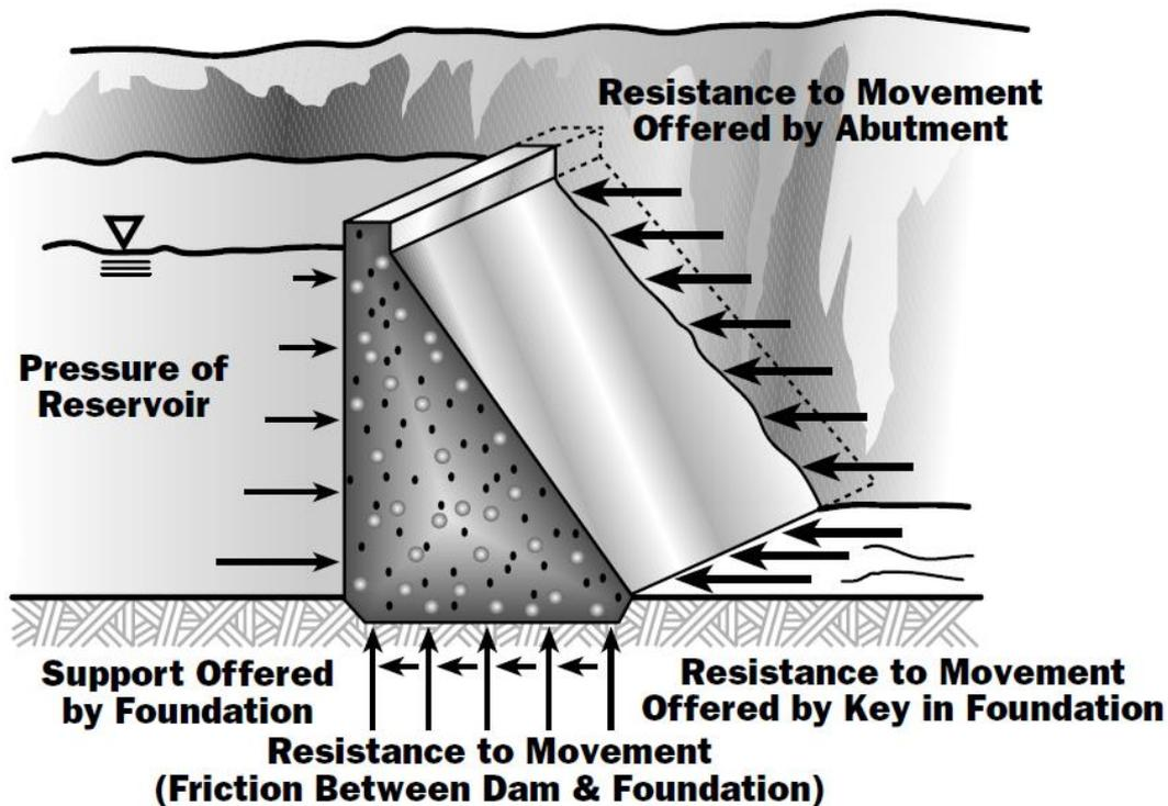
Fig. 2.1: Simplified sketch to illustrate force situation for a gravity dam (TCEQ, 2011)
