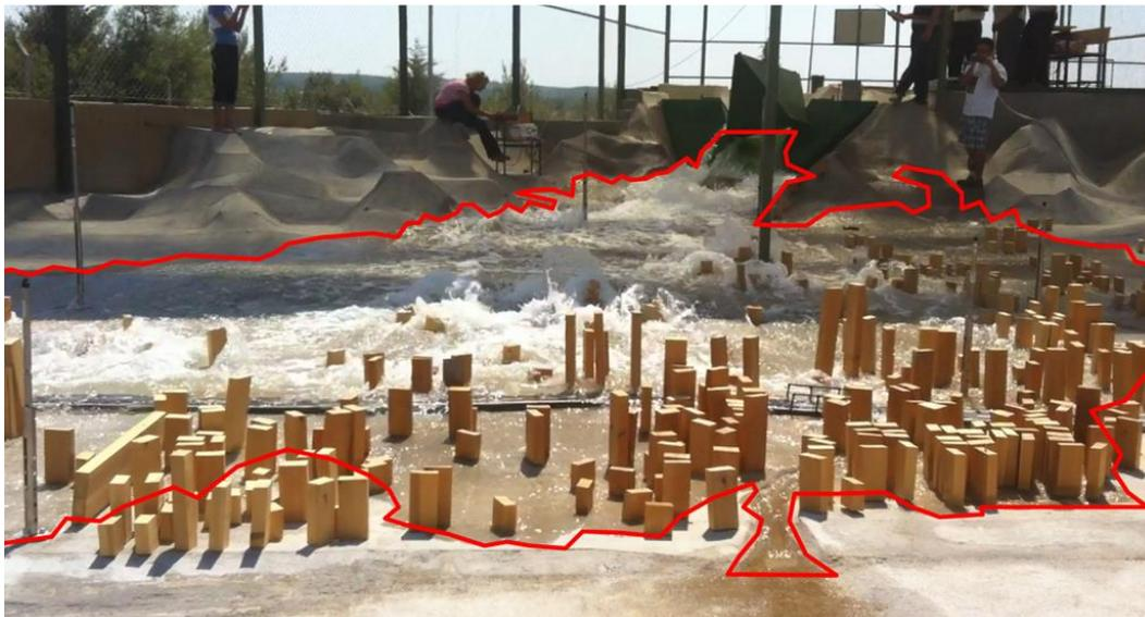
**Fig. 5.5:** Physical model to simulate dam breakage and flooding (Güney et al., 2014)
