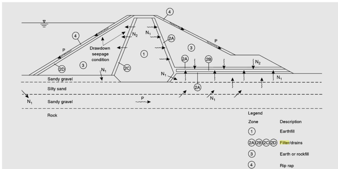
**Fig. 4.1:** Filters and flow conditions (P: flow parallel to interface, N<sub>1</sub>: Flow with high gradient normal to interface, N<sub>2</sub>:Flow with low gradient normal to interface) (Fell et al., 2015)
