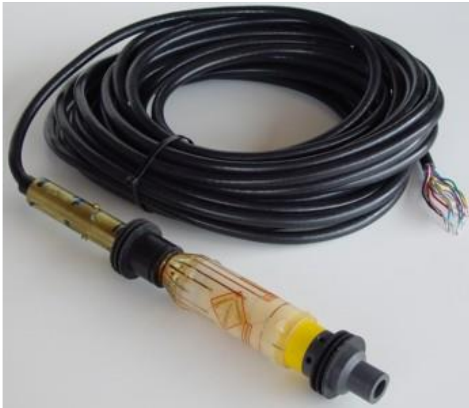
Fig. 4.2: CSIRO-HI-Cell based on over-coring technology (company material)
