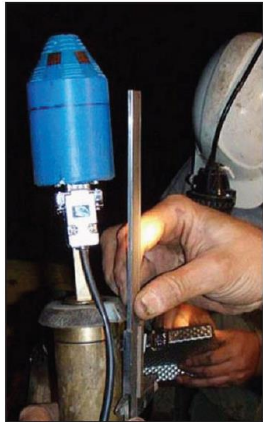
Fig. 4.3: CCBO-Cell based on over-coring technology (Waclawik et al., 2016)
