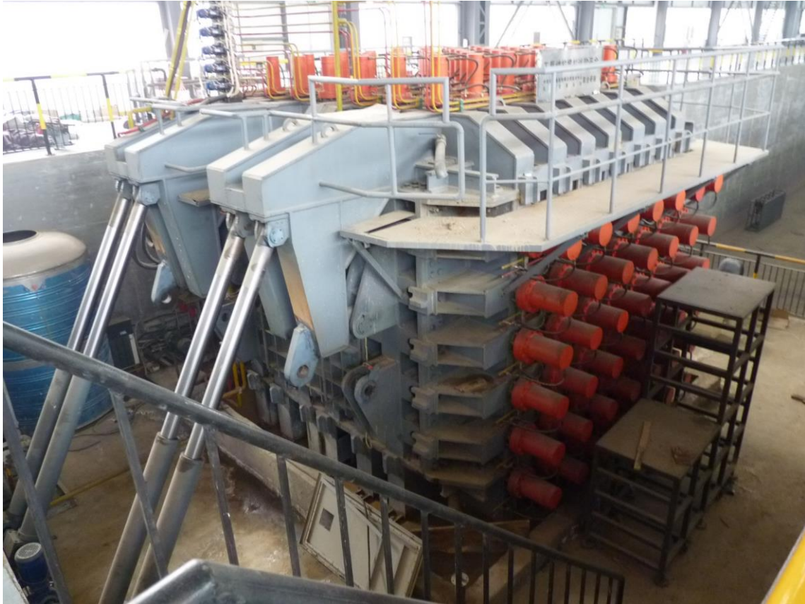
Fig. 5.2: Large scale triaxial device for 3.0 m x 3.0 m x 3.5 m model / sample size (Zhengzhou, China)
