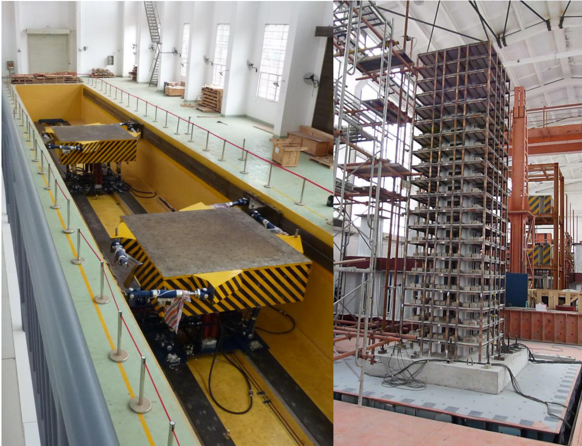
Fig. 5.4: Shaking tables (left) with scaled skyscraper model (China, right)
