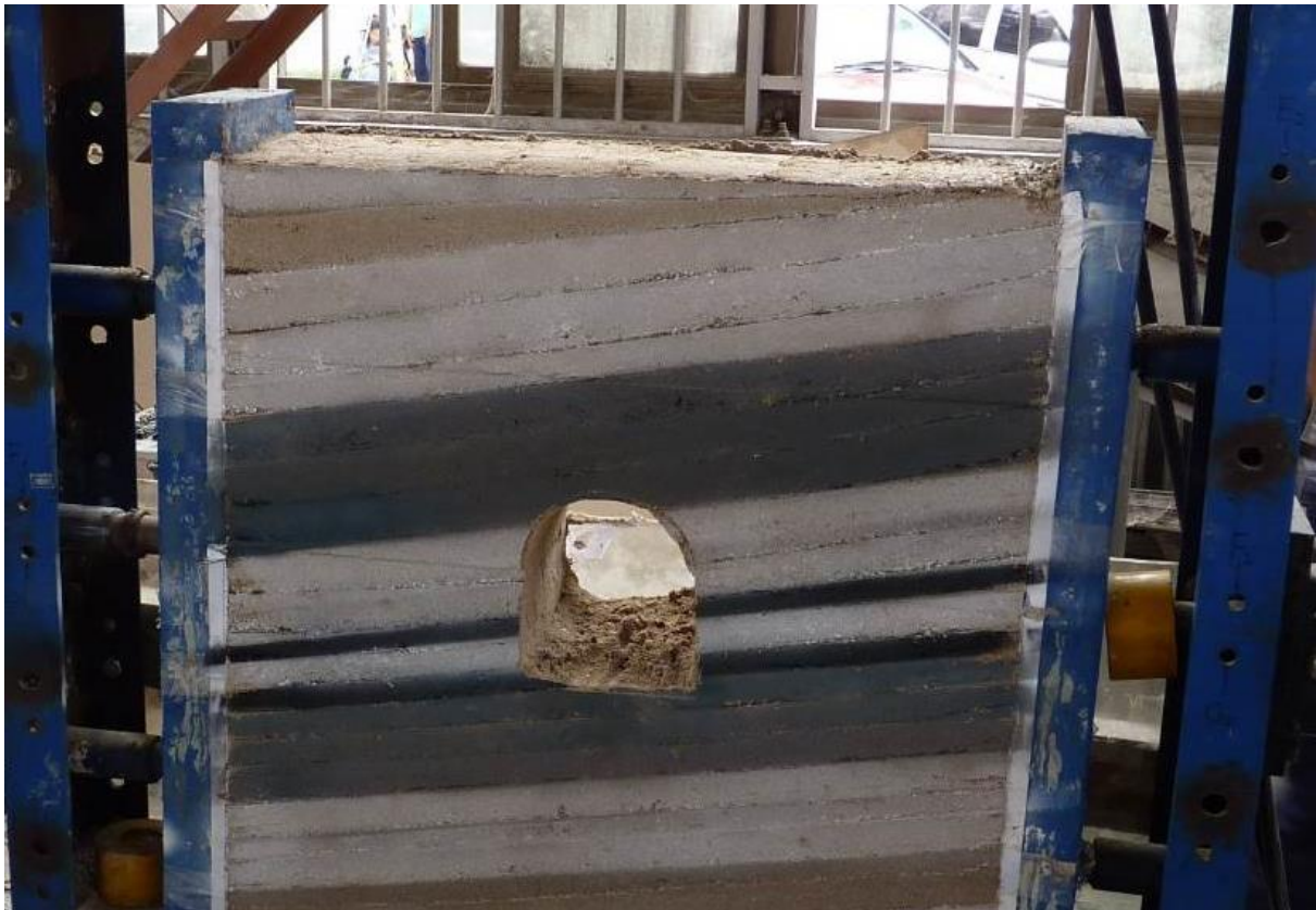
Fig. 4.1: Physical model with inclined layering representing strata with different properties (China)
