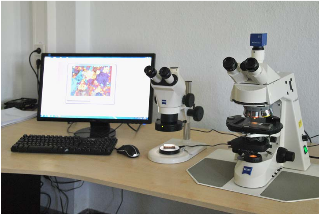
Fig. 5: Polarising microscope Axioscop 40 with digital camera (right) and binocular stereo microscope Stemi 2000-C (left) (RML 2016).
