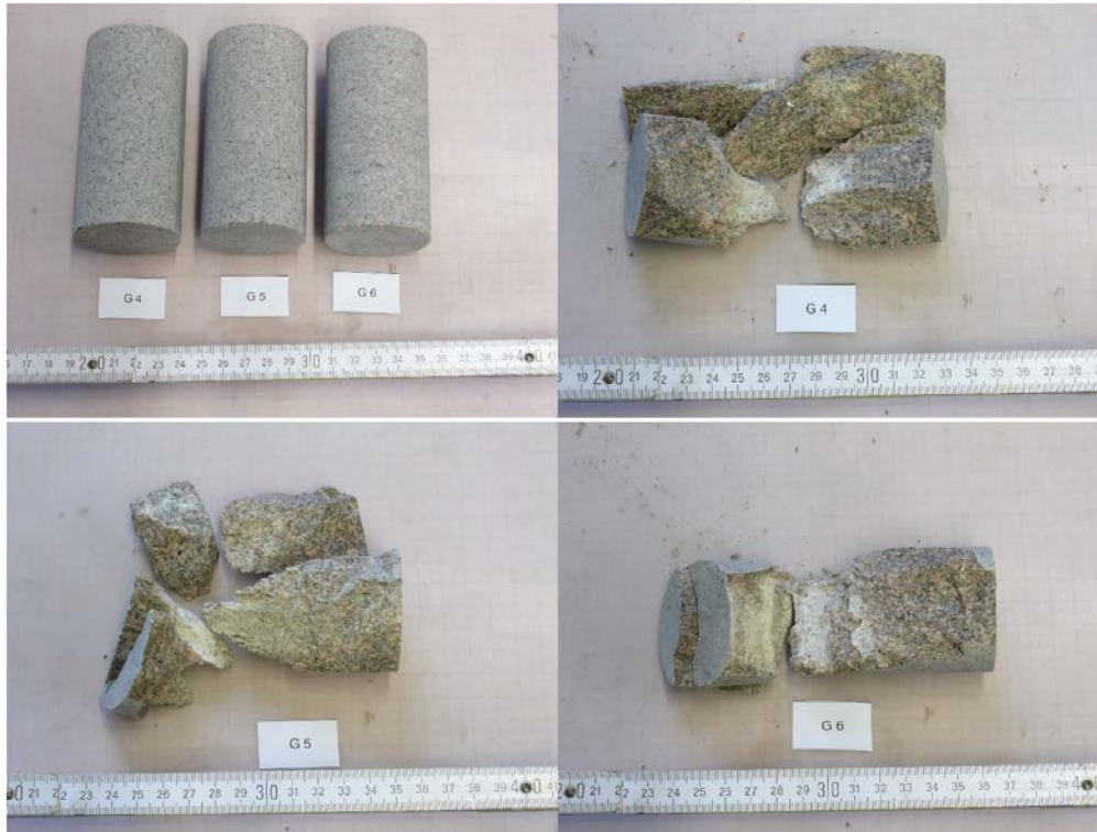
Fig. 1: Granite samples before (top left) and after testing (else) (RML 2016)
