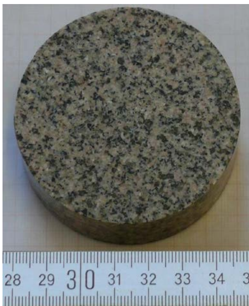
Fig. 2: Granite sample before testing (RML 2016)
