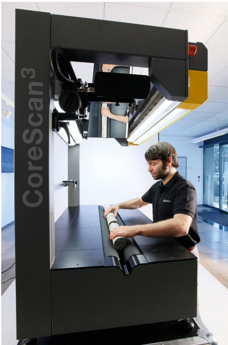
Fig. 3: Core scan device in operation (DMT: company material)
