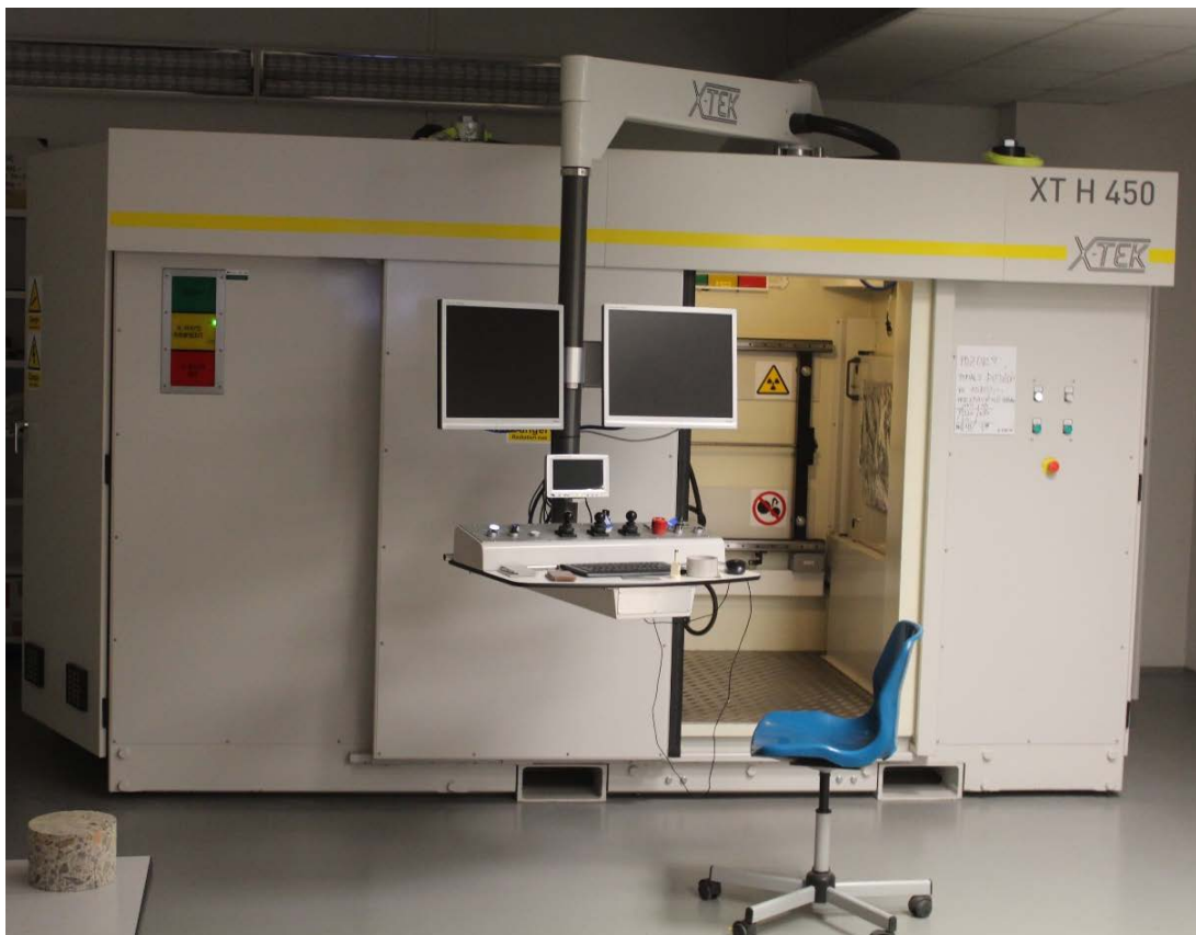
Fig. 9: CT device XT-H-450 (power: 450 keV) (Inst. Geonics, Czech Republic)
