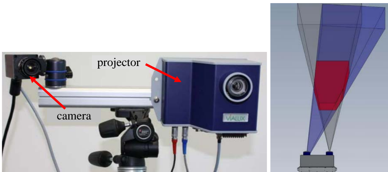
Fig. 20: zSnapper (Vialux 2010) scanning device (accuracy about 20 \mu\text{m} , resolution up to 4.200.000 pixels, field of views up to 1 m, scanning time between 20 and 200 ms), (RML 2016).
