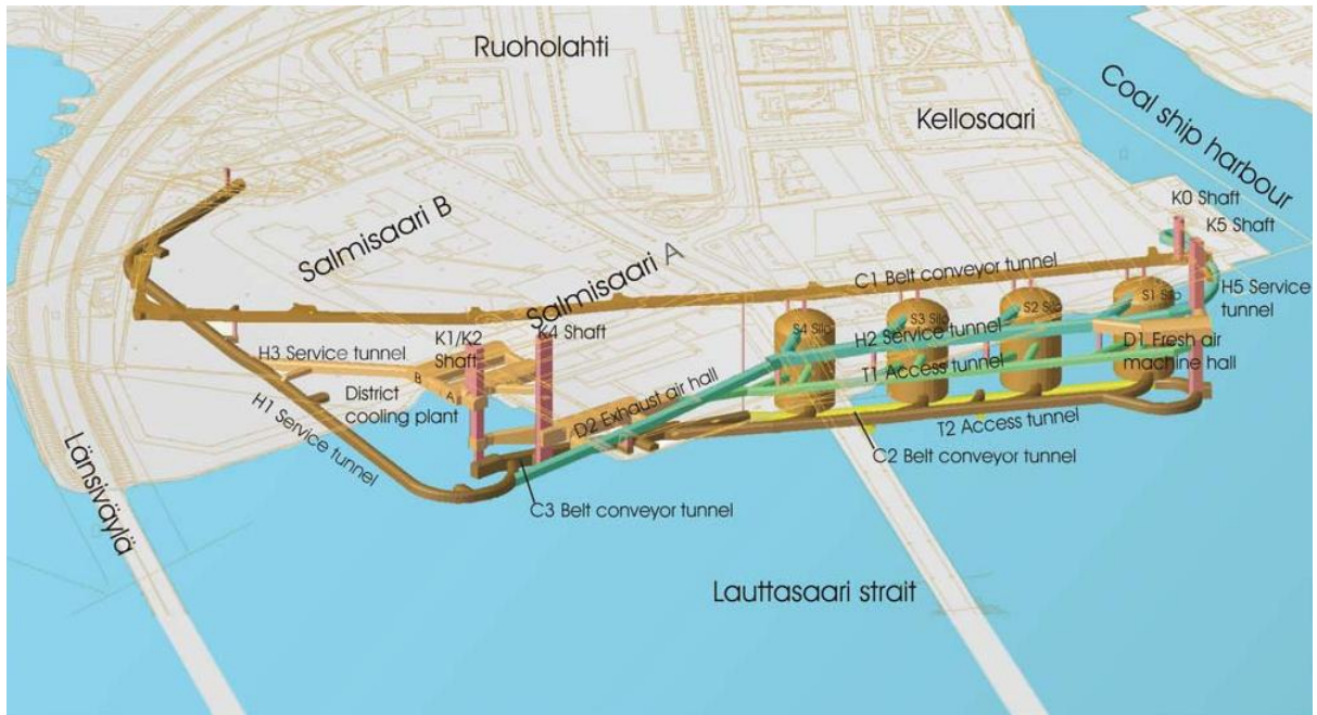
Fig. 7.4: Underground coal storage (Rockplan, 2020)
