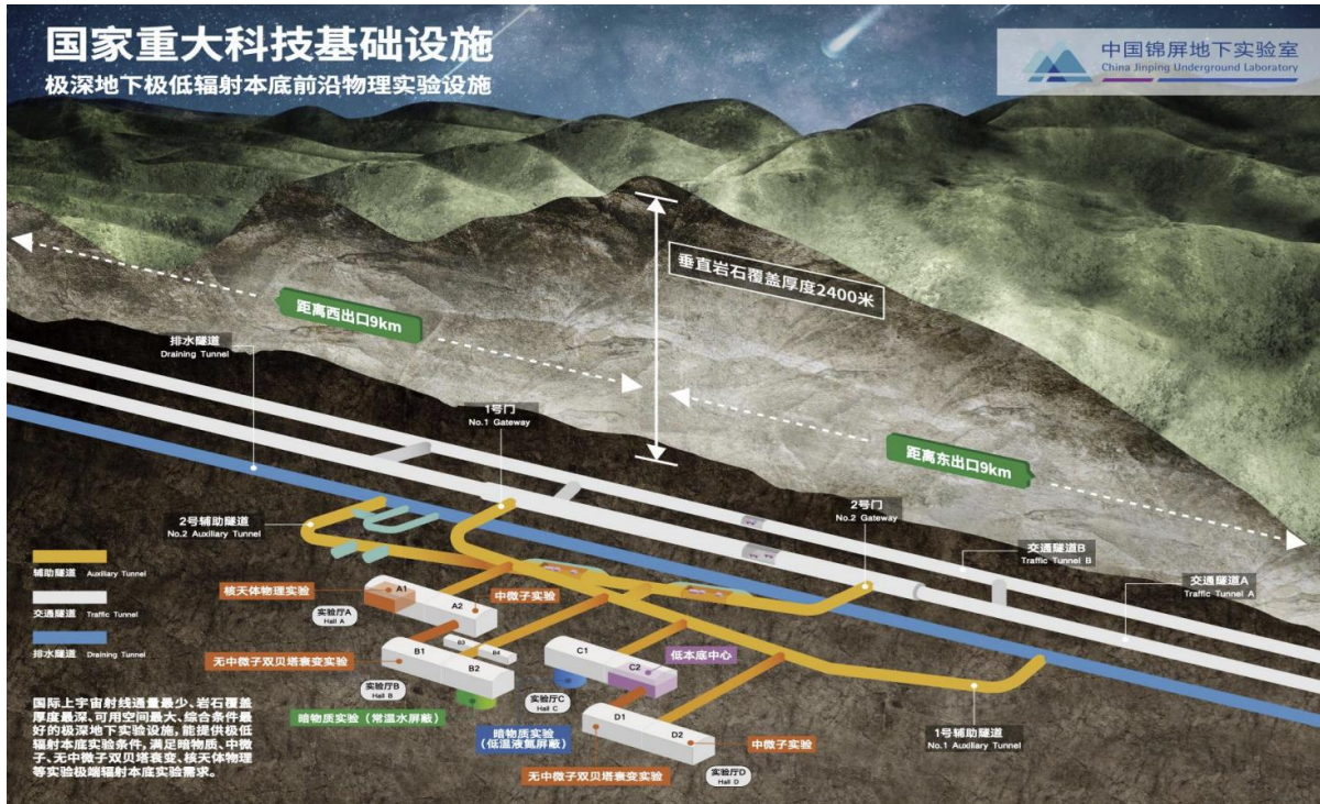
Fig. 9.7: Underground structure of JinPing Underground Research Lab, China (Yue, 2023)
