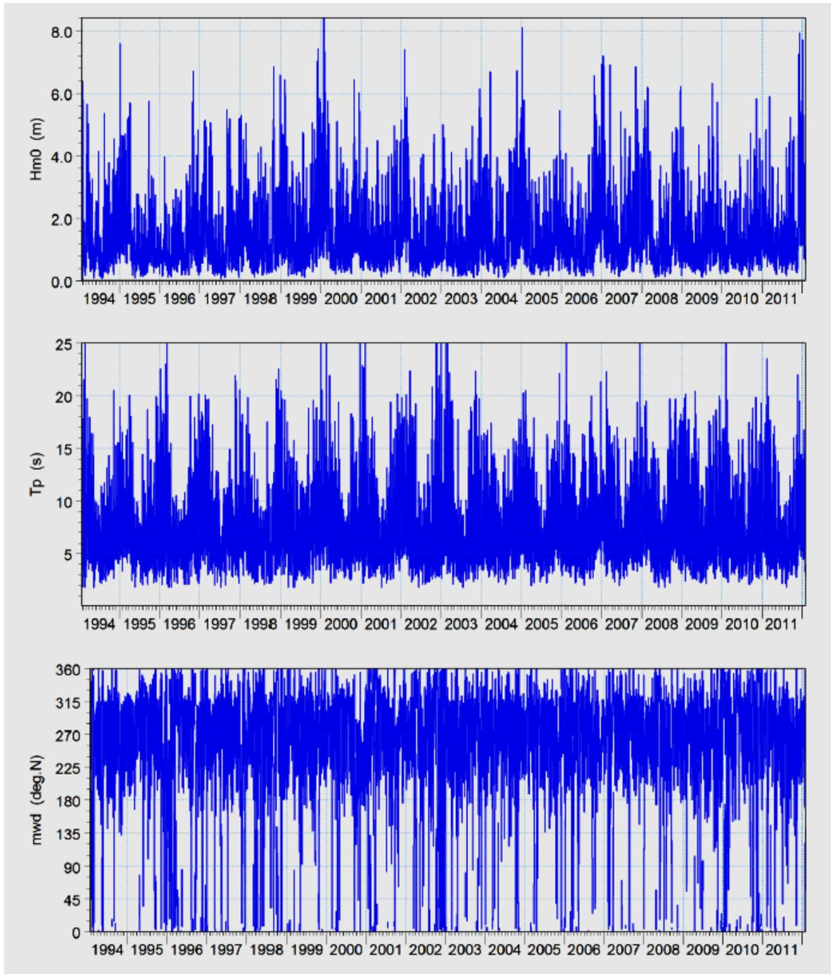
Fig. 2.2: Time series of significant wave height (top), peak wave period (middle) and mean wave direction (bottom) (Mangor et al., 2017)
