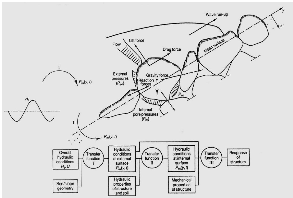
Fig. 9.1: Hydromechanical coupled behaviour of a rocky revetment (CIRIA, 2007)
