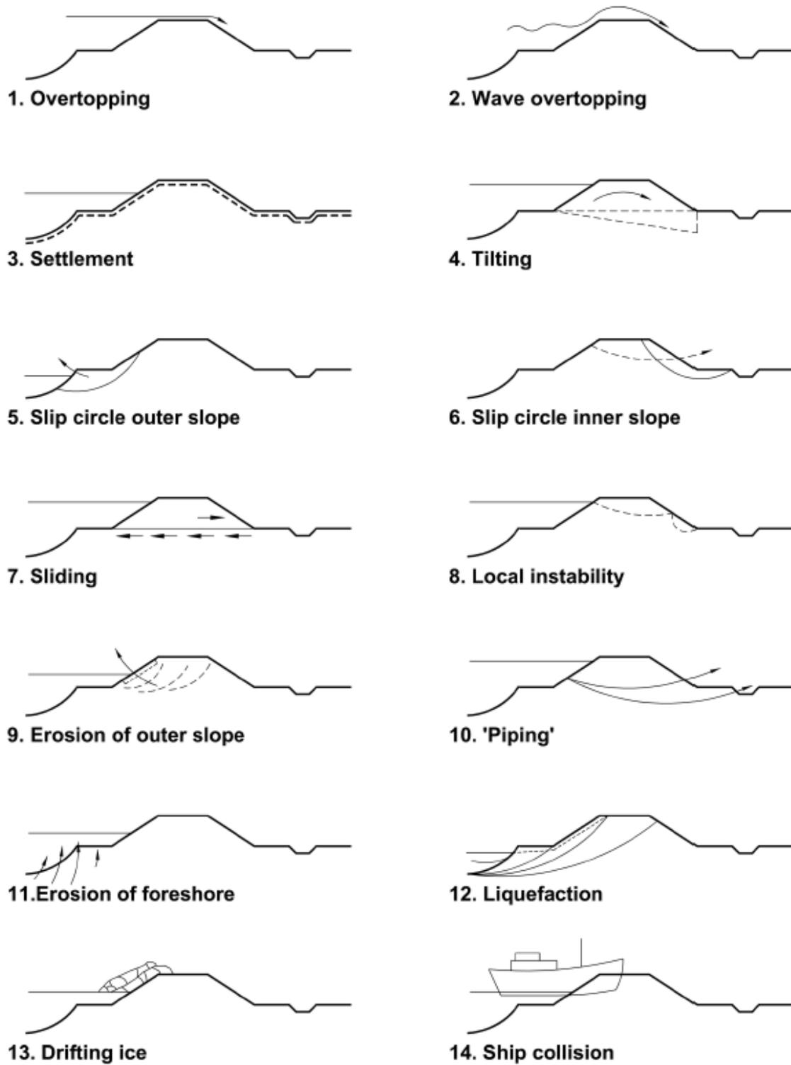
Fig. 9.2: Potential failure mechanisms of rip-rap revetments (CIRIA, 2007)
