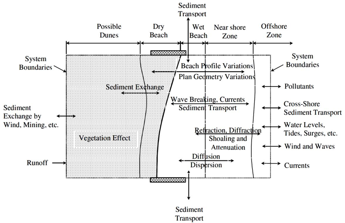
Fig. 1.2: Geotechnical elements of a coastal system (Kamphuis, 2010).
