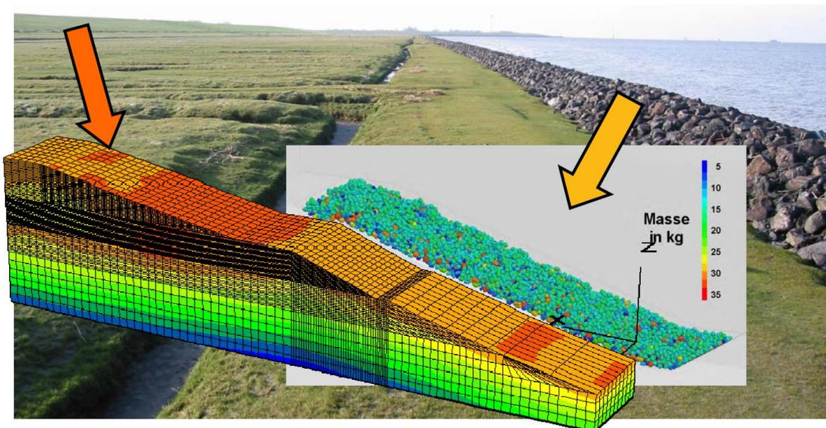
Fig. 9.9: Numerical simulation of rip-rap revetment (Herbst et al., 2010)
