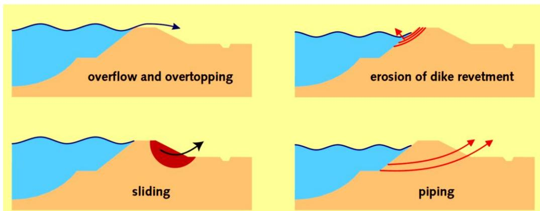
Fig. 4.3: Typical failure mechanisms at the coastline (van Westen, 2005)
