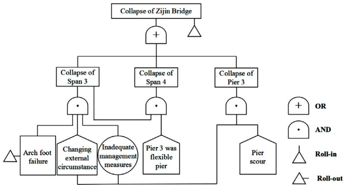
Fig. 4.1.4: Main fault tree of Zijin Bridge collapse (Tan et al. 2020)
