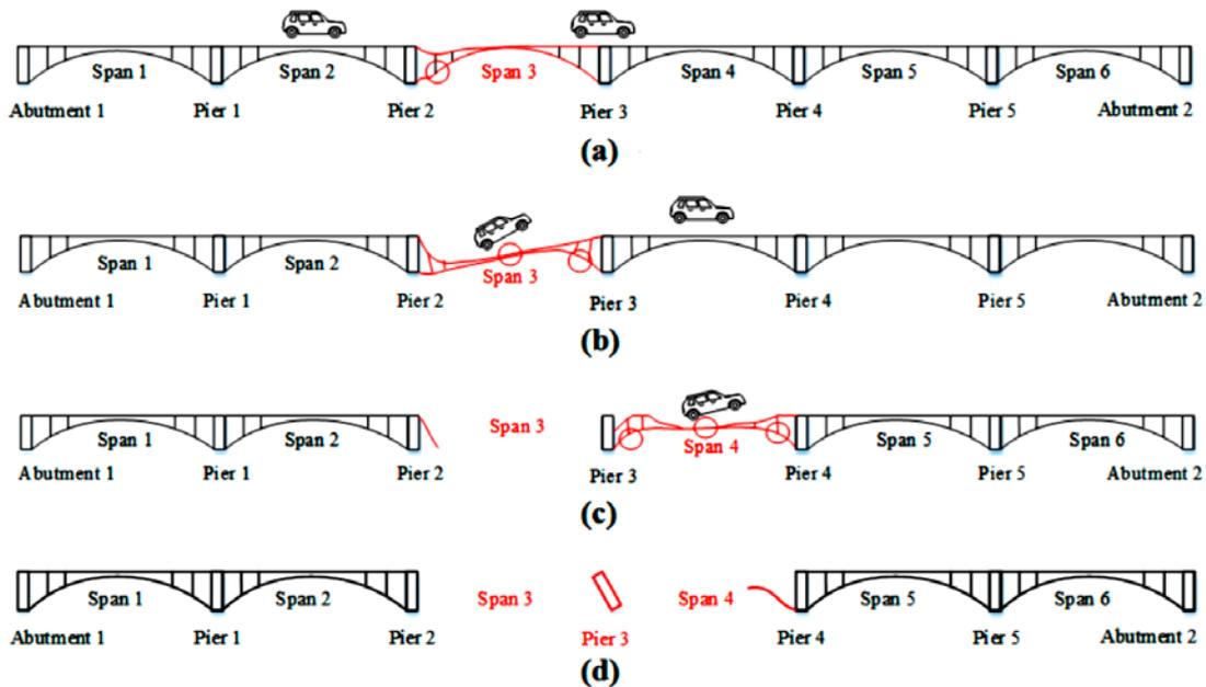
Fig. 4.1.5: Collapse sequence of Zijin Bridge (Tan et al. 2020)
