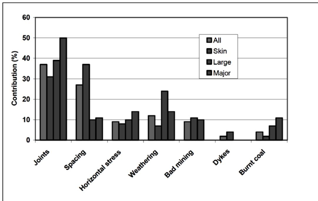
Fig. 4.2.2: Summary of RCA for rock fall events in coal mines in South Africa (van der Merwe et al., 2001)
