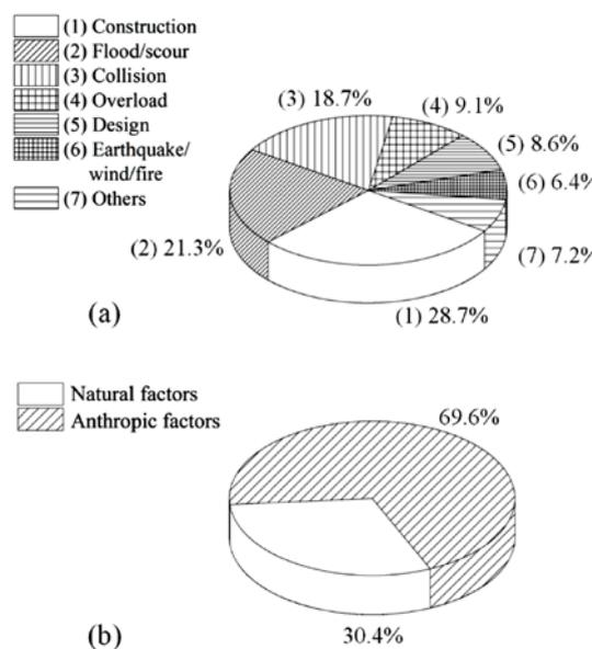
Fig. 4.1.1: Failure causes for bridge collaps (China between 2009 and 2018, Tan et al. 2020)
