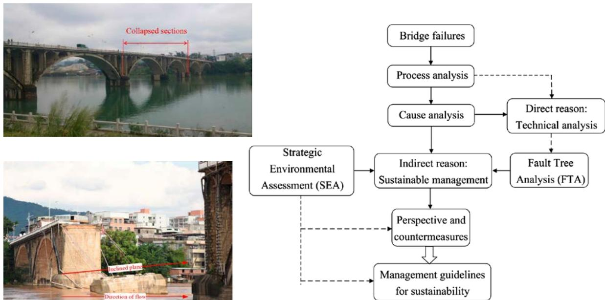
Fig. 4.1.3: Flow chart for RCA for Zijin Bridge (Tan et al. 2020)
