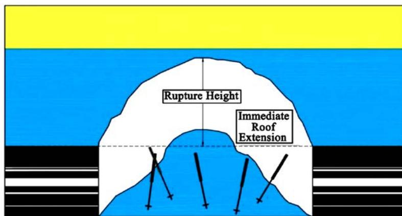
Fig. 4.2.1: Roof fall events a coal mine (Zingano & Andrade, 2021)
