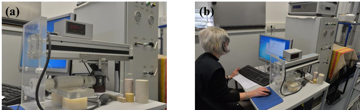
Fig. 3.2: (a) ultrasonic wave speed measurement (b) data acquisition
