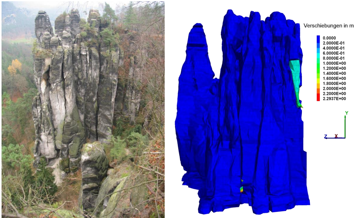
Fig. 27: Sandstone massive (Germany) and corresponding 3D model indicating potential rockfall areas (Herbst & Konietzky, 2012)
