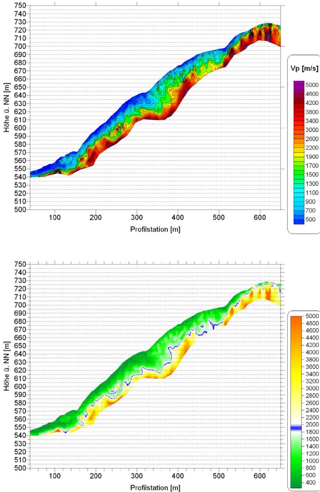
Fig. 6.1: Result of seismic tomography to detect sliding surface shown in blue in lower plot and indicated as boundary between red and green colors in upper plot, seismic velocity values in m/s (Konietzky et al., 2004a,b & TFV, 2007)
