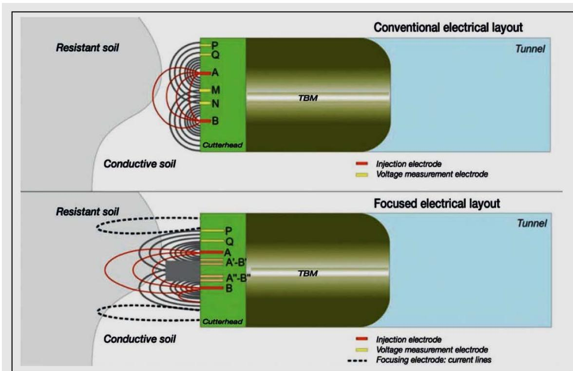
Fig. 5.4: Principles of electrical resistivity based exploration methods while TBM tunneling (AFTES, 2014)
