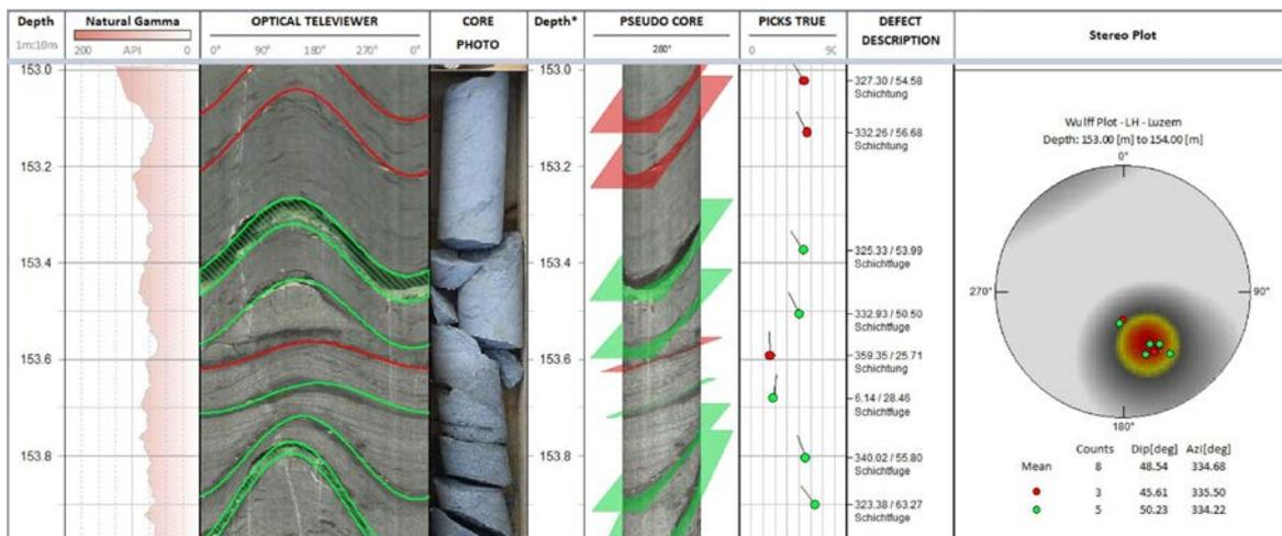
Fig. 9.4: Optical televiewer image indicating stratification (Mount Sopris Instruments: company material)
