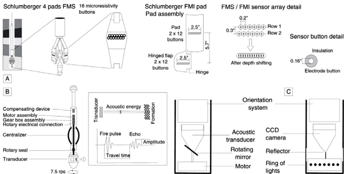
Fig. 9.1: Schematic of electrical (A), acoustic (B) and optical (C) borehole image tools (Gaillot et al. 2007)
