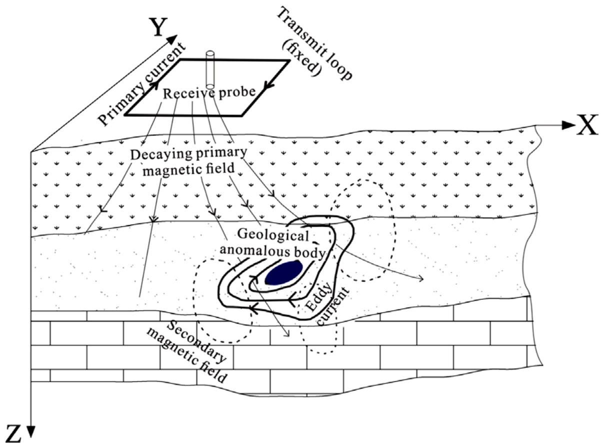
Fig. 4.3: Principle of TEM (Su et al., 2021)
