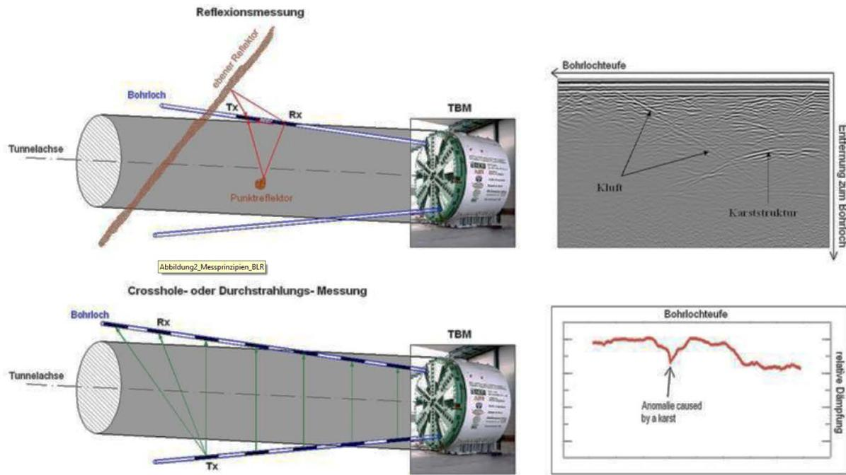
Fig. 5.5: Principle of borehole radar approach in reflection (RX) and cross-hole (CH) mode (Lehmann et al., 2018)
