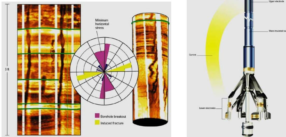
Fig. 9.2: Left: FMI formation image indicating fractures and breakouts, right: FMI tool (Schlumberger: company material)
