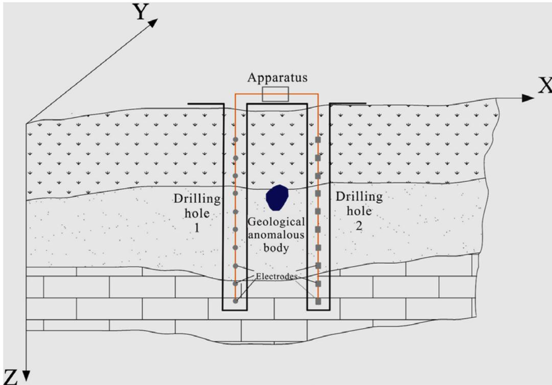
Fig. 4.4: Principle of cross-hole ERT (Su et al., 2021)
