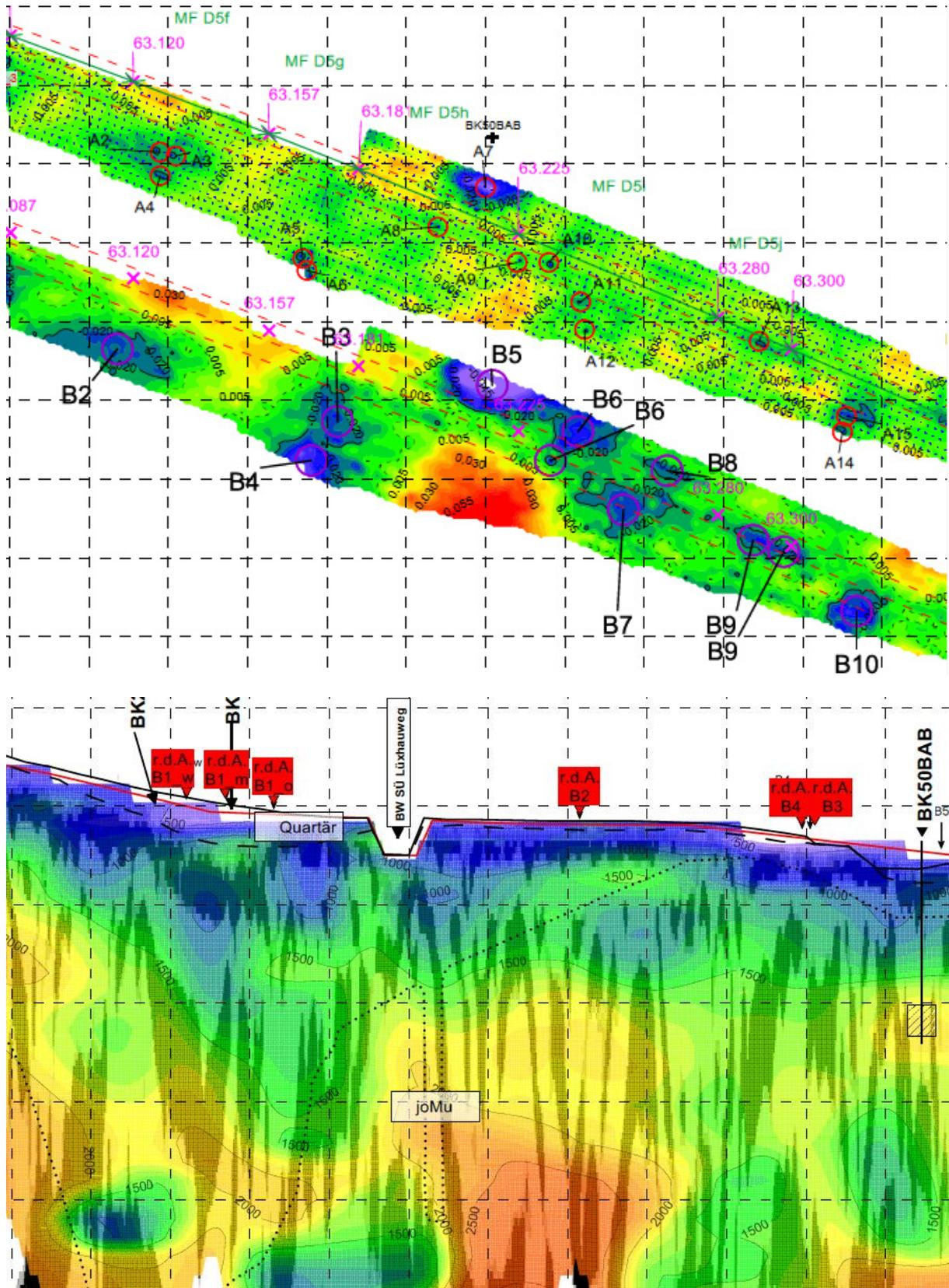
Fig. 4.9: Gravimetric and seismic survey results along the railway route Ulm-Wendlingen indicating karst cavities (Raithel et al., 2016)
