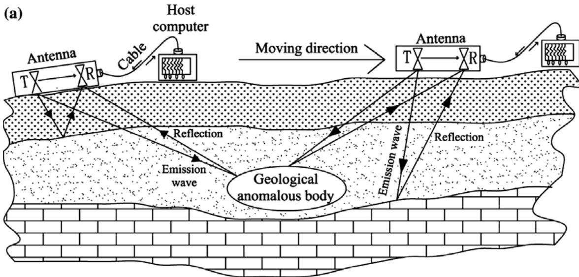
Fig. 4.2: Principle of GPR (Su et al., 2021)
