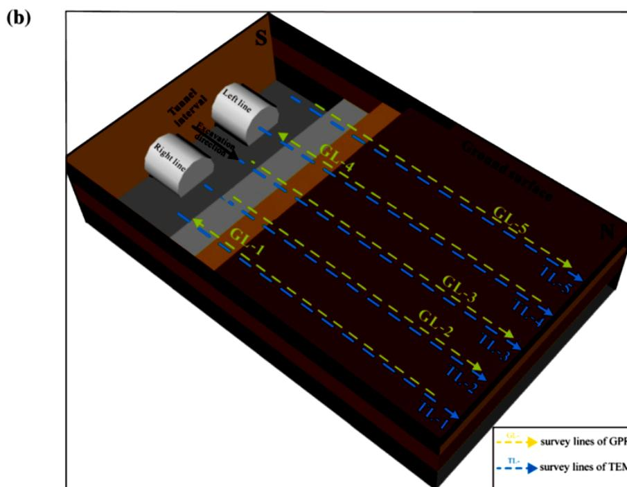
Fig. 4.1: Overview about integrated geophysical approach to detect cavities applied by Su et al. (2021)
