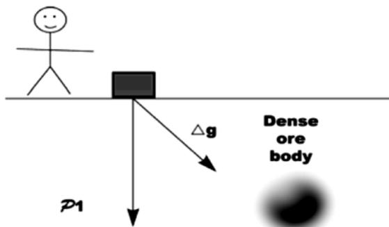
Fig. 3.2.1: Principle of gravimetry
