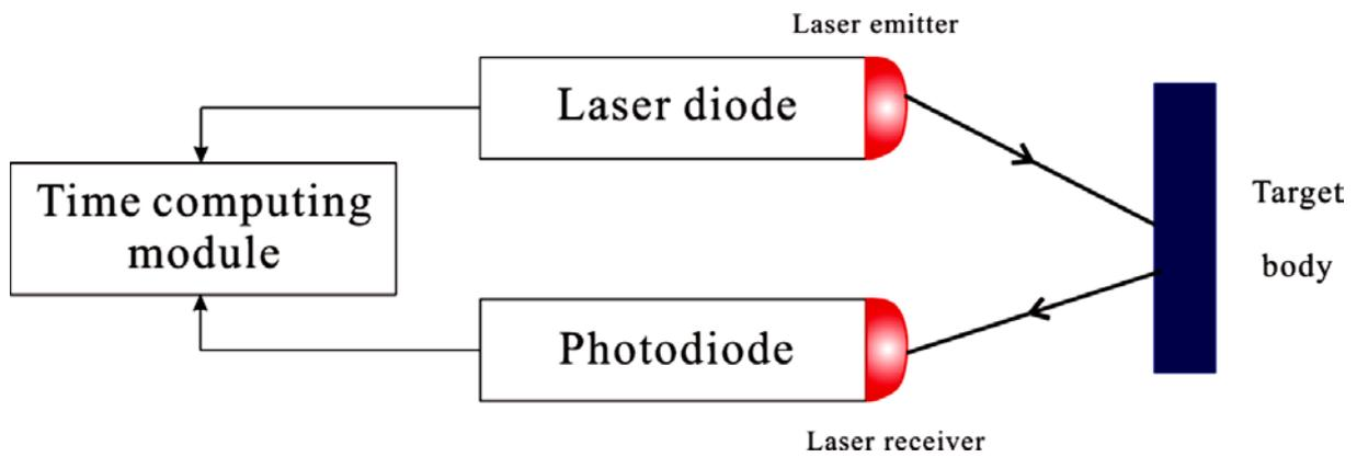
Fig. 4.5: Principle of 3D laser scan (Su et al., 2021)
