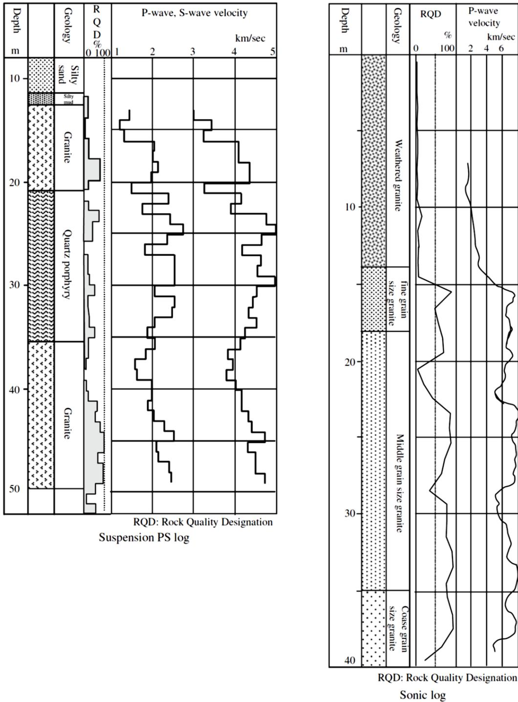
Fig. 7.2: Example for PS logging (P- and S-wave velocities) and Sonic log (high frequency P-wave velocity) (Takahashi et al., 2006)
