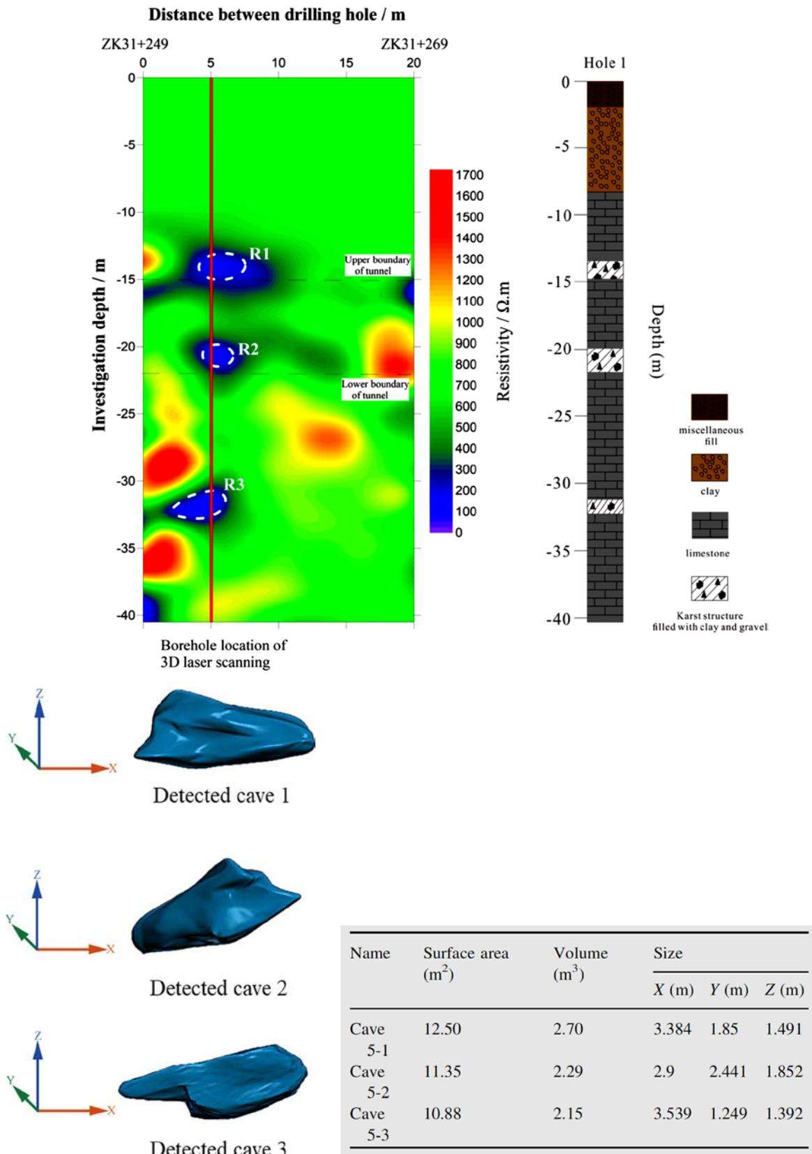
Fig. 4.6: Detected cavities (Su et al., 2021)
