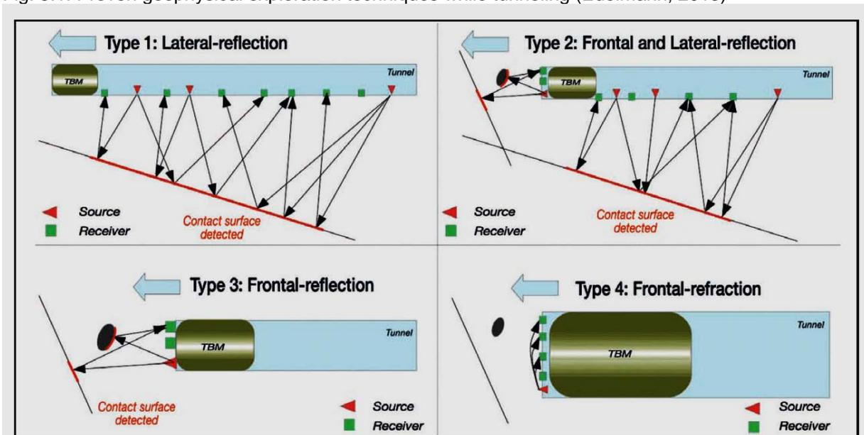
Fig. 5.2: Principles of seismic techniques while TBM tunneling (AFTES, 2014)
