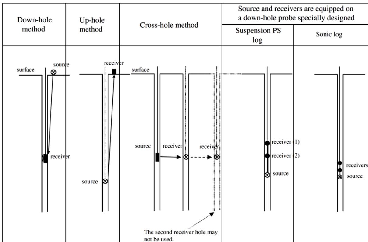
Fig. 7.1: Different set-ups for velocity logging (Takahashi et al., 2006)
