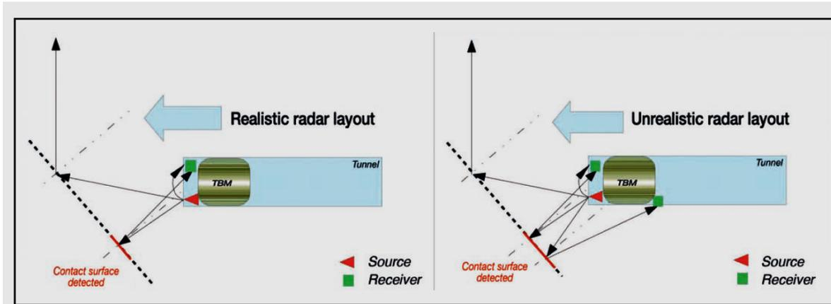
Fig. 5.3: Principles of radar based exploration while TBM tunneling (AFTES, 2014)
