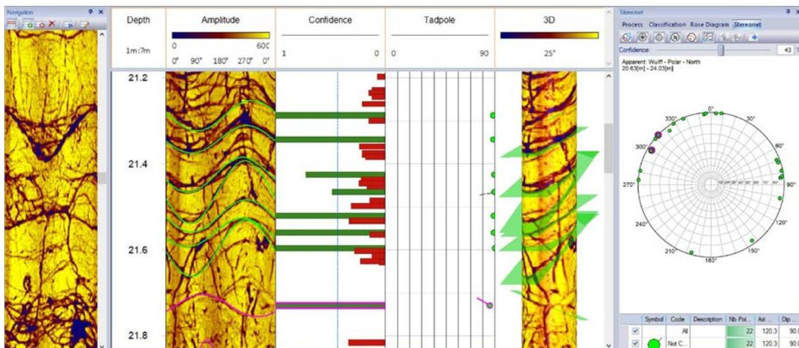
Fig. 9.3: Acoustic televiewer image indicating fractures (Mount Sopris Instruments: company material)
