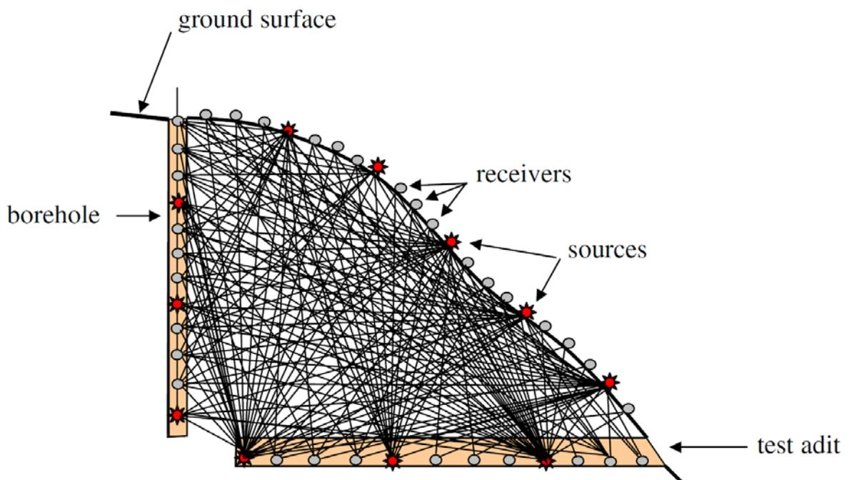
Fig. 7.4: Seismic tomography scheme using borehole and underground drift (Takahashi et al., 2006)
