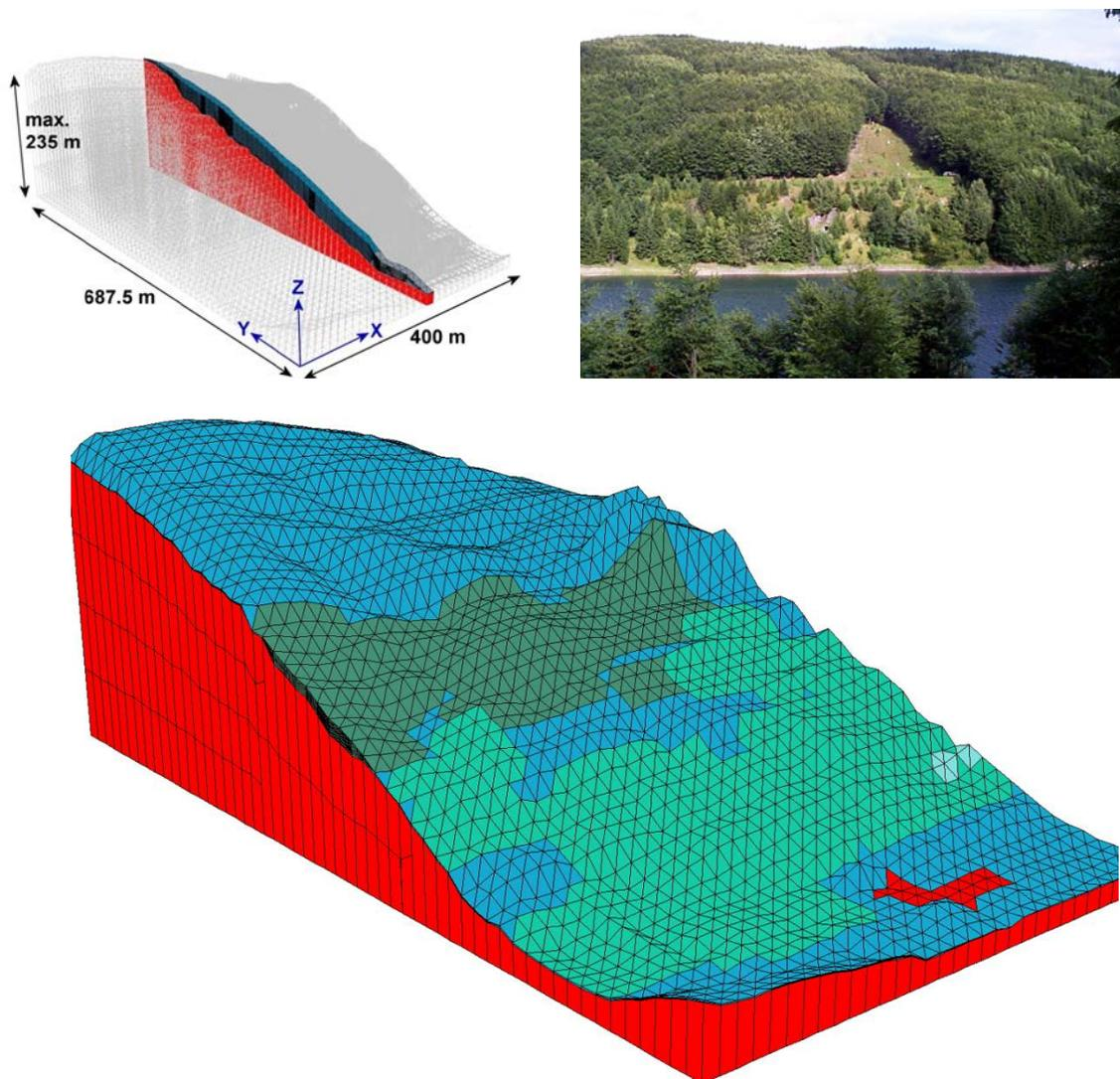
Fig. 6.1: Photo and numerical model of creeping reservoir slope (Konietzky 2004a,b et al. & TFV, 2007)
