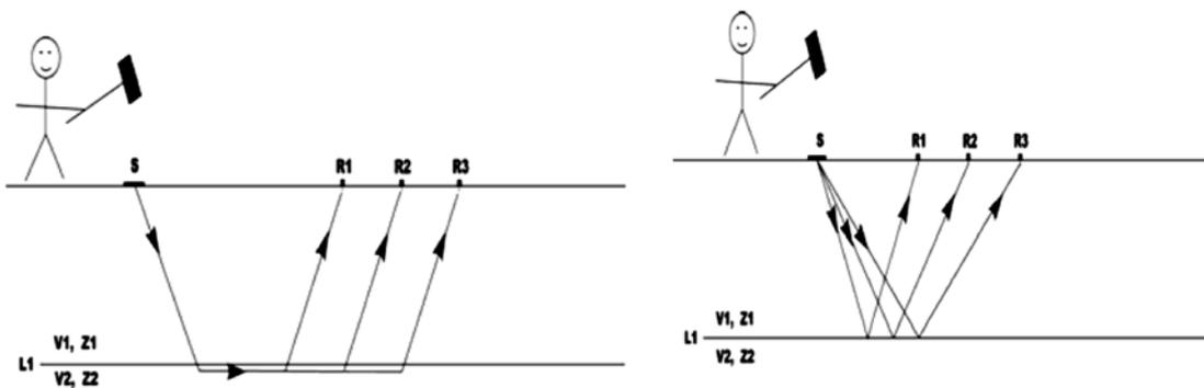
Fig. 3.1.1: Seismic refraction (left) and reflection (right) method
