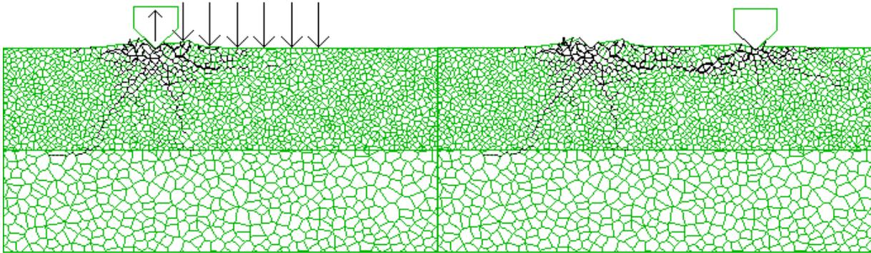
Fig. 27: Simulation of rock fragmentation due to penetration of a single disk cutter (Lunow & Konietzky 2010)
