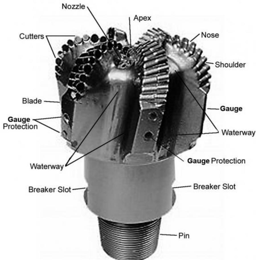
Fig. 14. Principle design of PDC drill bits (company material)
