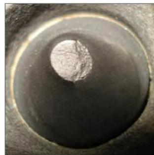
**WT** – Minor wear (Level 2 severity)
