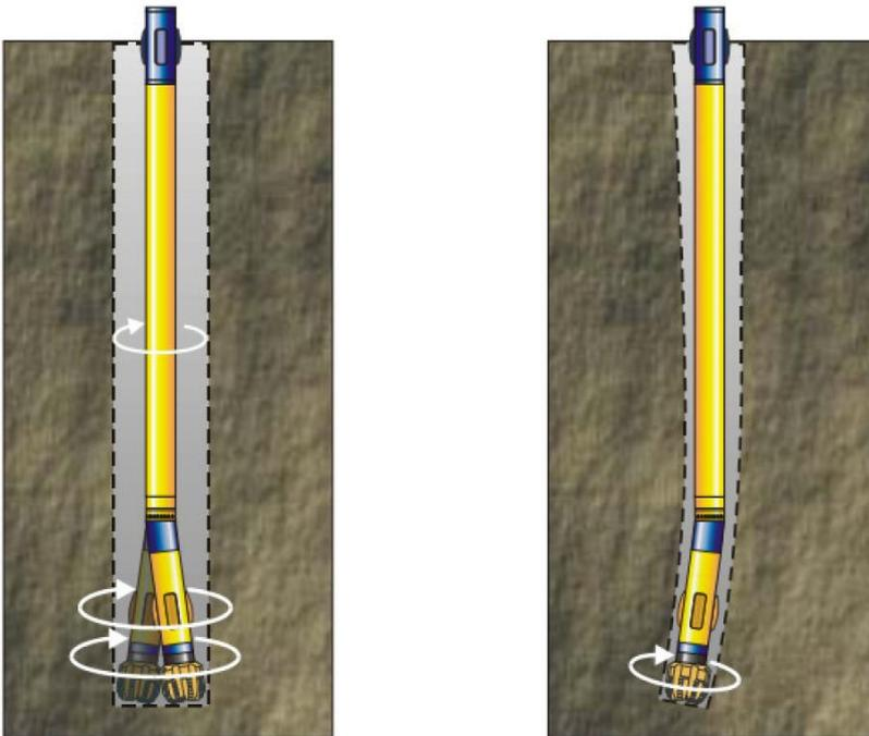
Fig. 2. Principle of rotary steerable systems (company material)
