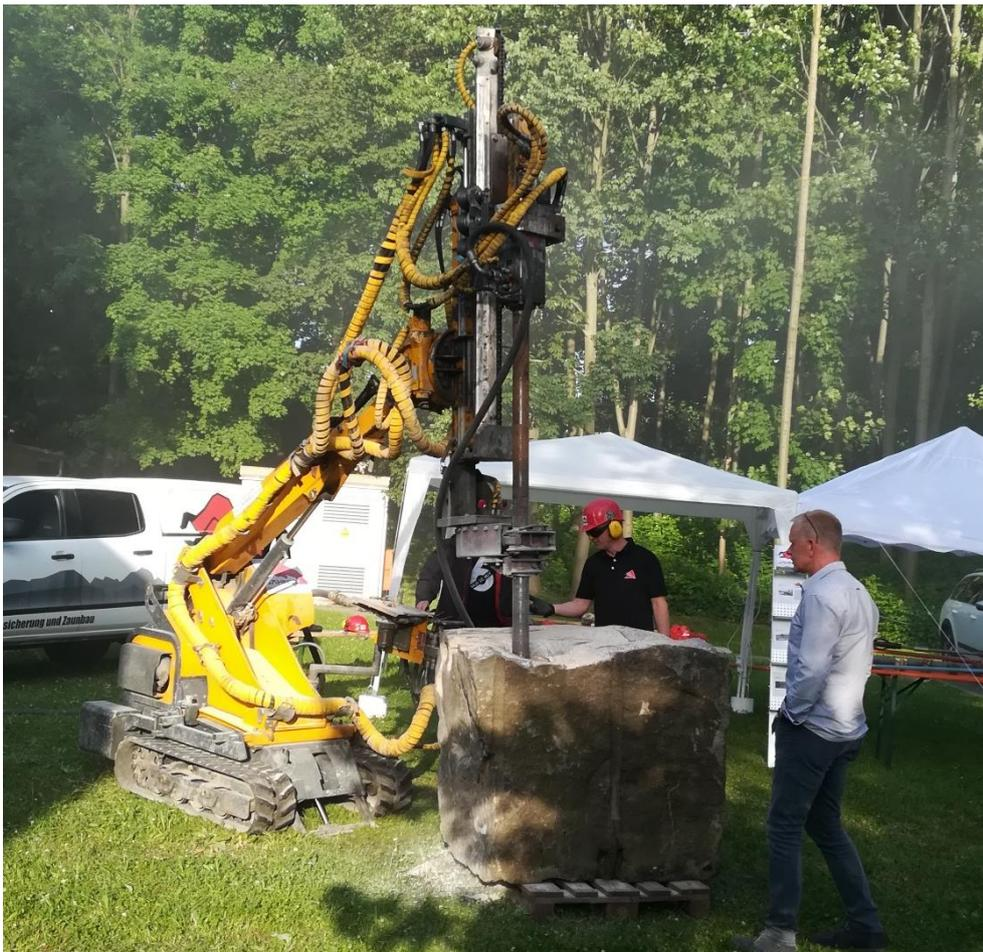
Fig. 17: Portable drill rigs for small scale holes
