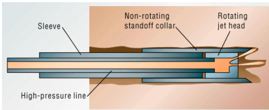
Fig. 6: Water jet drilling (company material)
