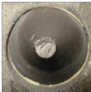
**WT** – Minimal wear (Level 1 severity)
