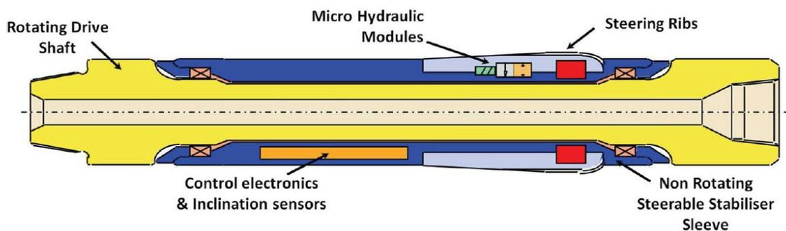
Fig. 4: Sketch of steering mechanism (company material)
