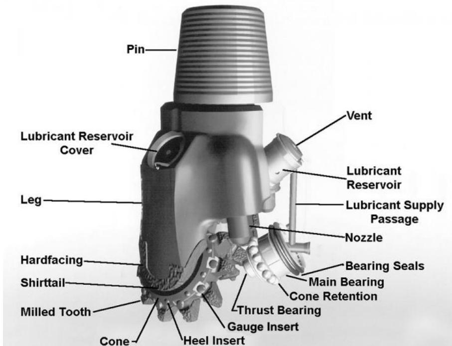
Fig. 13. Principle design of roller cone bits (company material)
