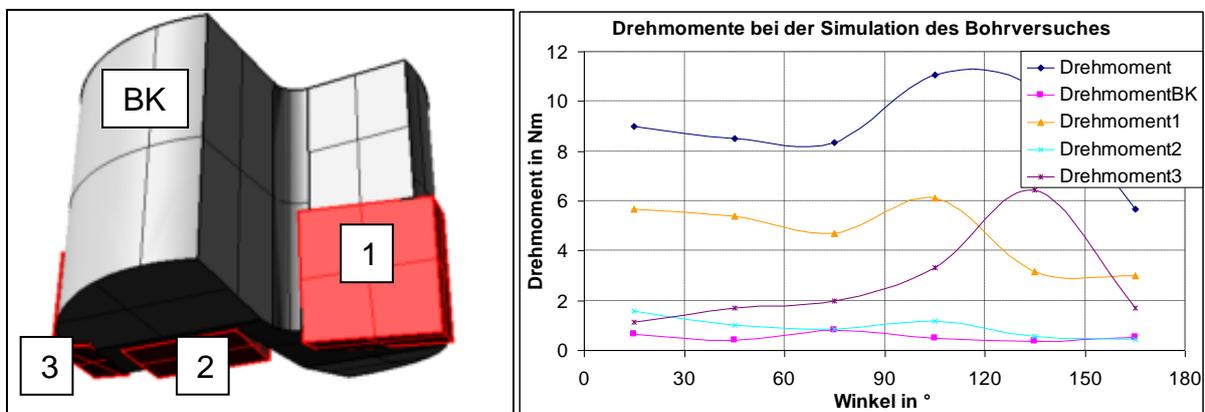
Fig. 29: Drilling head with three inserts and simulated moments acting on these parts (Lunow 2015)
