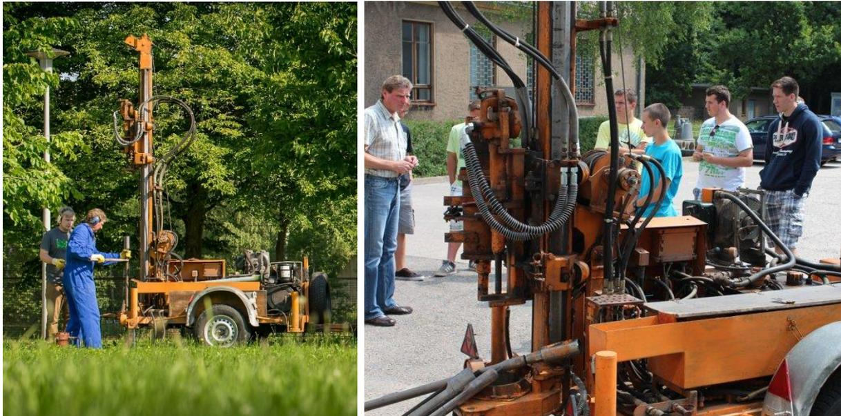
Fig. 19: Mobile trailer drill rig (RML 2016)
