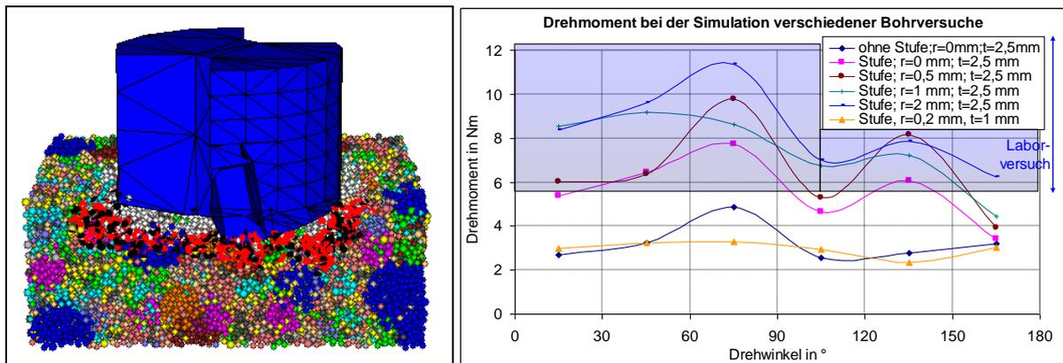
Fig. 28: Simulation of drilling process and comparison with moments measured in the lab (Lunow 2015)
