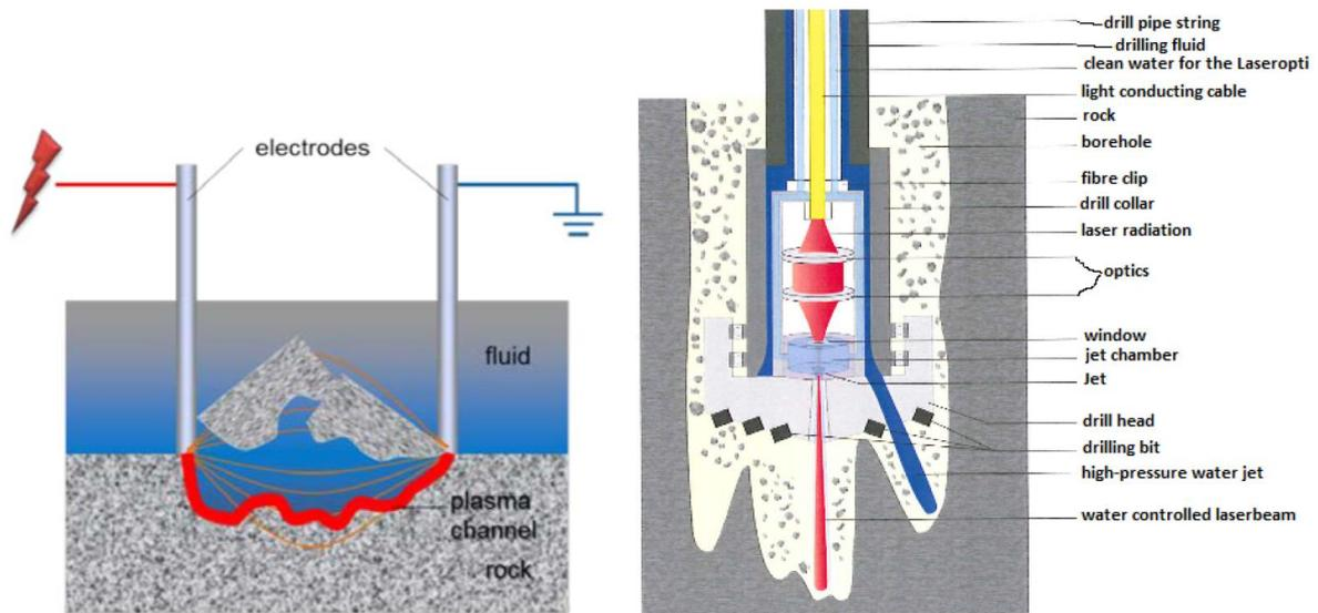
Fig. 30: Scheme of EIT (left) and laser drilling (right) (Richter, 2017)
