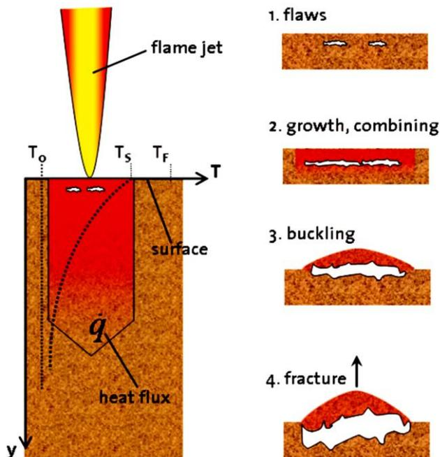
Fig. 8. Principal of hydrothermal spalling drilling (www.transfer.ETH.ch)
