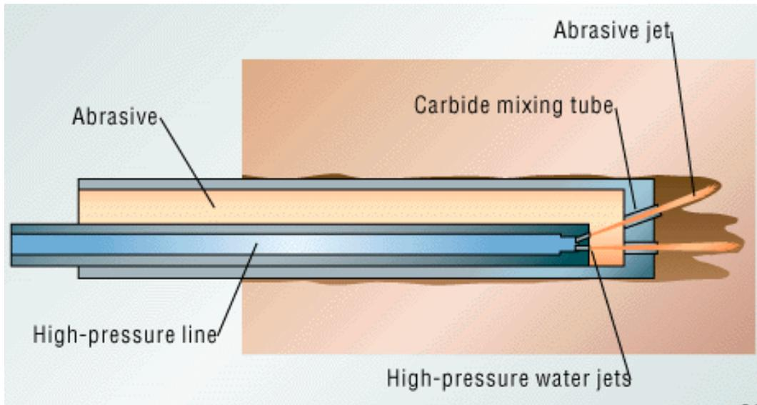
Fig. 7: Abrasive water jet drilling (company material)
