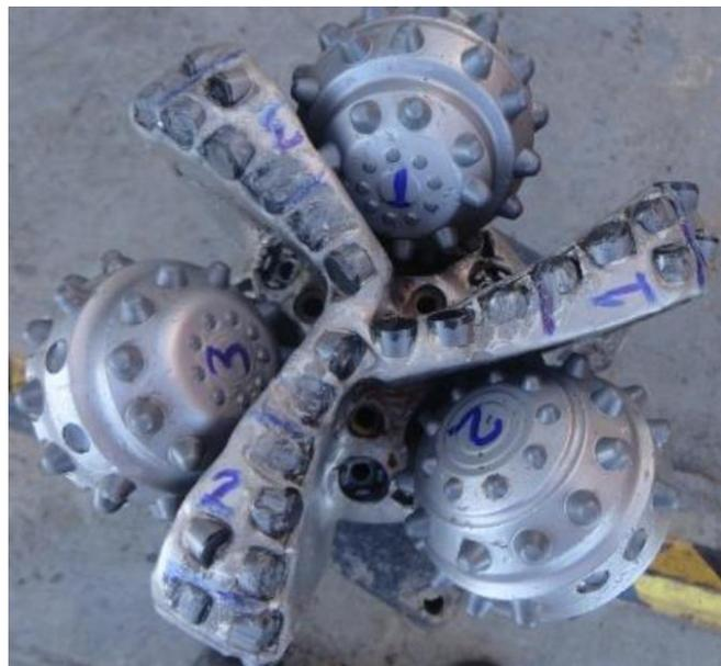
Fig. 11: Hybrid drill bit with PDC cutters for large holes and deep drilling (company material)
