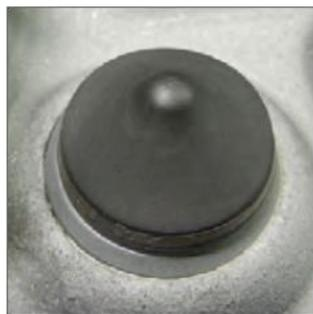
**WT** – No wear (Level 0 severity)
