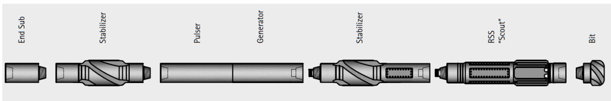
Fig. 3. Principle set-up of RSS (company material)
