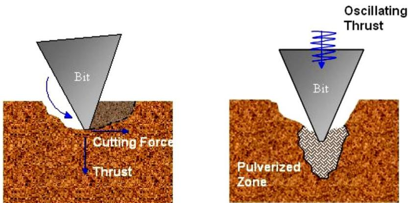
Fig. 26: Principal of rock fragmentation in rotary (left) and percussion (right) drilling (Terralog 2005)
