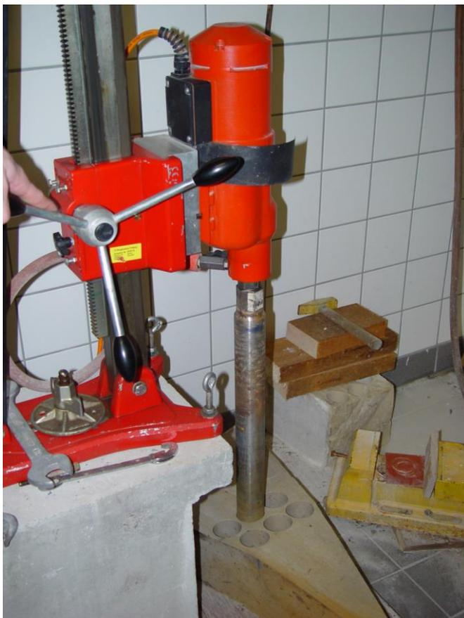
Fig. 24: Lab drill rig to extract cores from rock blocks (RML 2017)
