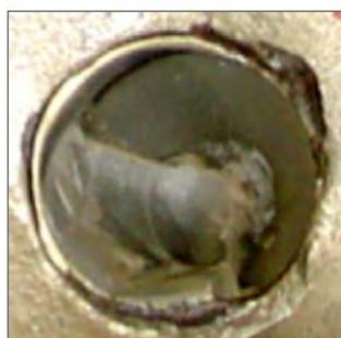
**DL** – Stinger element delamination
