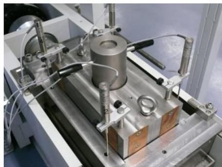
f) LVDTs for displacement measurement
