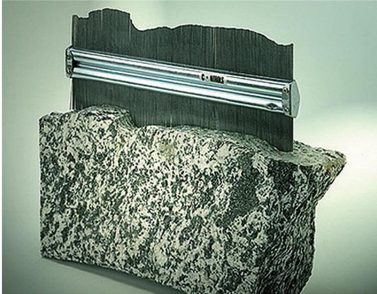
Fig. 4. Classical profilometer for measuring the roughness profile of rock samples [ControlsGroup 2013]
