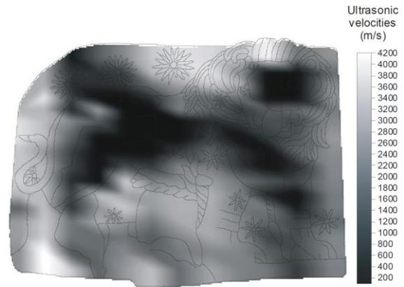
Fig. 5: Ultrasonic P-wave speed measurements (Fitzner, 2004b)
