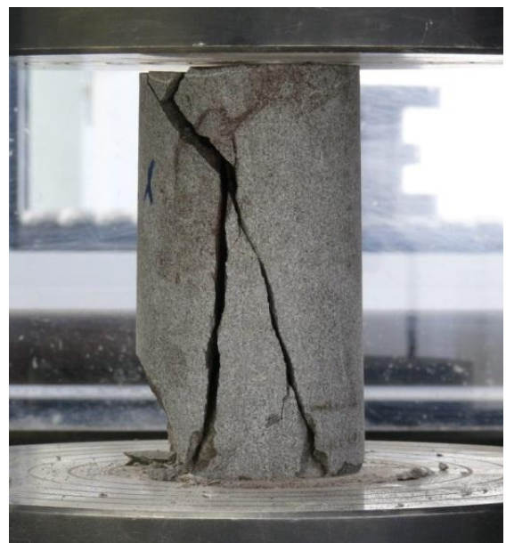
Fig. 3.7.4: Typical fracture pattern: axial splitting (left) and shear fracturing (right) [RML 2016]
