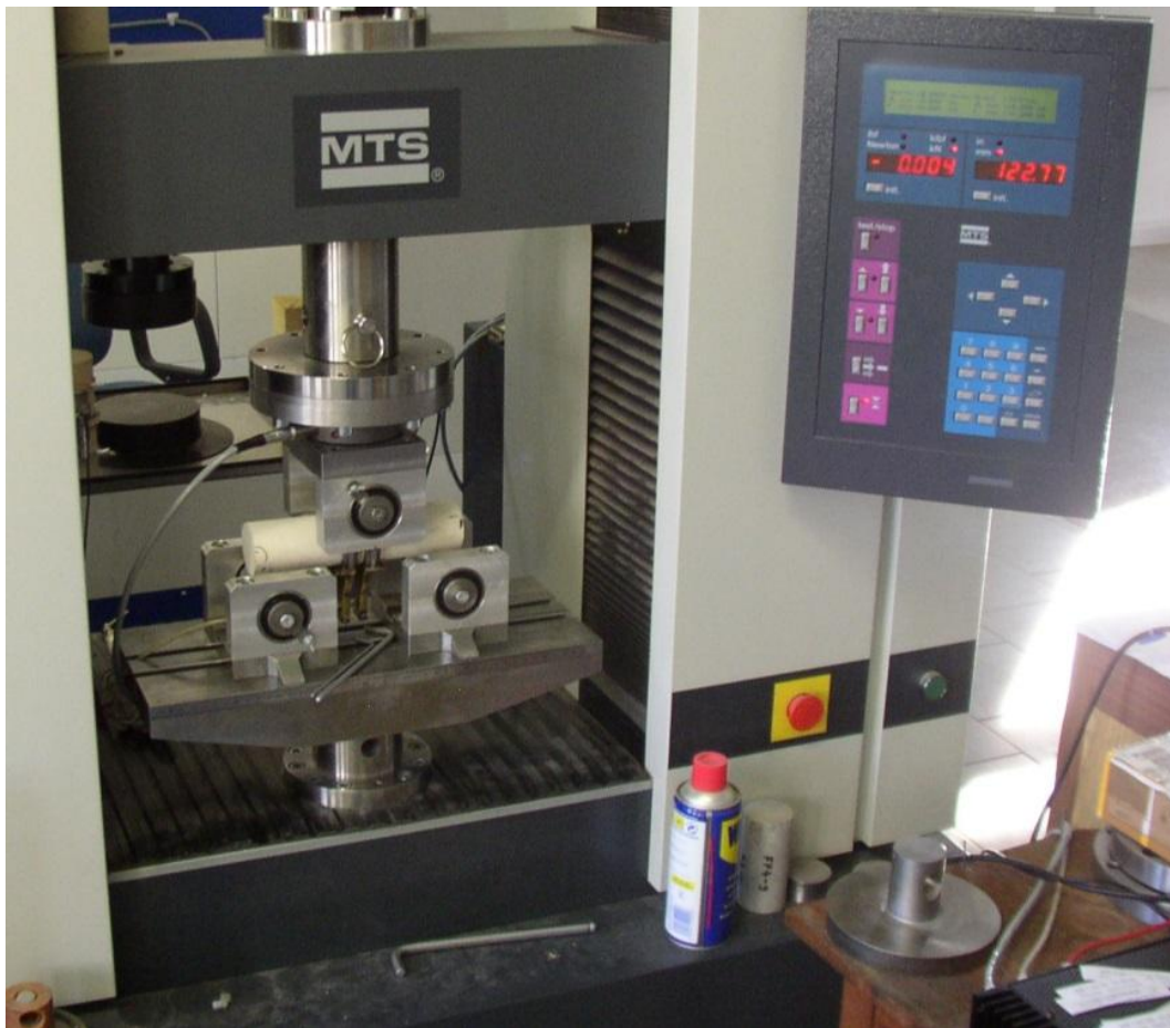
Fig. 3.15.1: Test set-up for CBS test [RML 2016]
