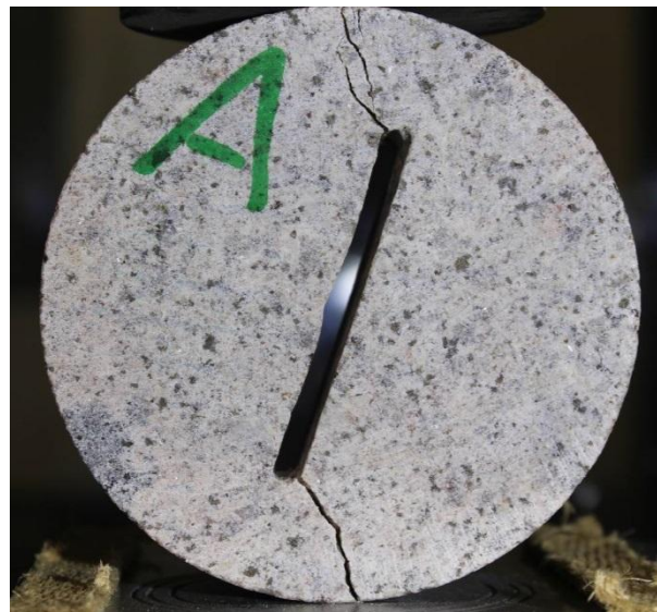
Fig. 3.15.3: Test set-up for CCNBD test [RML 2016]
