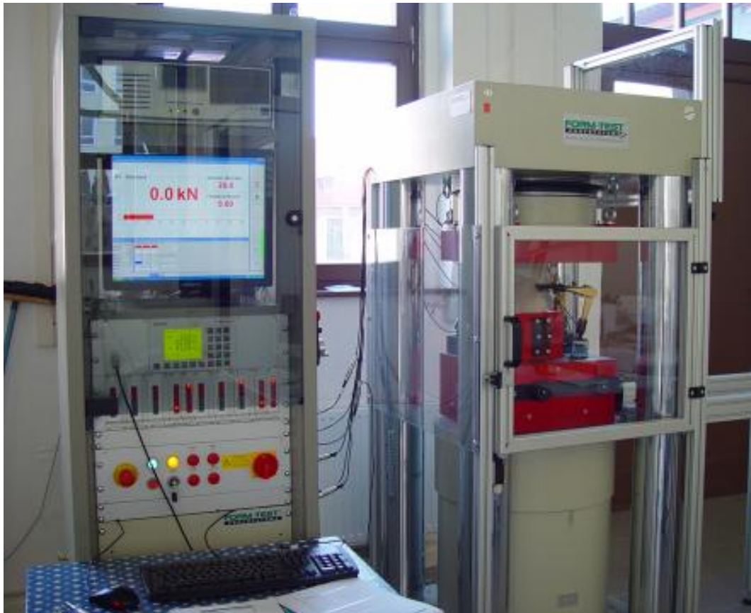
Fig. 3.7.1: Typical machine for uniaxial compression tests [RML 2016]
