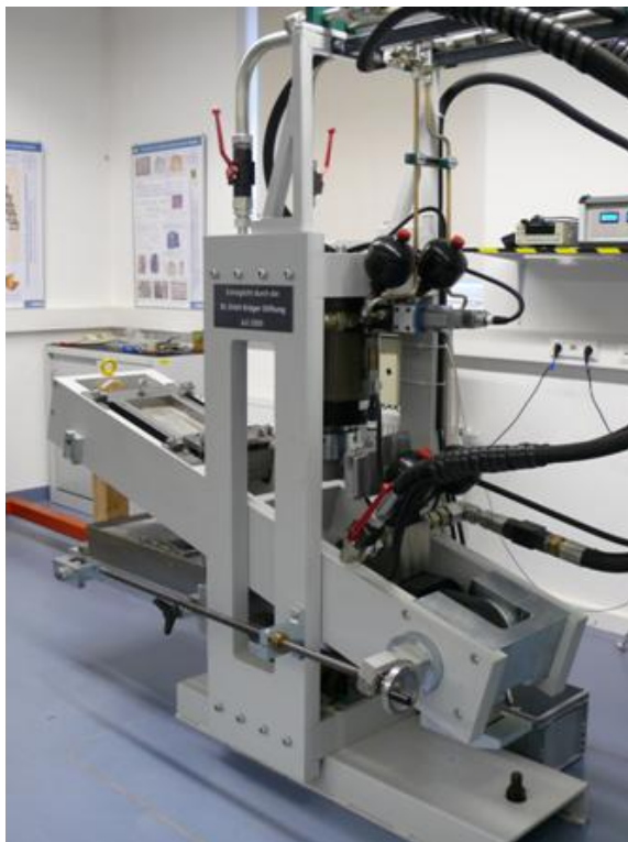
Fig. 3.14.2: Foto of a shear box device and view into empty shear boxes [Konietzky et al. 2012]
