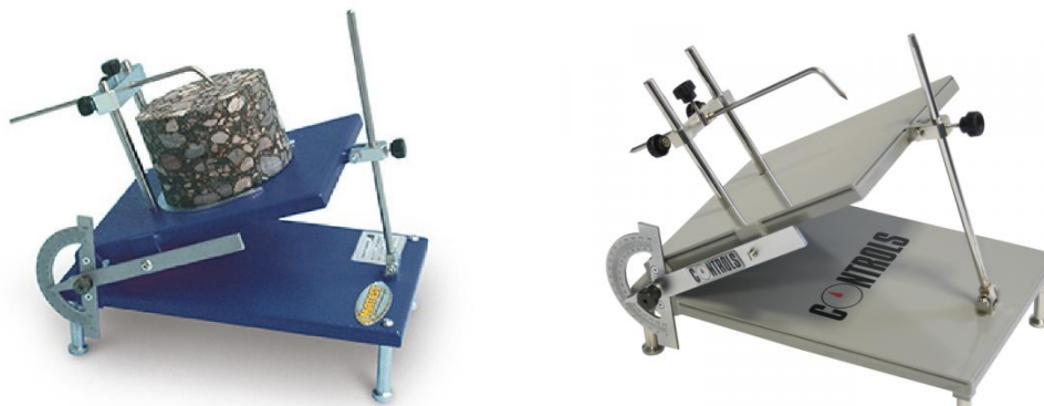
Fig. 3.11.2: Tilt test equipment (company material)
