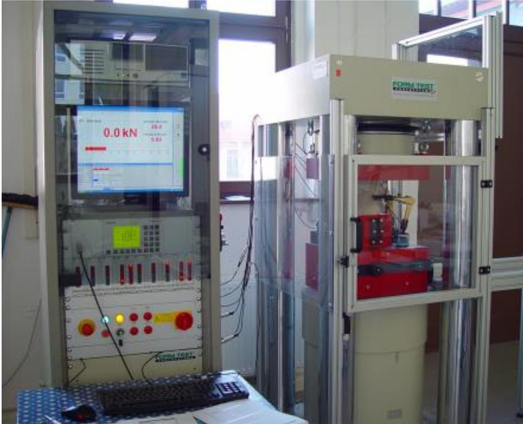
Fig. 3.7.1: Typical machine for uniaxial compression tests [RML 2016]
