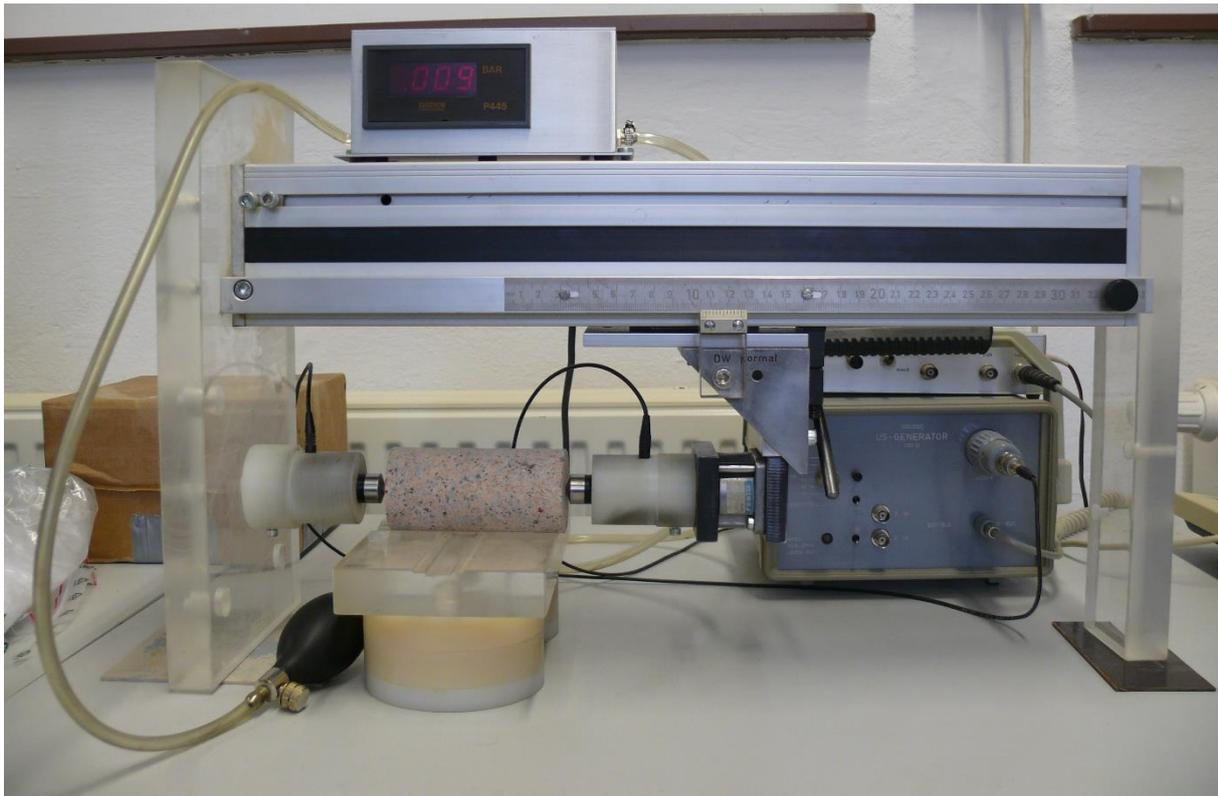
Fig. 3.6.1: Typical equipment to measure sound velocity on core samples [RML 2016]
