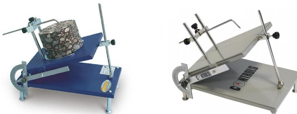
Fig. 3.11.2: Tilt test equipment (company material)
