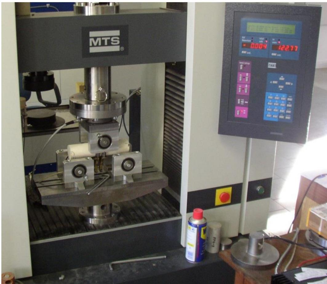
Fig. 3.15.1: Test set-up for CBS test [RML 2016]
