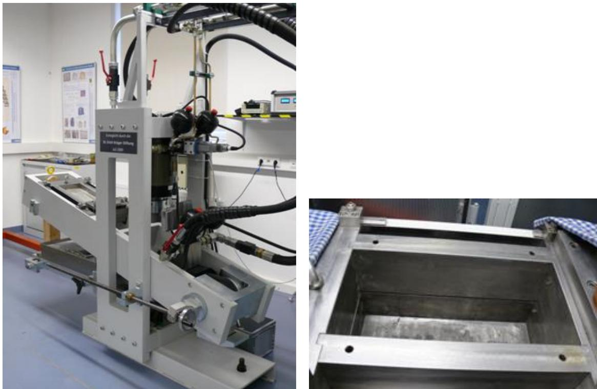
Fig. 3.14.2: Foto of a shear box device and view into empty shear boxes [Konietzky et al. 2012]
