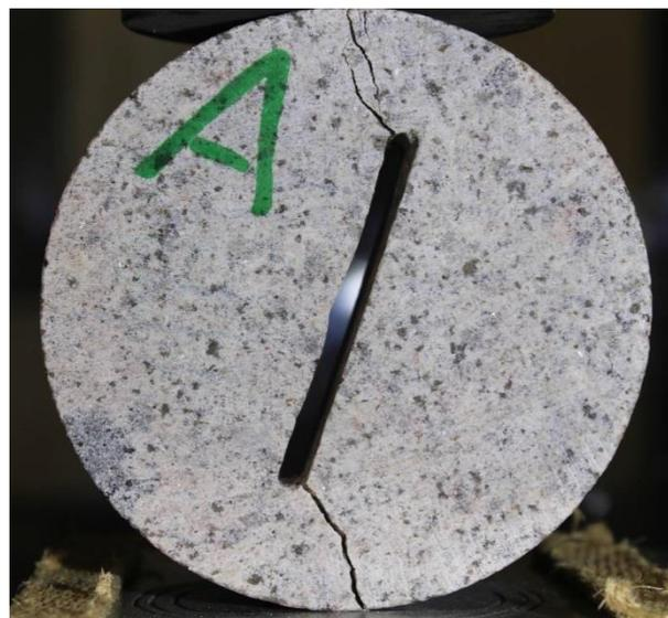
Fig. 3.15.3: Test set-up for CCNBD test [RML 2016]
