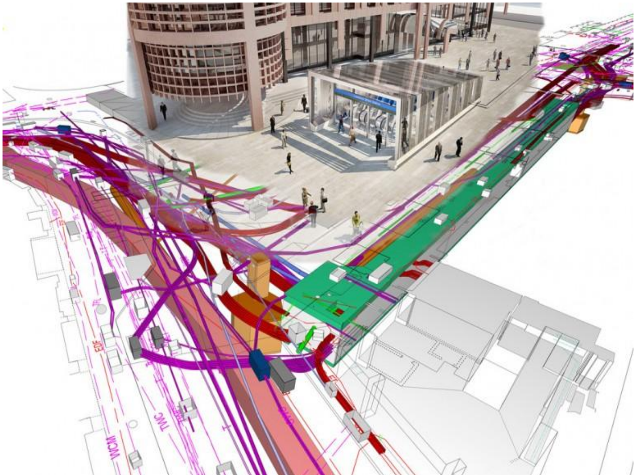
Fig. 5.2.6: BIM based presentation of existing underground infrastructure at a crossing in London (Cross-rail in DAUB, 2019)
