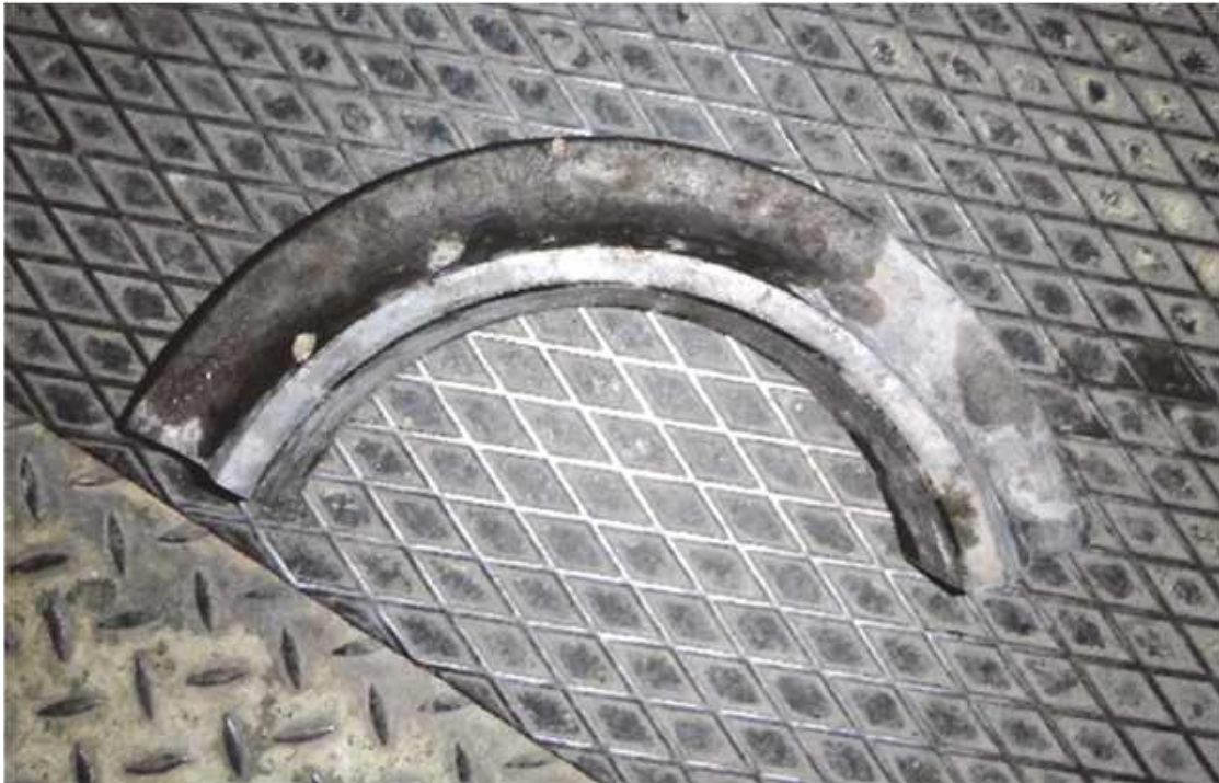
Fig. 4.2: Broken 17"-cutter disc of a hardrock TBM (Photo: Plinninger).
