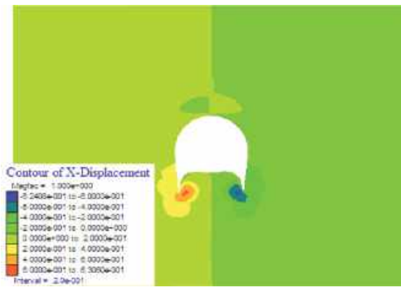
(a) Horizontal convergence of original support
