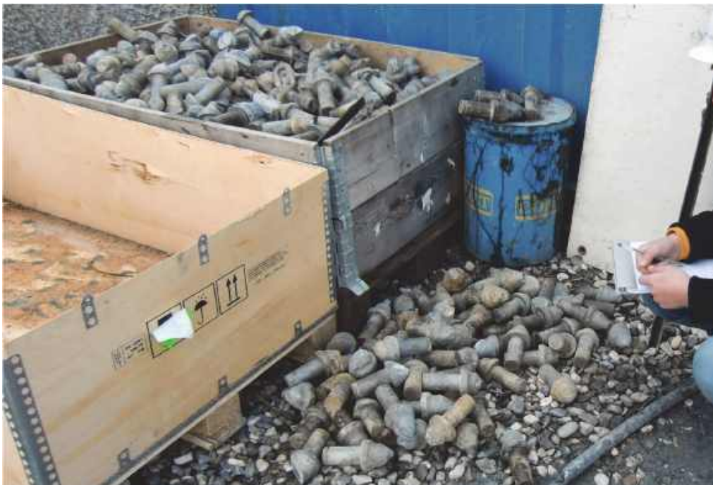
Fig. 2.1: Worn point attack picks of a roadheader, whose replacement was both caused by continuous abrasion, as well as partial failure of tool components (Photo: Plinninger).
