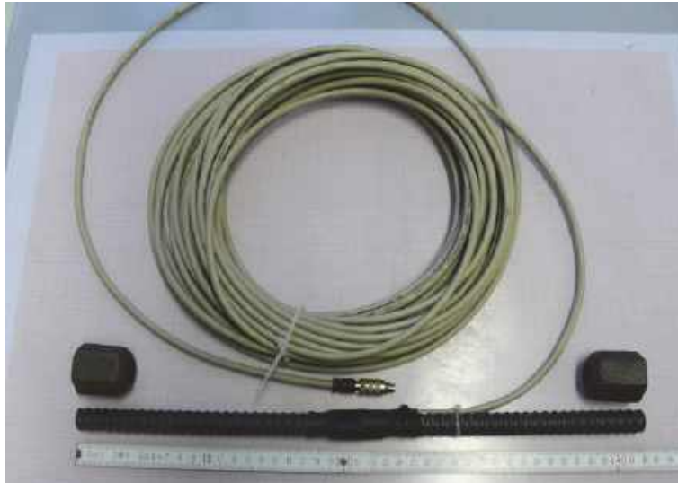
Fig. 3.1: Prototype of gauged rock bolt rod equipped with encapsulated strain gauges and 30 m electrical cable.
