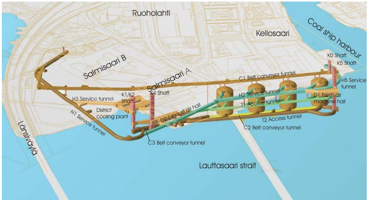
Fig. 7.4: Underground coal storage (Rockplan, 2020)
