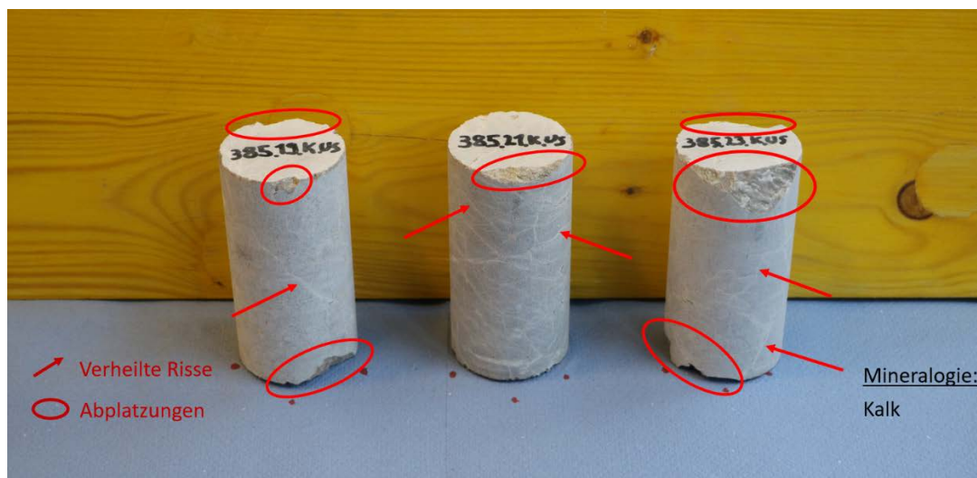
Fig. 5: Limestone samples in their original state: Spalling caused by processing the samples during cutting with a circular saw and/or grinding is circled in red in the image. Some of the healed cracks are marked with red arrows.
