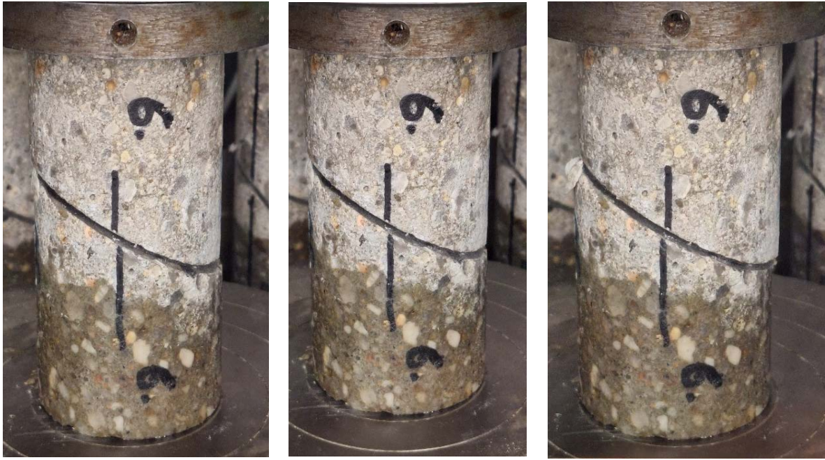
Fig. 11: Pictures made during the creep test of T-2_30-6 for temperature T = -1^{\circ}\text{C} . The ice-layer is clear, no fracturing occurred.
