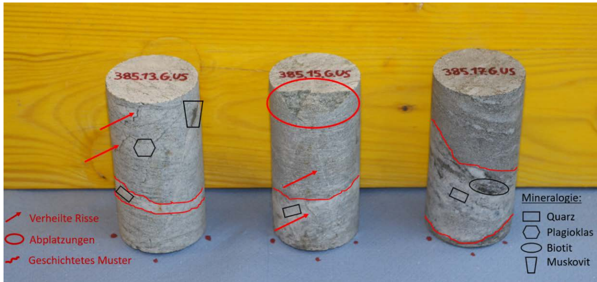
Fig. 6: Gneiss in its original state: Spalling caused by processing the samples during cutting with a circular saw and/or grinding is circled in red in the image. Some of the healed cracks are marked with red arrows. The red lines represent foliations.
