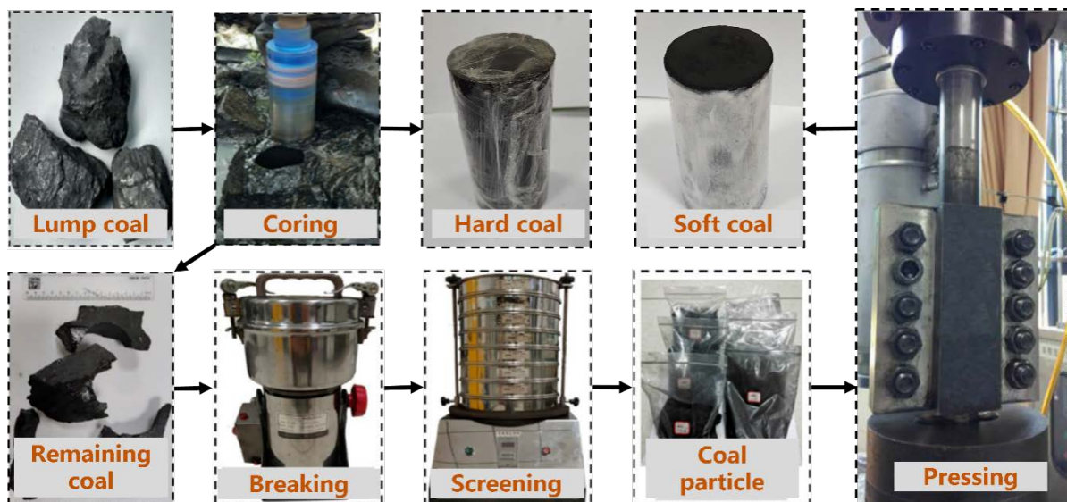
Fig. 8: Preparation process of regularly shaped coal columns.
