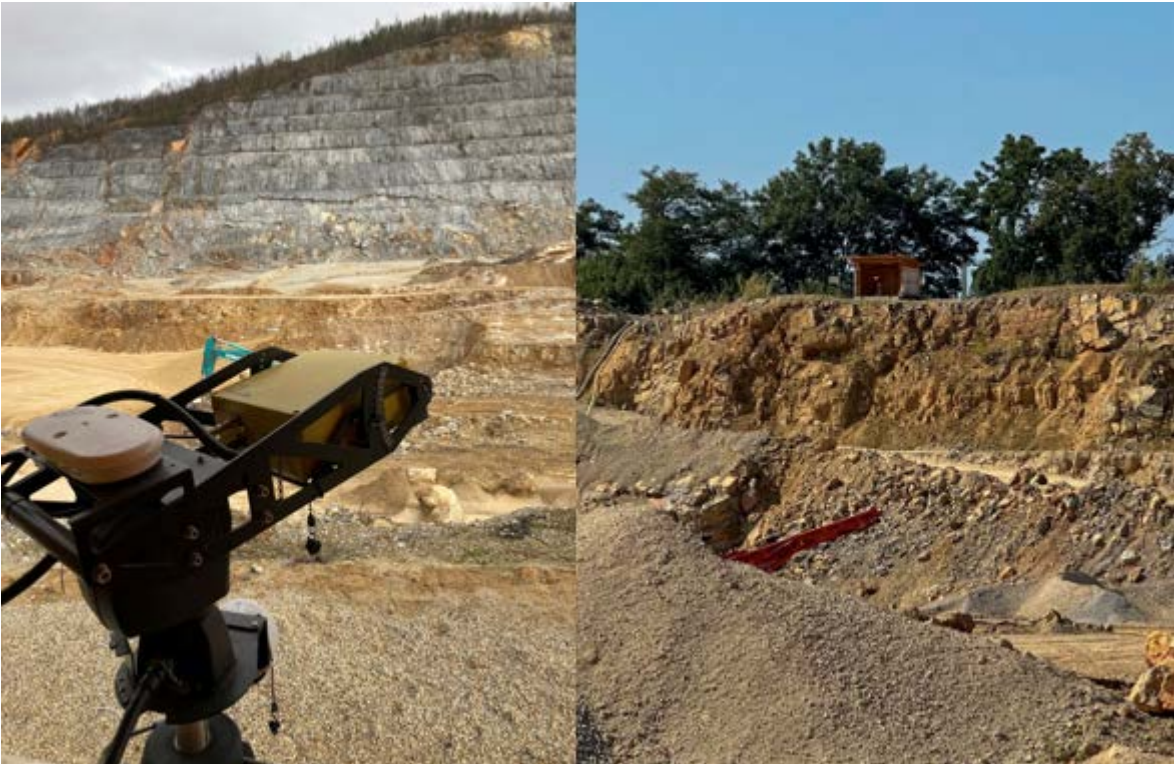
Fig. 23: Position of IDS Georadar HYDRA – X on Quarry.
