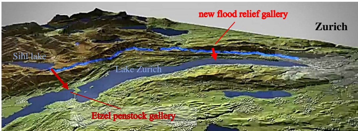
Fig. 2: Model view of Lake Zurich with the Sihl river, the penstock gallery of the existing Etzel hydropower station, and the new free-flow gallery at Thalwil [1].
