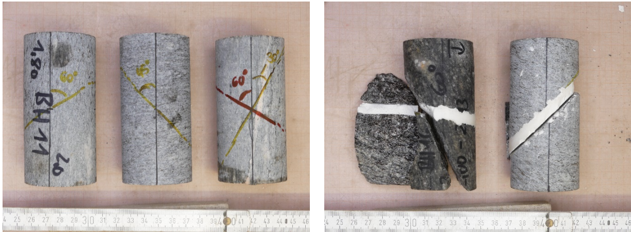
Fig. 26: Gneiss samples with distinct discontinuities before preparation and after testing.
