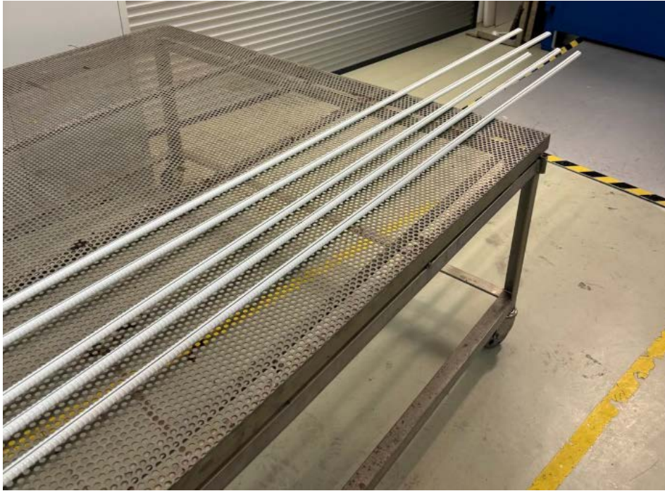
Fig. 17: Intelligent rock bolts prepared for the curing process.
