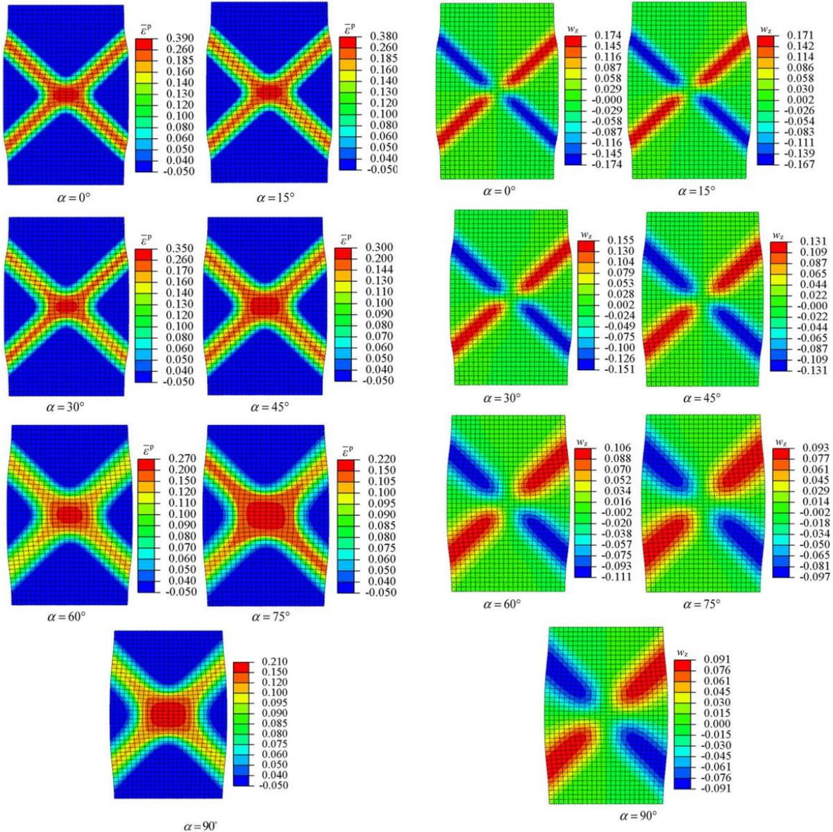
Fig. 10.4: Plastic strain (left) and rotations (right, in radians) for a biaxially loaded sample (transverse isotropic MC model) with different angle of weak plane  $\alpha$  in the post-failure region at 6% vertical strain (Wei et al. 2025).
