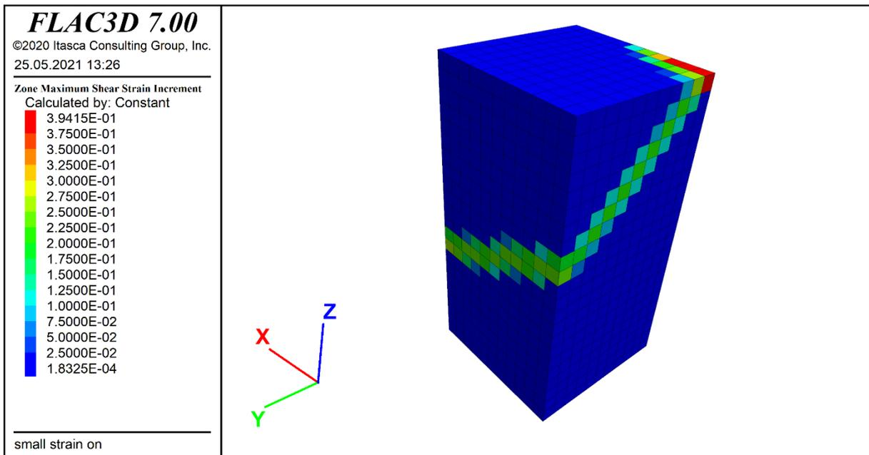
Fig. 12.4: UCS test: Accumulated shear strain for **large strain modulus** (above) and **small strain modulus** (below) for identical vertical displacement at sample top and sample bottom of  $9e-3$  m
