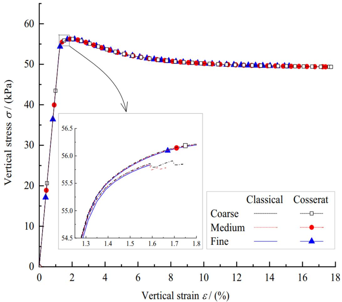
Fig. 10.5: Stress-strain curve for model with inclination angle of weak plane of 45° (Wei et al. 2025). The edge length of the meshes are as follows: coarse mesh: 3.5 mm, medium mesh: 2.5 mm, fine mesh: 1 mm.
