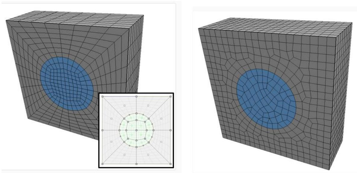
Fig. 4.5: Workflow from 3D CAD surface model to 3D volume mesh (Itasca, 2021)
