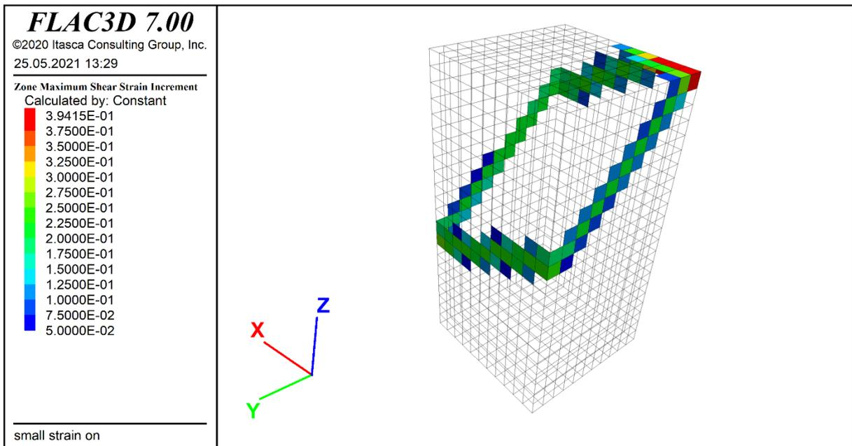
Fig. 12.5: UCS test: indication of shear plane (strain localization) by accumulated shear strain for **large strain modulus** (above) and **small strain modulus** (below) for identical vertical displacement at sample top and sample bottom of  $9e-3$  m
