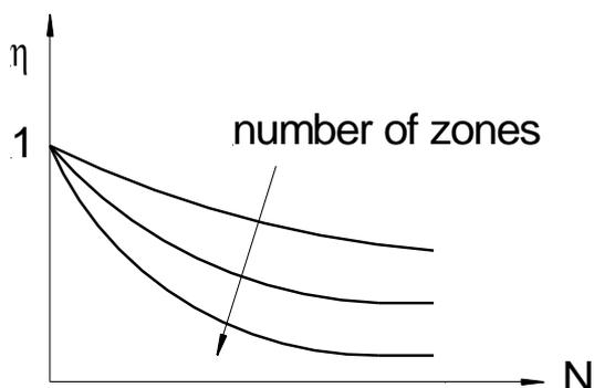
Fig. 11.2: Calculation efficiency  $\eta$  as function of number of processors  $N$  and number of zones
