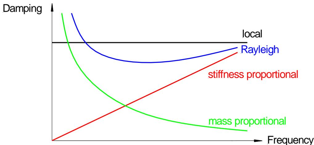
Fig. 8.1: Damping vs. frequency for different damping procedure
