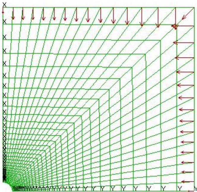
Fig. 10.2: Mesh for 1/4-symmetric tunnel including boundary conditions (900 zones)
