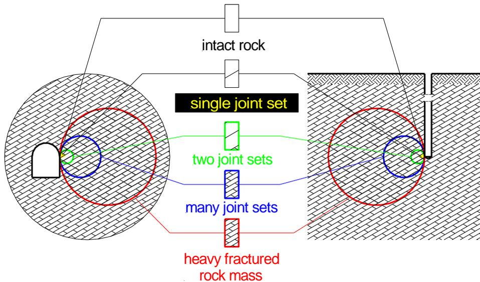
Fig. 7.2: Relation between structure and considered volume using the example of a rock mass (scale effect).
