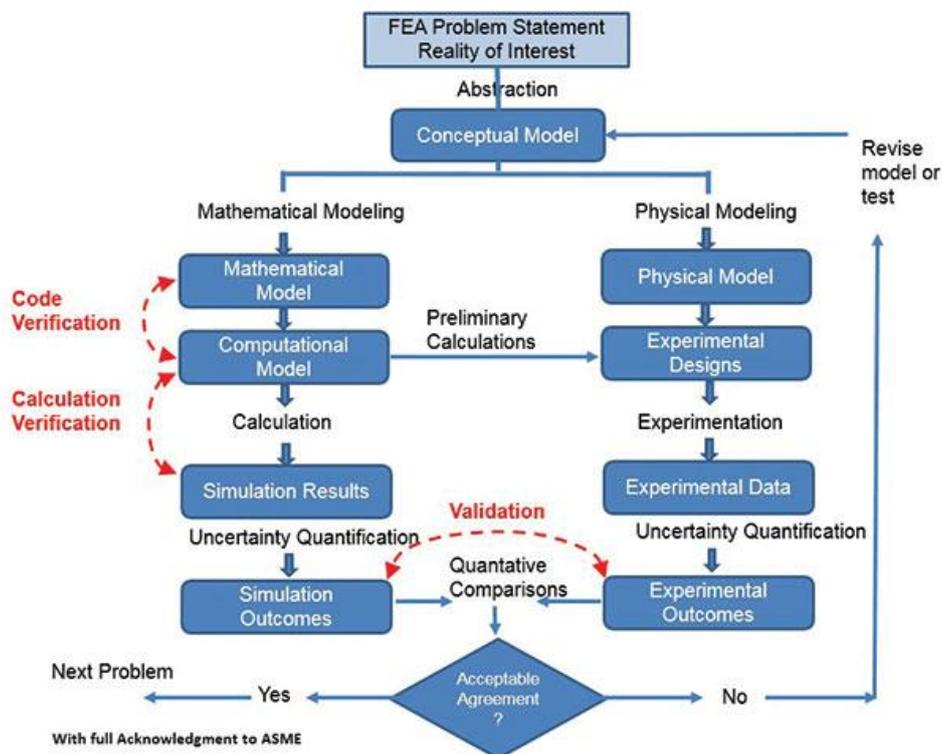
Fig. 15.2: Illustration of verification and validation (ASTM)
