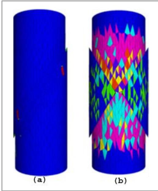
Fig. 10: Images of failed specimens for the (a) single-joint model, and (b) double-joint model of Chong et al. (2013) (the non-blue colour areas denote shear/tensile failure within intact material)
