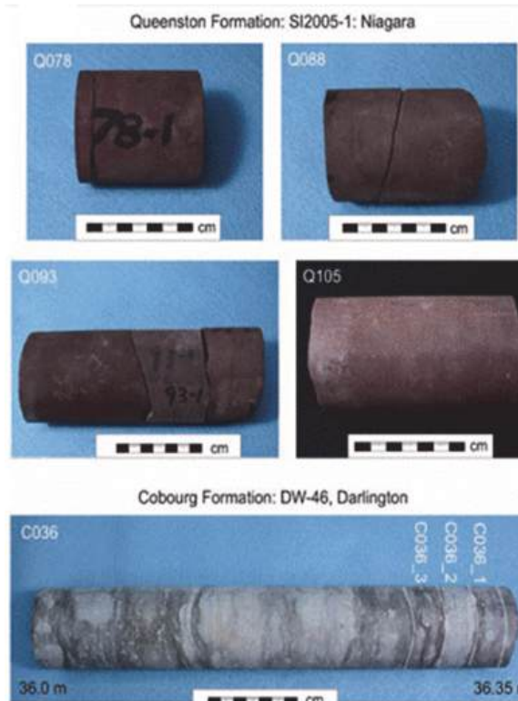
Fig. 7 Drilled core samples from Queenstone Shale and Cobourg Formations (Vilks and Miller, 2007)
