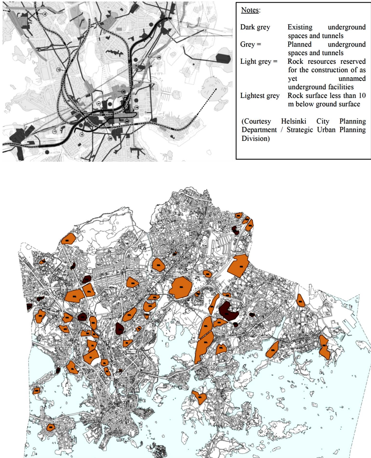
Fig. 1.2: Existing and planned usage of underground space in the city centre of Helsinki (top) and planned used for underground constructions according to the master plan 2010 (bottom) for Helsinki (Vähäaho, 2011).
