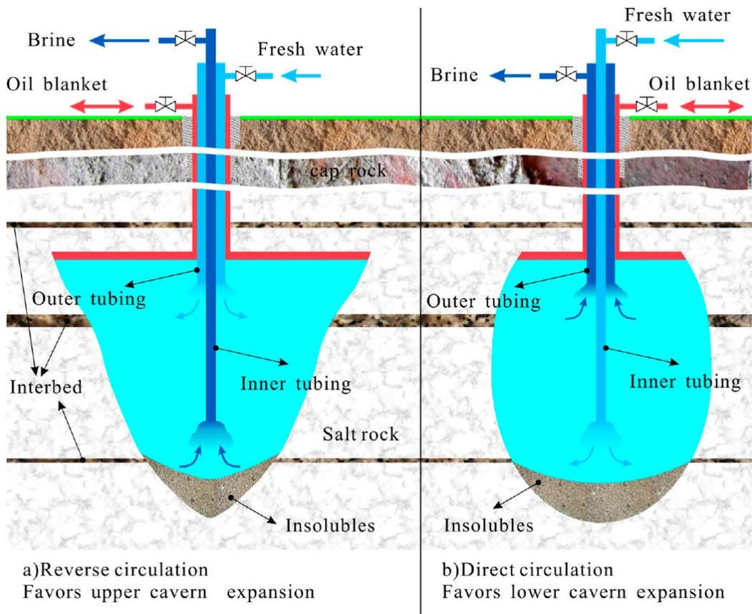
Fig. 2.8: Principles of direct and reverse circulation to create salt caverns (Ge et al., 2019)
