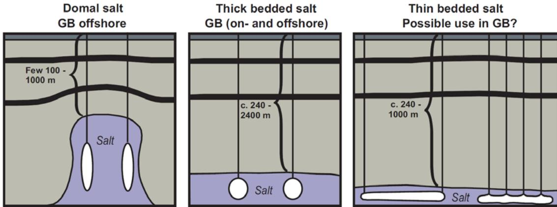
Fig. 2.2: Salt caverns in different types of salt deposits (BGS, 2008)
