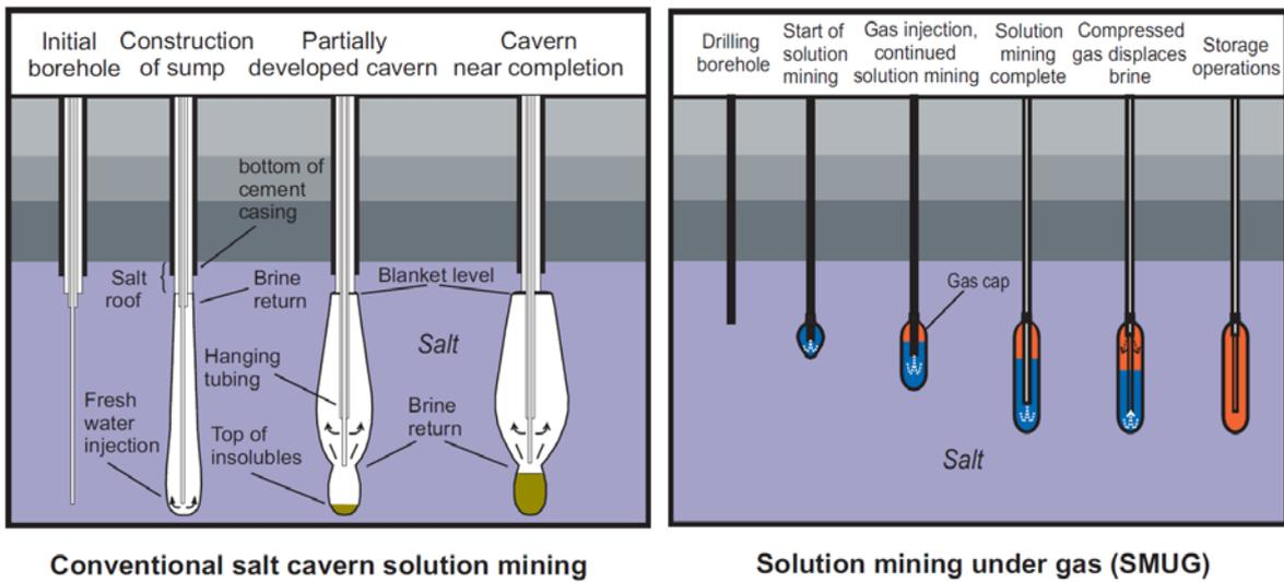
Fig. 2.6: Conventional versus SMUG solution process (BGS, 2008)
