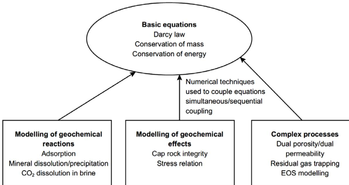
Fig. 3.4: Workflow of CO<sub>2</sub> modeling (Ajayl et al., 2019)
