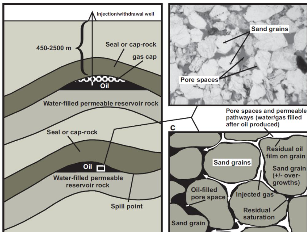
Fig. 3.1: Concept of pore storage (BGS, 2008)
