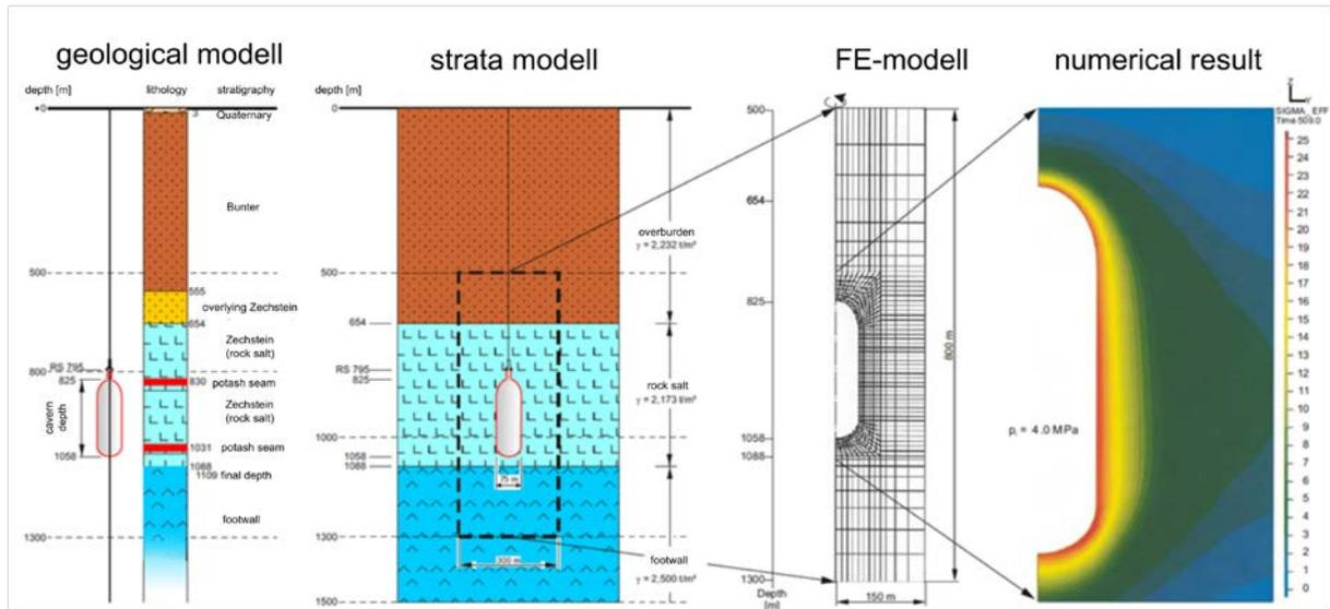
Fig. 2.10: Procedure for rockmechanical cavern dimensioning (Modified after KBB et al., 2007)
