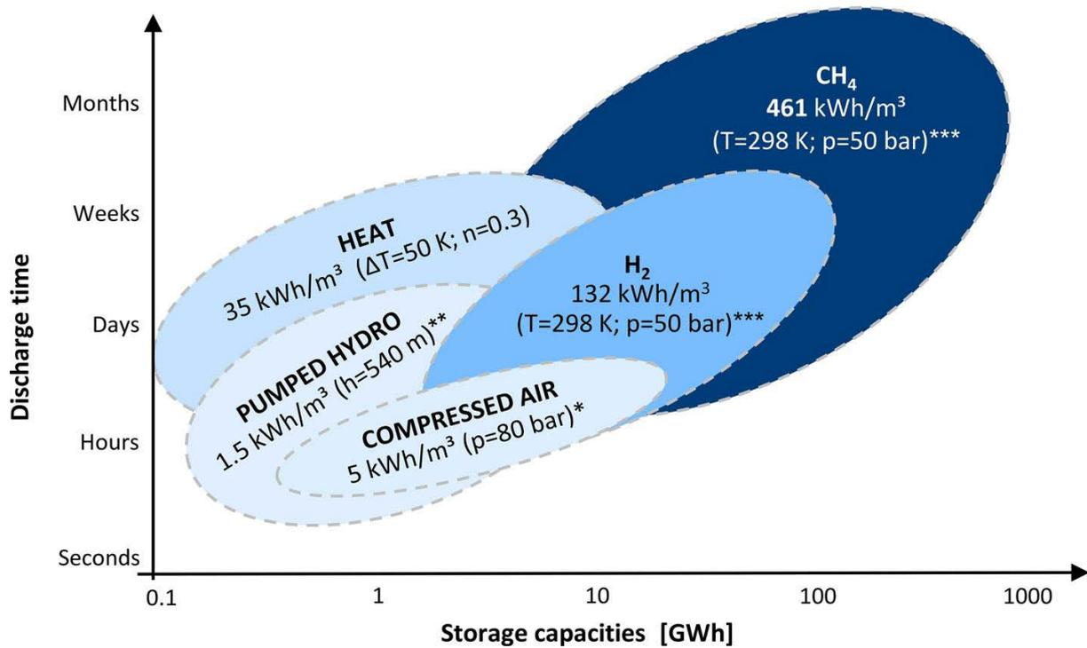
Fig. 1.3: Storage capacity and discharge time of different storage media (Kabuth et al., 2017)
