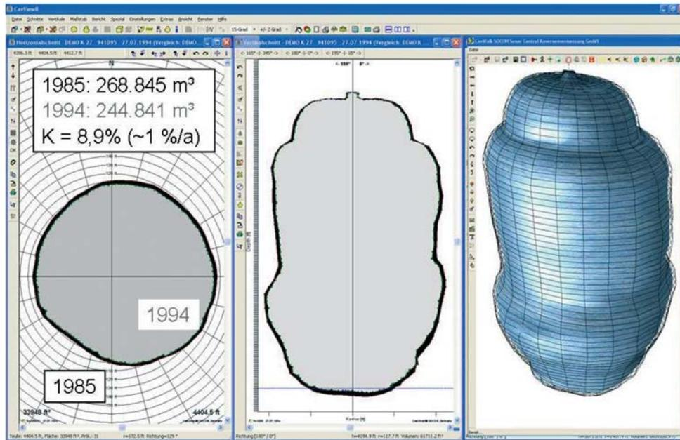
**Fig. 2.14:** Results of sonar measurement of a salt cavern (Reitze et al., 2010)
