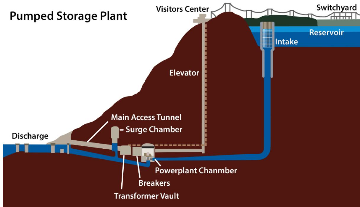
Fig. 4.1: Classical hydroelectric pumped-storage system (REA, 2016)
