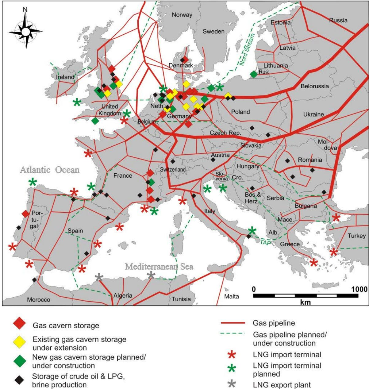
Fig. 2.5: Gas cavern storage system, pipelines and LNG import terminals in Europe (Gillhaus, 2007)
