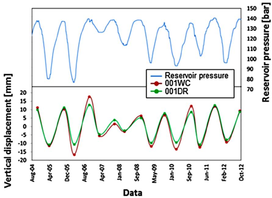
Fig. 5.3: Average reservoir pressure and vertical movement of two measurement points above the storage area (Codegone et al., 2016)
