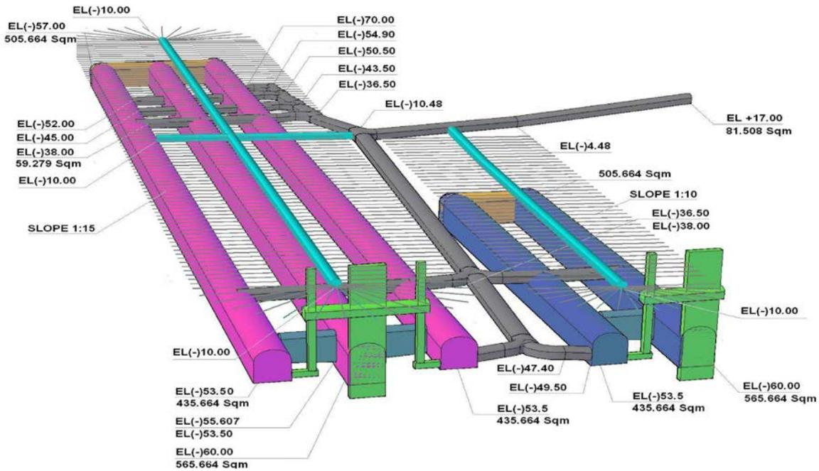
Fig. 2.15: Unlined cavern system in hardrock in India with water curtain boreholes (Höfer-Öllinger et al., 2014)
