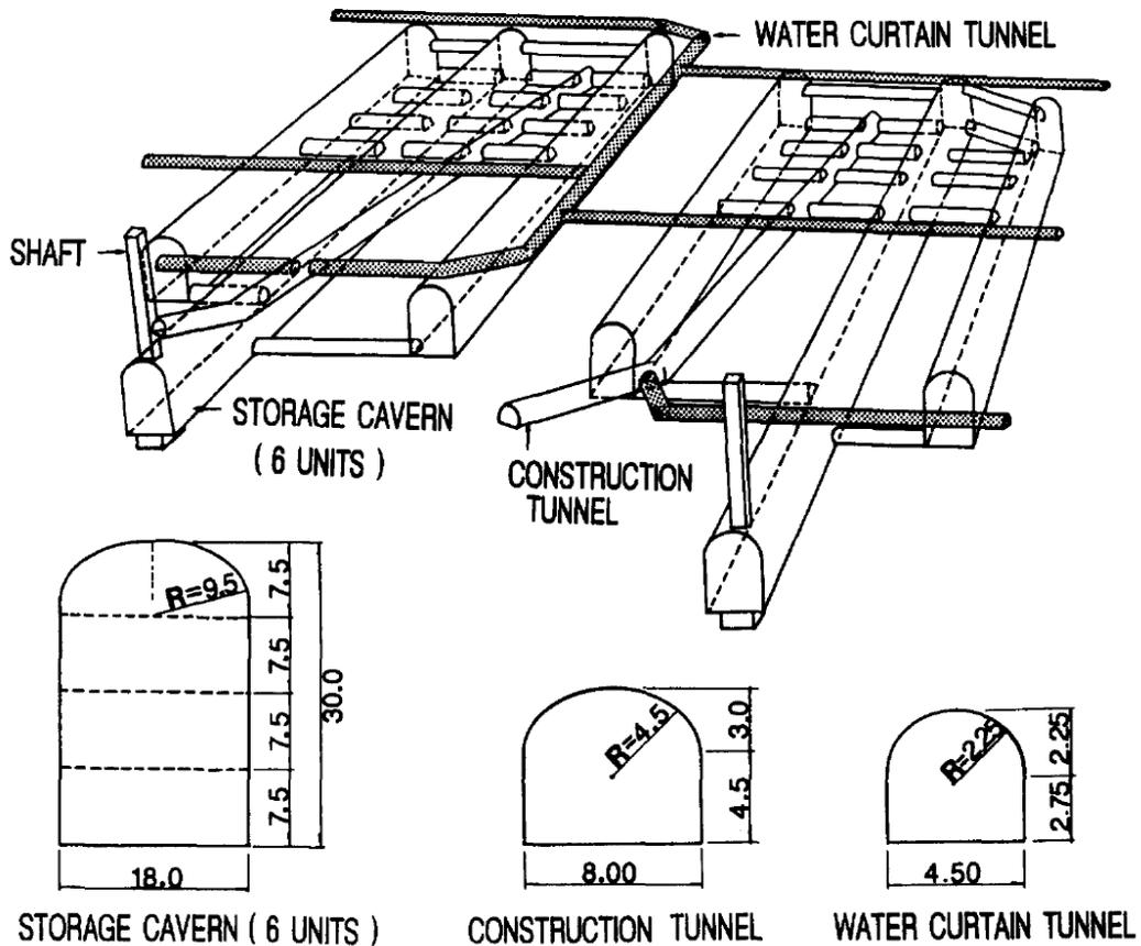
Fig. 2.16: Unlined cavern system in hard rock in South Korea with water curtain tunnels (Lee et al., 1996)
