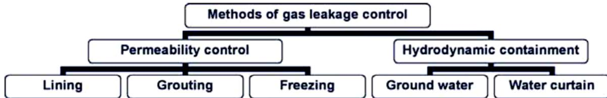
Fig. 2.17: Methods to control gas leakage from pressurised underground storage facilities (Grøv, 2007)
