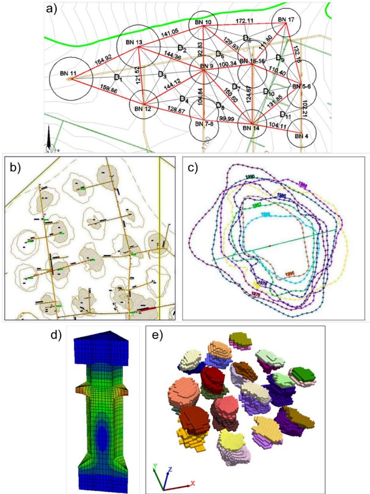
Fig. 2.13: Numerical simulation of a cavern field. a) idealized sketch of cavern field; b) real cavern field; c) contour of one single cavern for several depth values; d) numerical model for single pillar in idealized cavern field; e) complex 3D model for cavern field with realistic geometries (Modified after Huber et al., 2012)
