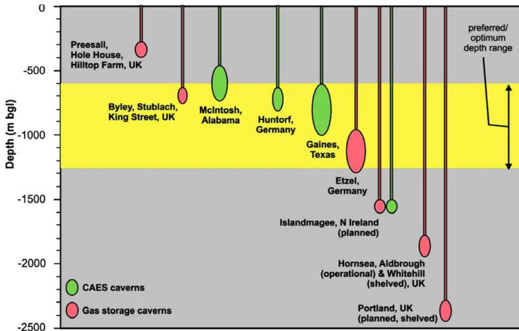
Fig. 2.3: Depth of operational and planned CAES and gas storage cavern (Kepplinger et al., 2011)
