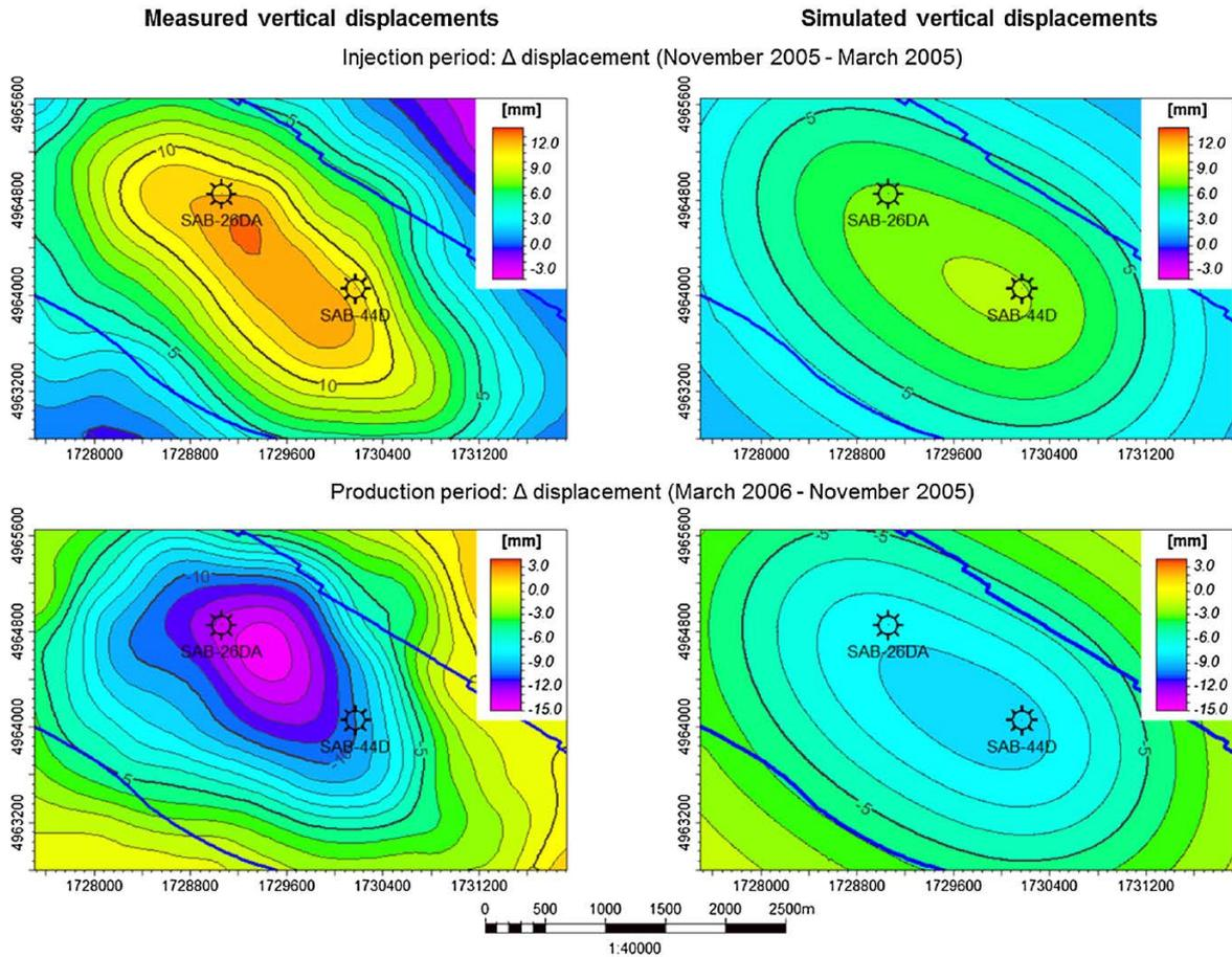
Fig. 5.4: Measured and simulated ground surface displacements above the storage area (Codegone et al., 2016)
