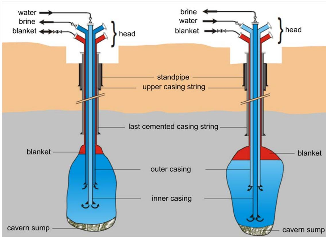
Fig. 2.7: Principles of direct (left) and reverse (right) circulation to create salt caverns (Modified after KBB, 2007)
