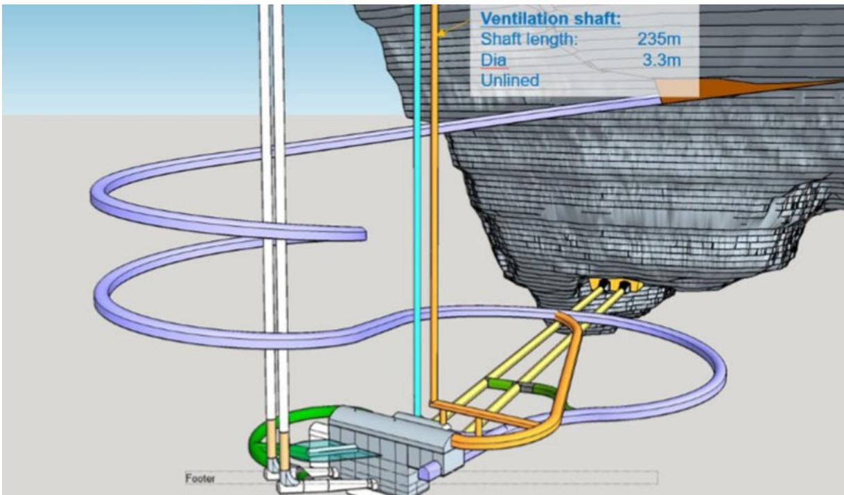
Fig. 4.3: Scheme for underground pumped-storage system in a abandoned mine: The Kidston project in Australia (Reynolds, 2020)
