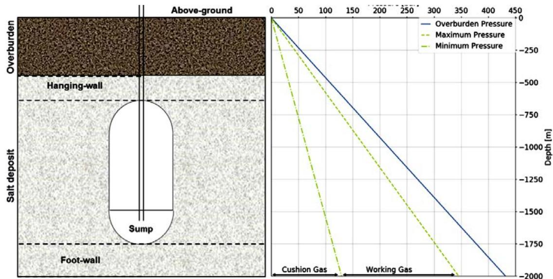
Fig. 2.18: Illustration of general cavern layout and pressure regime used to estimate the hydrogen storage potential (Caglayan et al., 2020)
