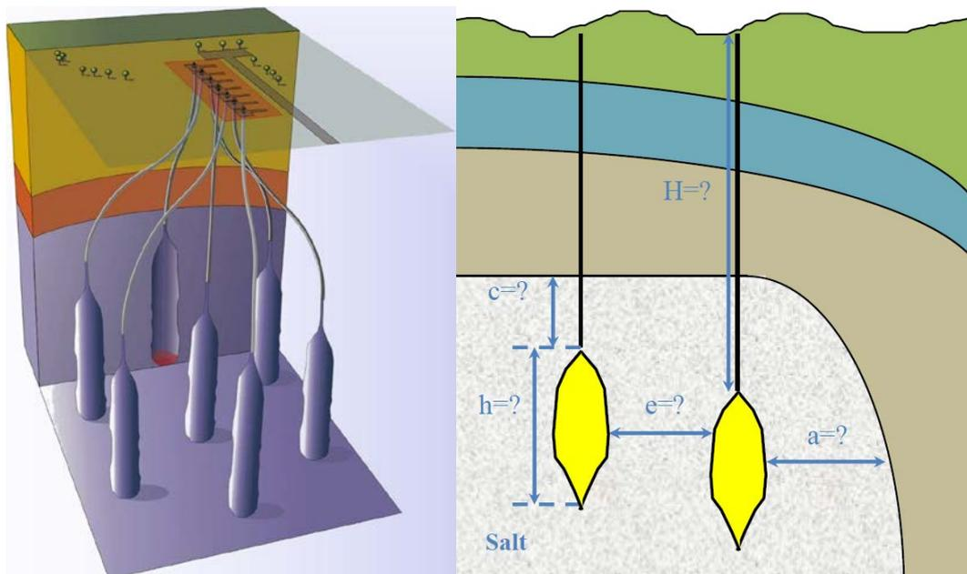
Fig. 2.11: Illustration of a cavern field (company material: KBB) and key geometrical parameters for salt caverns (Hevin, 2019)
