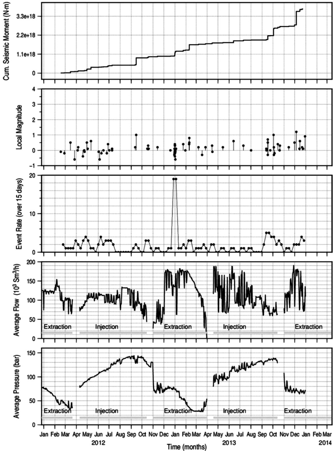
Fig. 5.2: Comparison between seismicity and gas storage activity of the Collalto Stocaggio field (Priolo et al., 2015)
