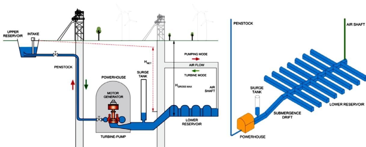
Fig. 4.2: Scheme for underground-pumped-storage system in a abandoned mine (Menéndez et al., 2019)
