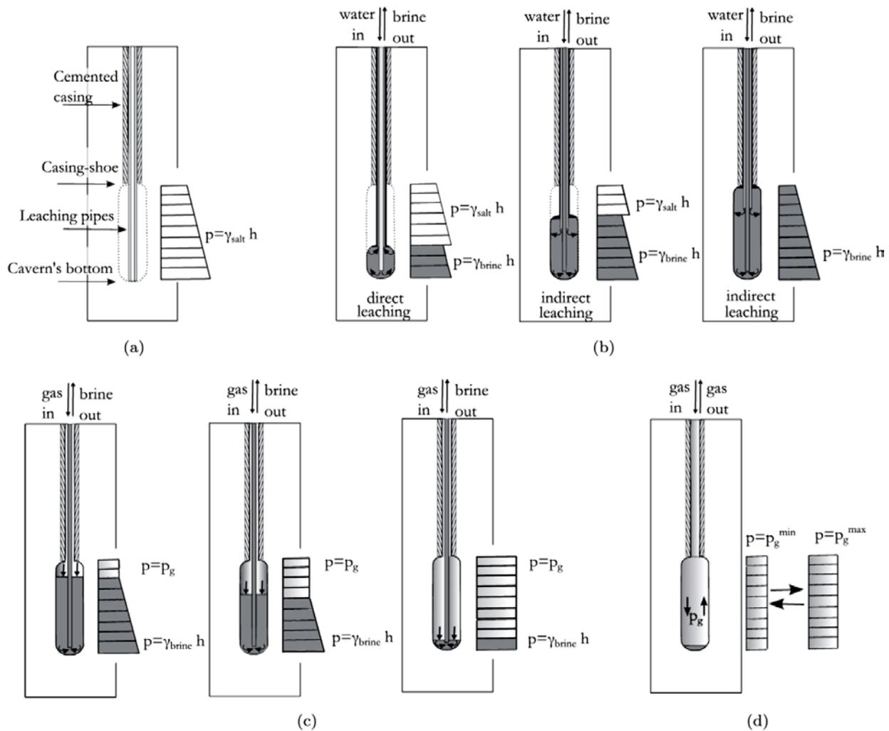
Fig. 2.9: Schematic representation of salt cavern leaching process and subsequent use of cavern under special consideration of acting stresses. a) Virgin stress state prior to the leaching process; b) Leaching process; c) Extraction of brine and injection of storage product; d) First filling and cyclic operation (Khaledi et al., 2016)
