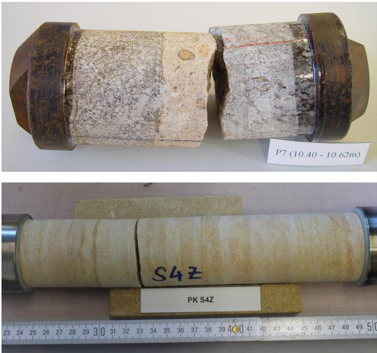
Fig. 6: Uniaxial tension tests: broken samples (gneiss-concrete-interface above, sandstone below) showing clearly developed tensile crack [RML 2016]
