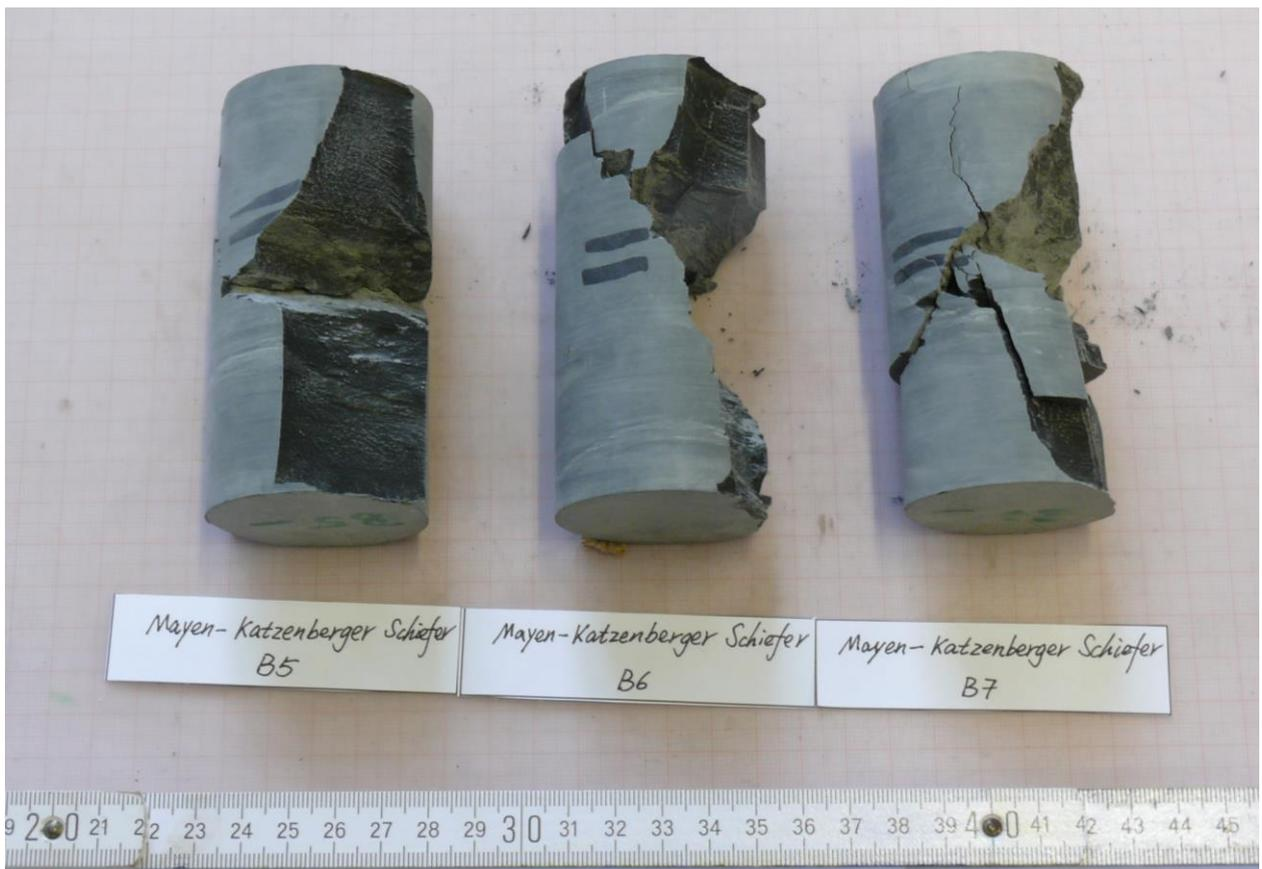
Fig. 10: Uniaxial compression test: mixed-mode shear-tensile fracturing (gneiss above, slate below) [RML 2016]
