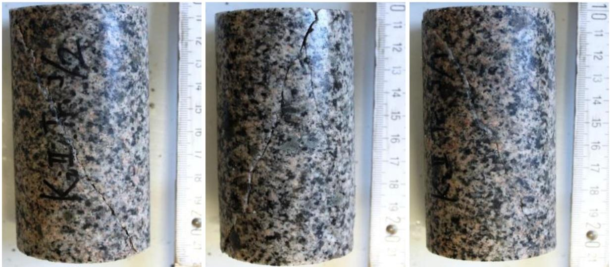
Fig. 11: Triaxial tests: single shear fractures as final fracture pattern, granite samples tested at different confining pressures (10, 20 and 30 MPa)
