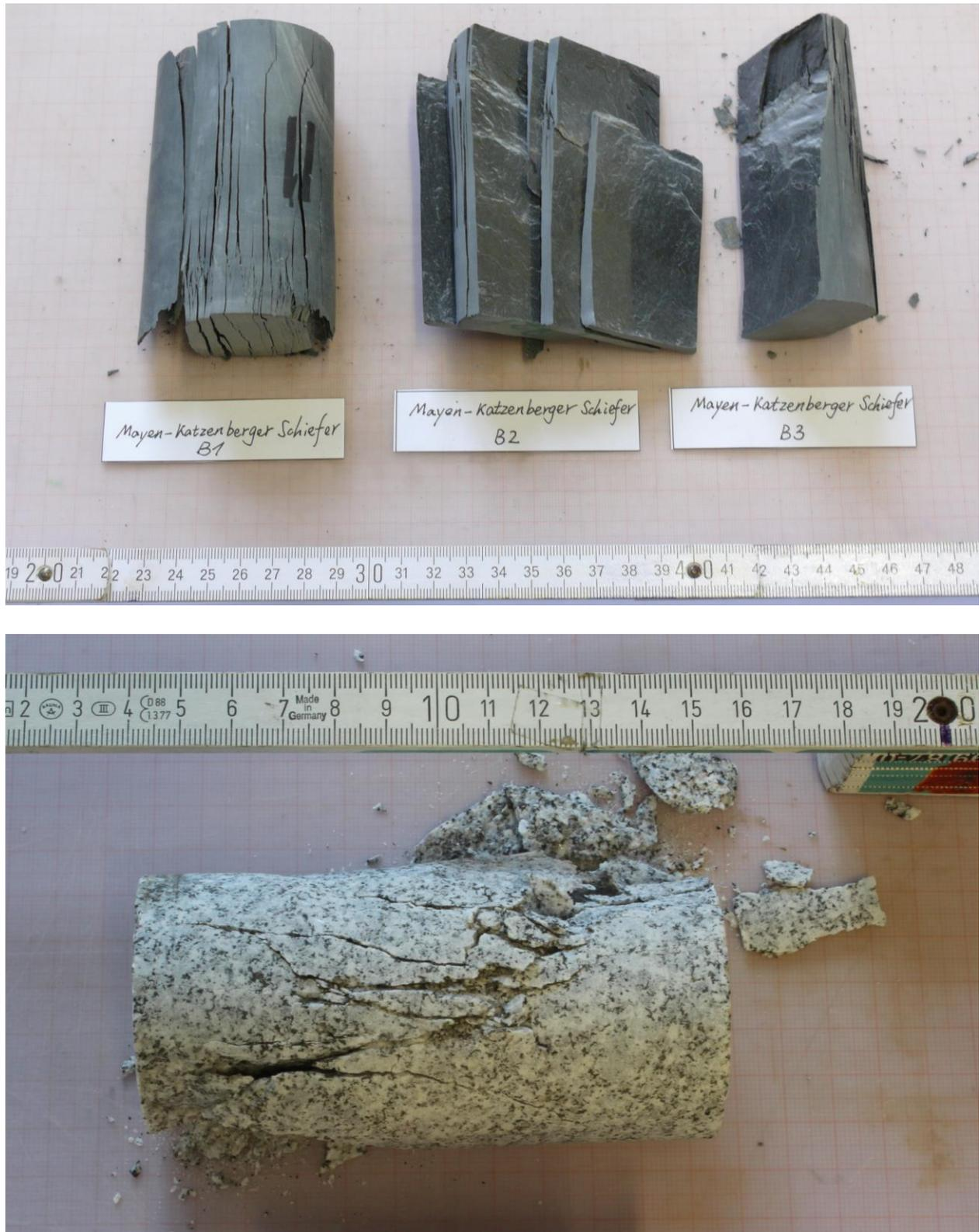
Fig. 7: Uniaxial compression test: vertical splitting (slate above, granite below) [RML 2016]
