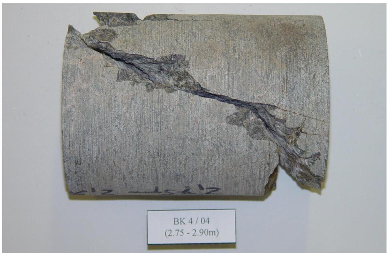
Fig. 8: Uniaxial compression test: single include shear fracture (gneiss above, gneiss below) [RML 2016]
