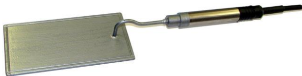
Fig. 4.6.1: Pressure cells (Glötzl, company material)
