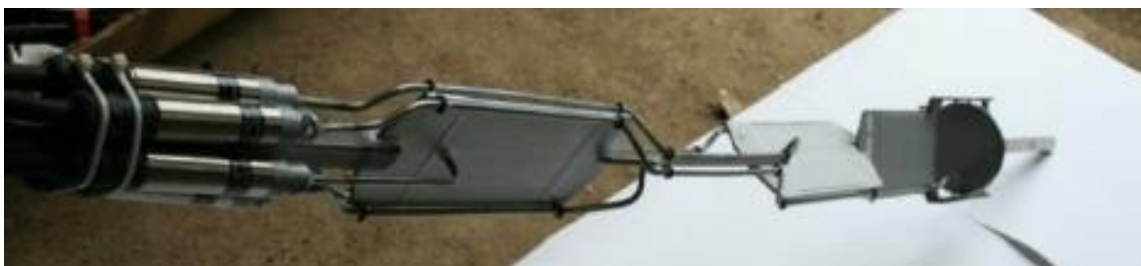
Fig. 4.6.4: Stress monitoring station with four pressure cells (Glötzl, company material)
