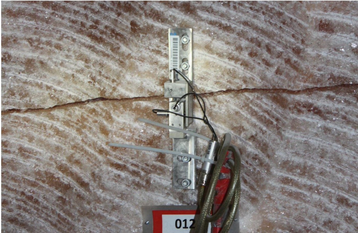
Fig. 4.8.4: Crackmeter (installation in an underground mine)
