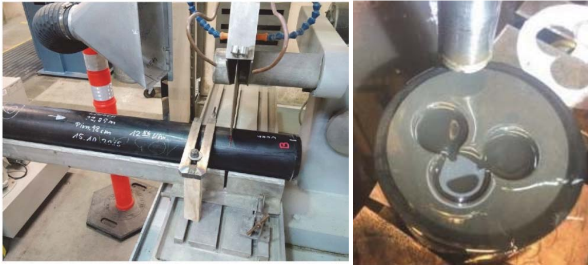
Fig. 7: Extraction of sub-core using a bandsaw (left), and sub-drilling of testing plugs (right).
