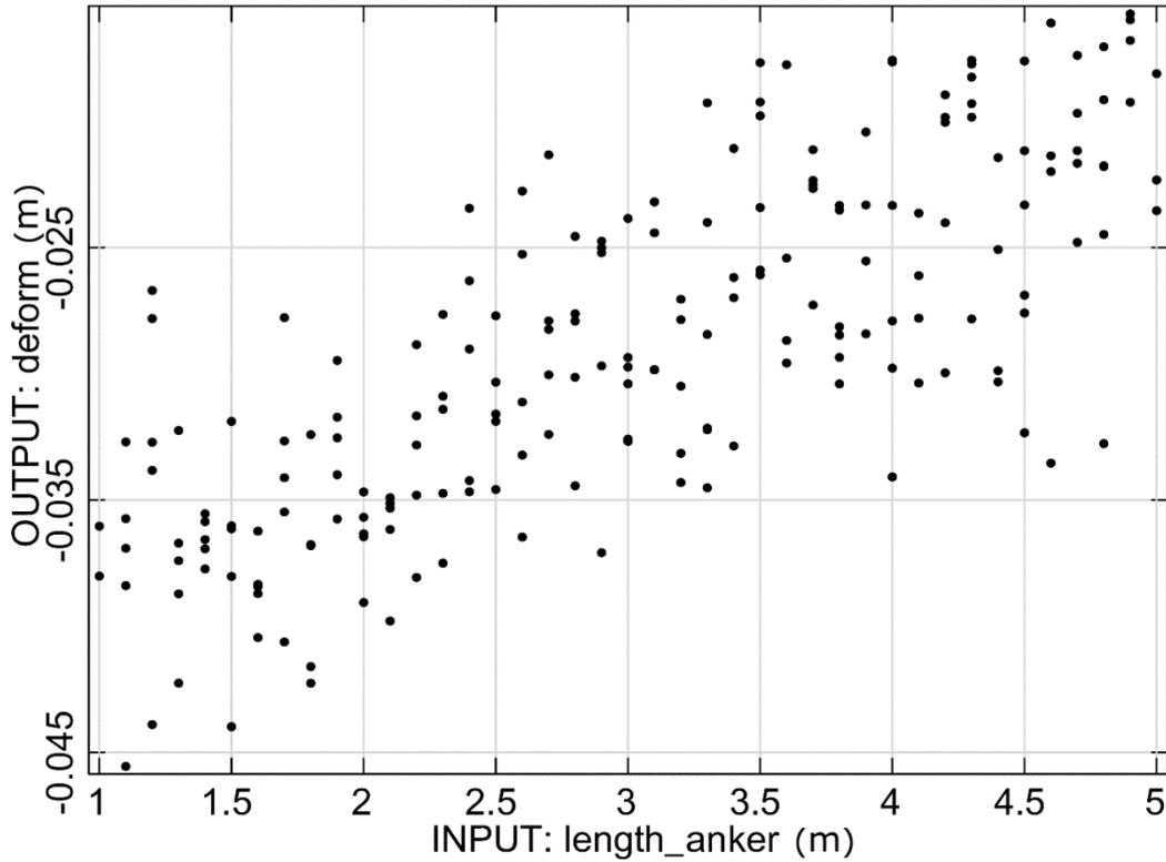
Fig. 6: Anthill-plot: anchor length versus output (maximum roof settlement).
