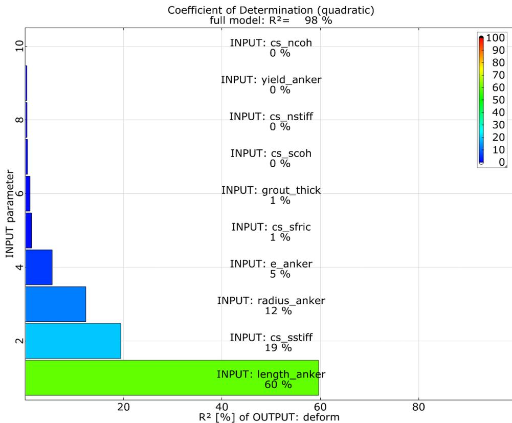
Fig. 7: Coefficient of determination
