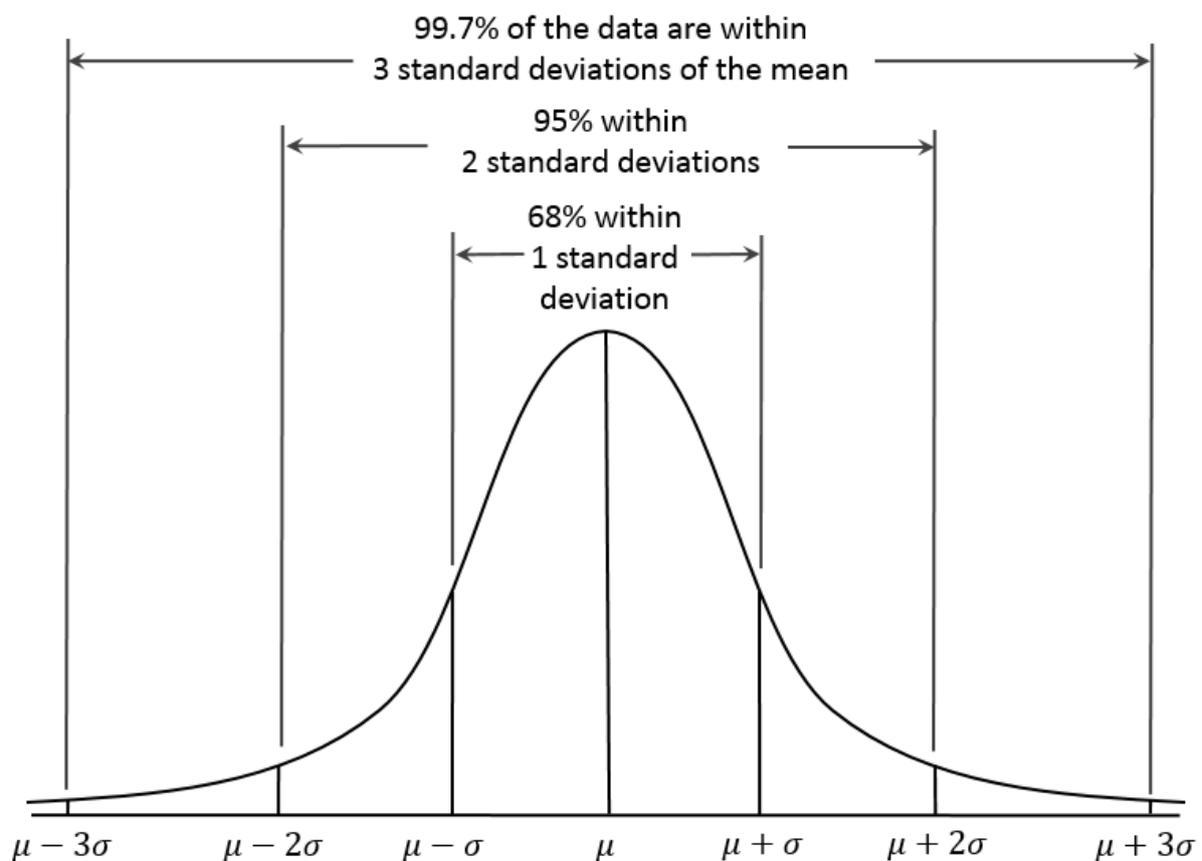
Fig. 3: Illustration of Sigma-levels based on the Gaussian normal distribution
