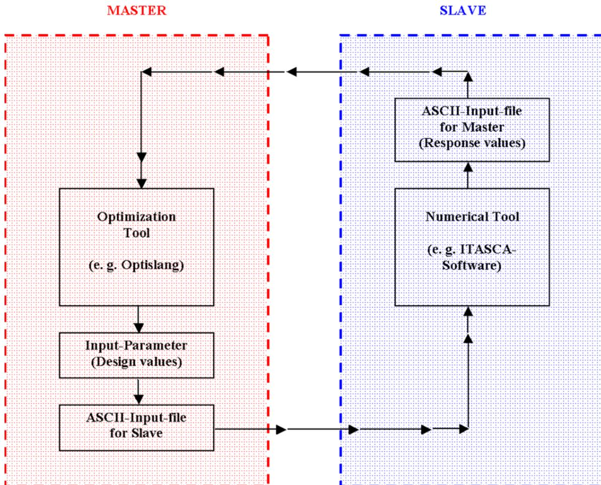
Fig. 5: Work flow of optimization tool and numerical solver in form of a master-slave-modus.
