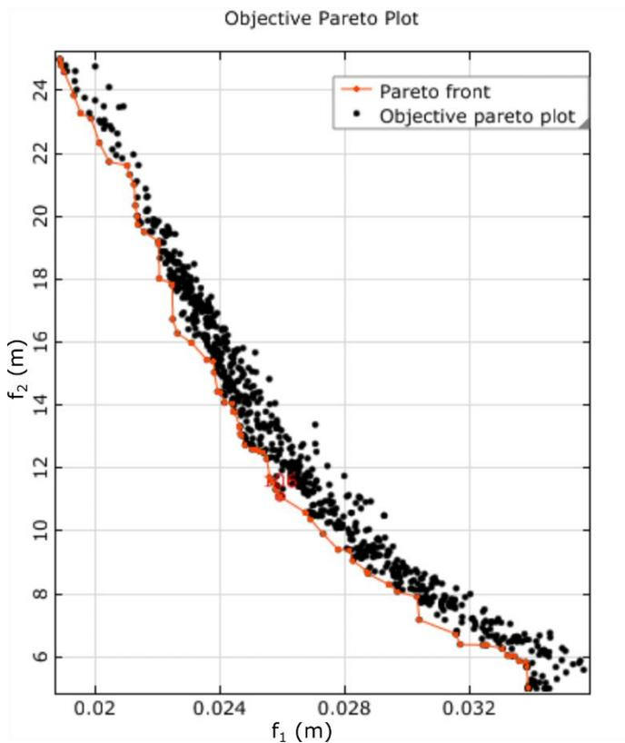
Fig. 12: Roof settlement  $f_1$  versus accumulated anchor length  $f_2$  with indication of best design (No. 106).
