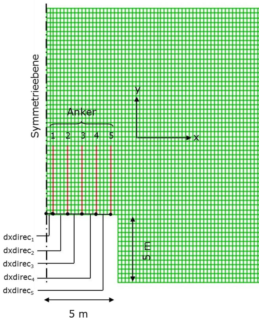
Fig. 4: Numerical model deduced from the rockmechanical problem of roof anchorage (mesh with 5 roof anchors) and variable anchor location.
