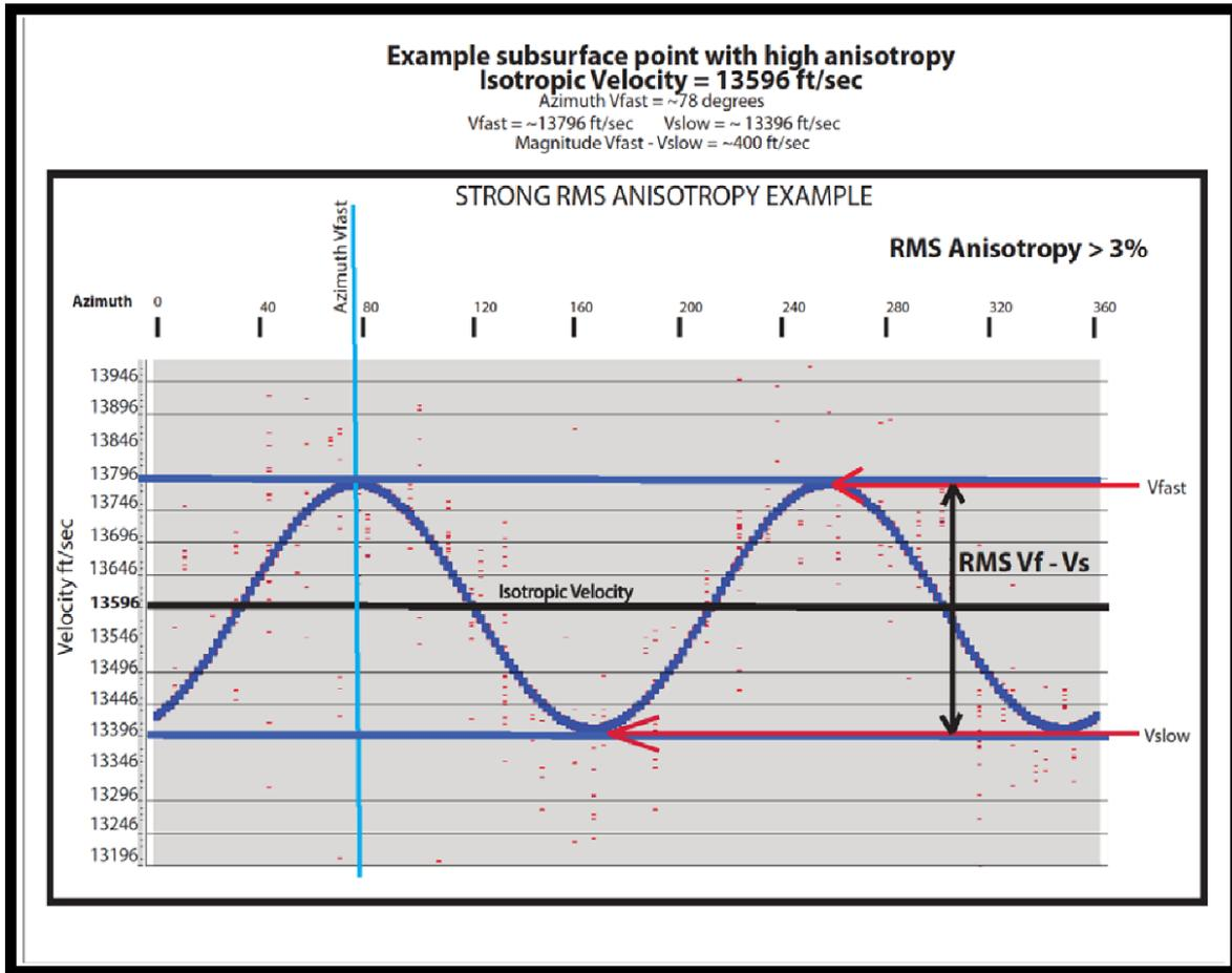
Fig. 14: Example of velocity anisotropy measured at cores (Root mean square of Vfast-Vslow > 3%, Inks et al. 2014)
