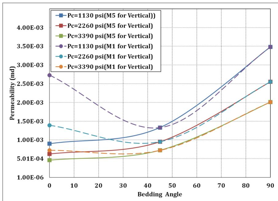
Fig. 13: Permeability anisotropy of Mancos Shale core samples ( $P_c$ : confining pressure; 1 psi = 0,0069 MPa) (Mokhtari et al. 2013)
