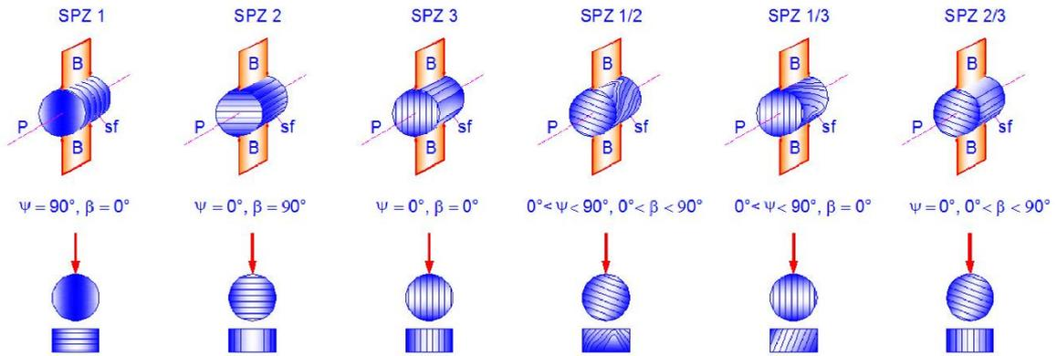
Fig. 6: Experimental arrangement for testing rock anisotropy relative to orientation angle  $\psi$  and foliation - loading angle  $\beta$  using the Brazilian test (Dinh et al. 2013).
