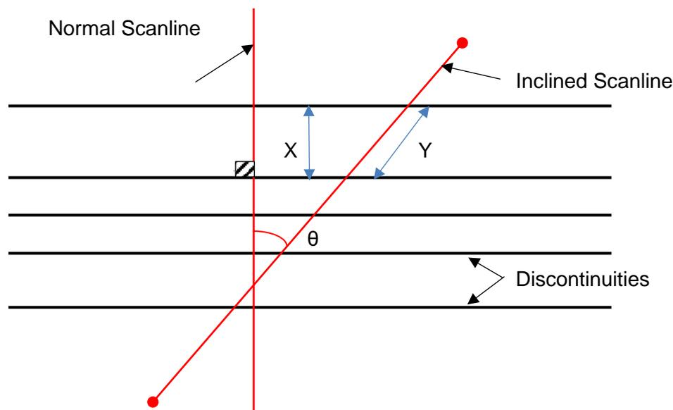
Fig. 3: Two different discontinuities frequencies due to the orientation of the scanlines
