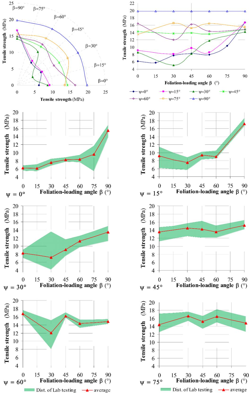
Fig. 7: Tensile strength results Gneiss samples as functions of  $\beta$  and  $\psi$  (Dinh et al. 2013)
