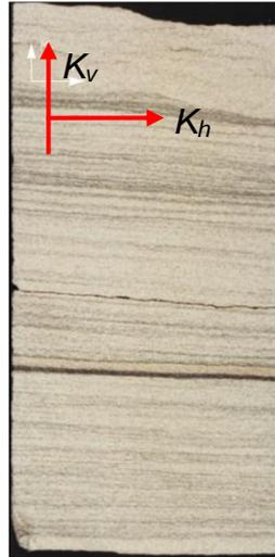
Fig. 12: Sandstone with pronounced permeability anisotropy, where  $k_v/k_h \approx [0.1 \dots 0.5]$  (Ayan et al. 1994)
