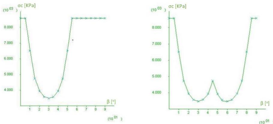
strength of ubiquitous-joint model (cross) versus analytical solution (line)
