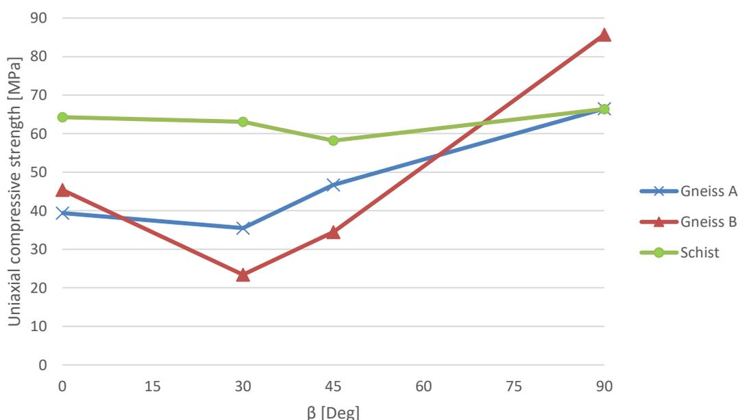
Fig. 4: Uniaxial compressive strength versus orientation angle  $\beta$  (modified after Saroglou and Tsiambaos (2008))
