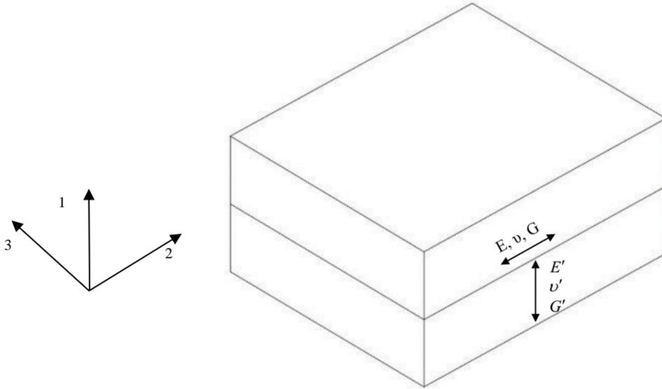
Fig. 16: Schematic of the transverse isotropy and this model parameters
