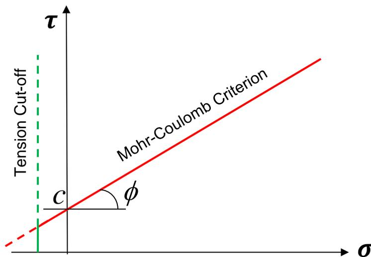
Fig. 17: Mohr-Coulomb failure criterion with a tension cut-off
