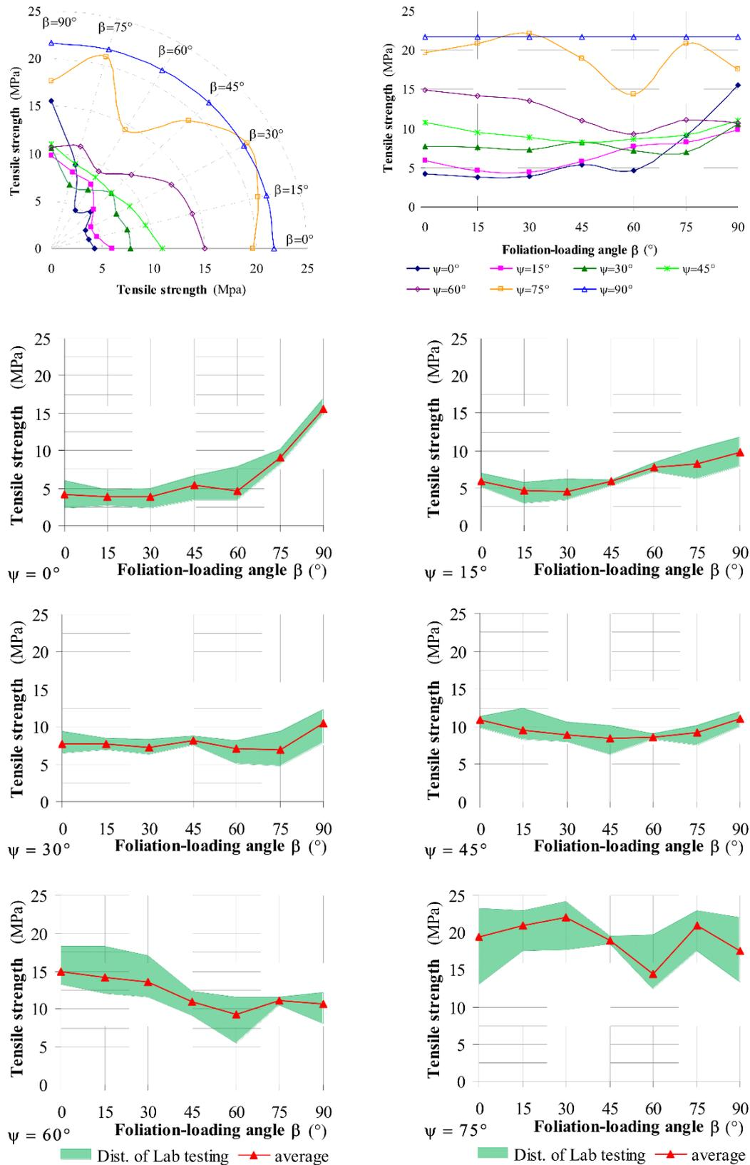
Fig. 8: Tensile strength results of Slate samples as functions of  $\beta$  and  $\psi$  (Dinh et al. 2013)
