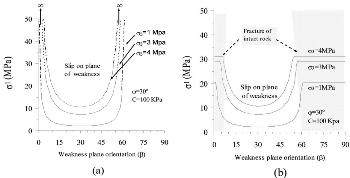
Fig. 5: Strength anisotropy: (a) theoretical solution according to Eq. 1, (b) realistic shoulder-shaped anisotropy (Bagheripour et al. 2011)
