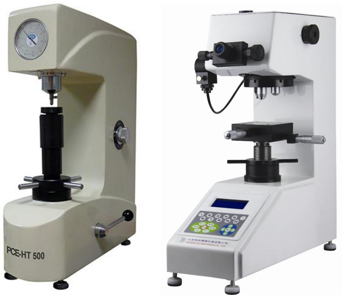
Fig. 3.1.4: Typical hardness testing devices [company leaflets]
