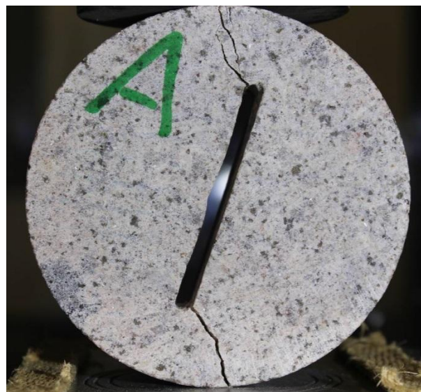
Fig. 3.15.3: Test set-up for CCNBD test [RML 2016]
