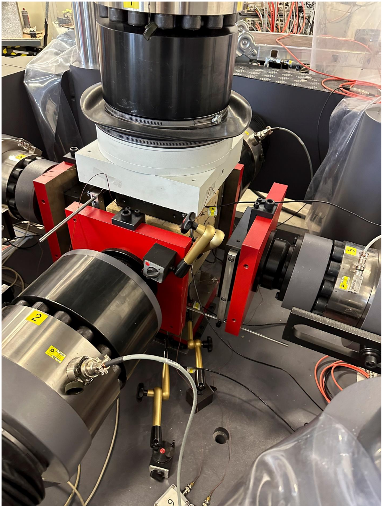
Fig. 3.13.1: Large true triaxial testing device [RML 2023]
