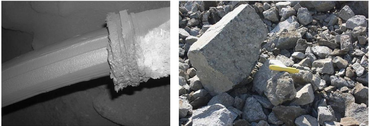
Fig. 1: Different types of backfill, left: paste fill; right: rock fill (Sivakuga et al. 2015)
