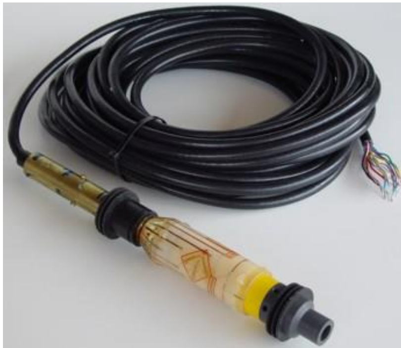
Fig. 4.2: CSIRO-HI-Cell based on over-coring technology (company material)
