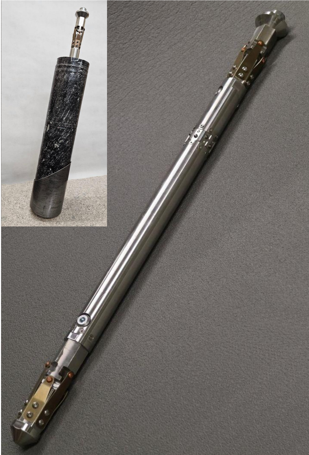
Fig. 4.10: Overcoring probe measuring 4 diametric convergences with 8 sensors (company material)
