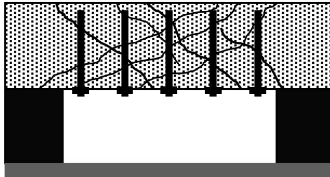
Fig. 2.3: Wedging effect mechanism
