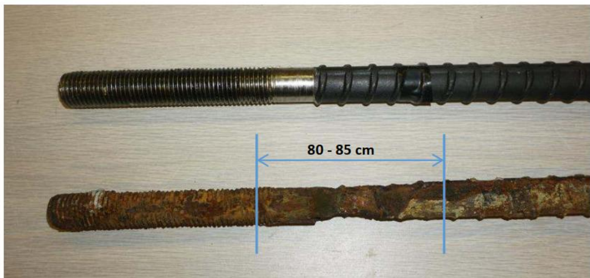
Fig. 6.14: Echo puls method: abnormal energy ratio between 80 and 90 cm indicates corrosion of rockbolt (Medfouni et al. 2015)
