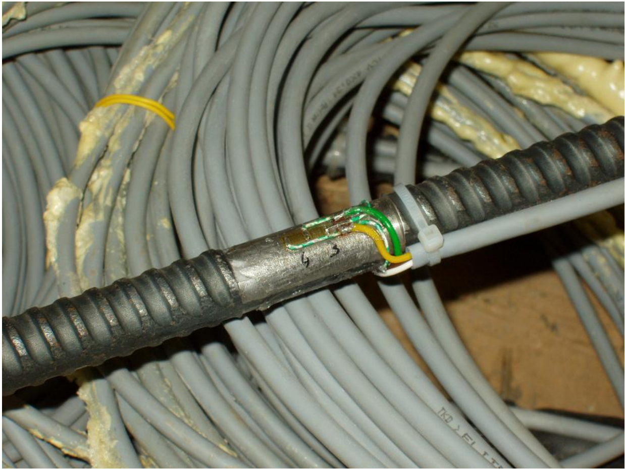
Fig. 6.9: Anchor with applied DMS for monitoring of axial load (Frühwirth et al. 2008)
