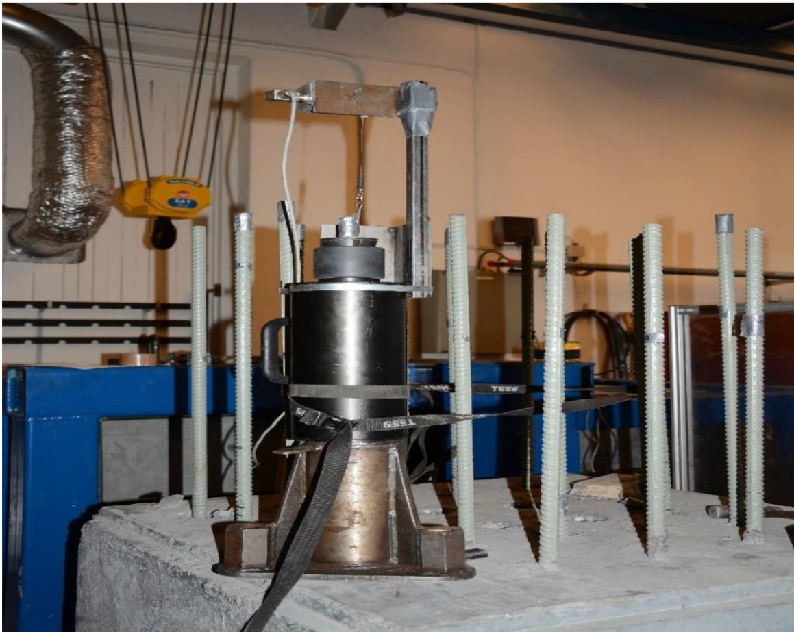
Fig. 6.2: Lab test set-up for pull-out-test (Kristjansson 2014)
