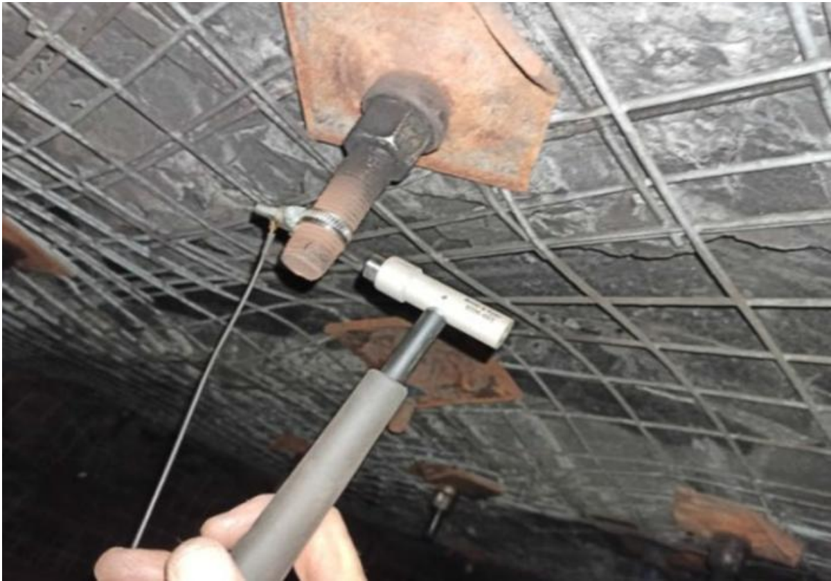
Fig. 6.15: Ultrasonic anchor measurement with impact hammer (Staniek, 2023)
