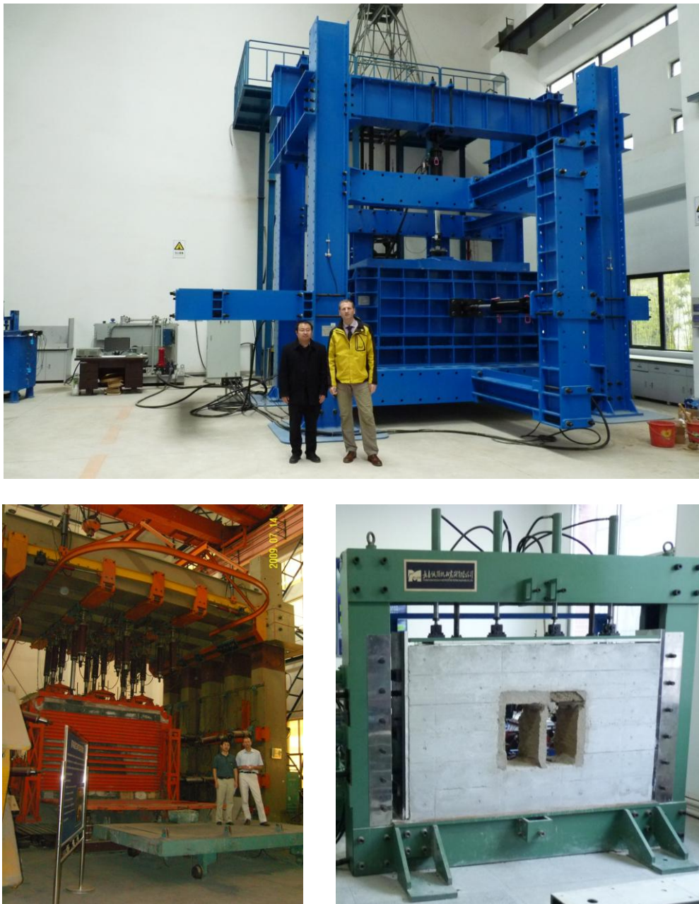
Fig. 5.1: Different loading frames (China)
