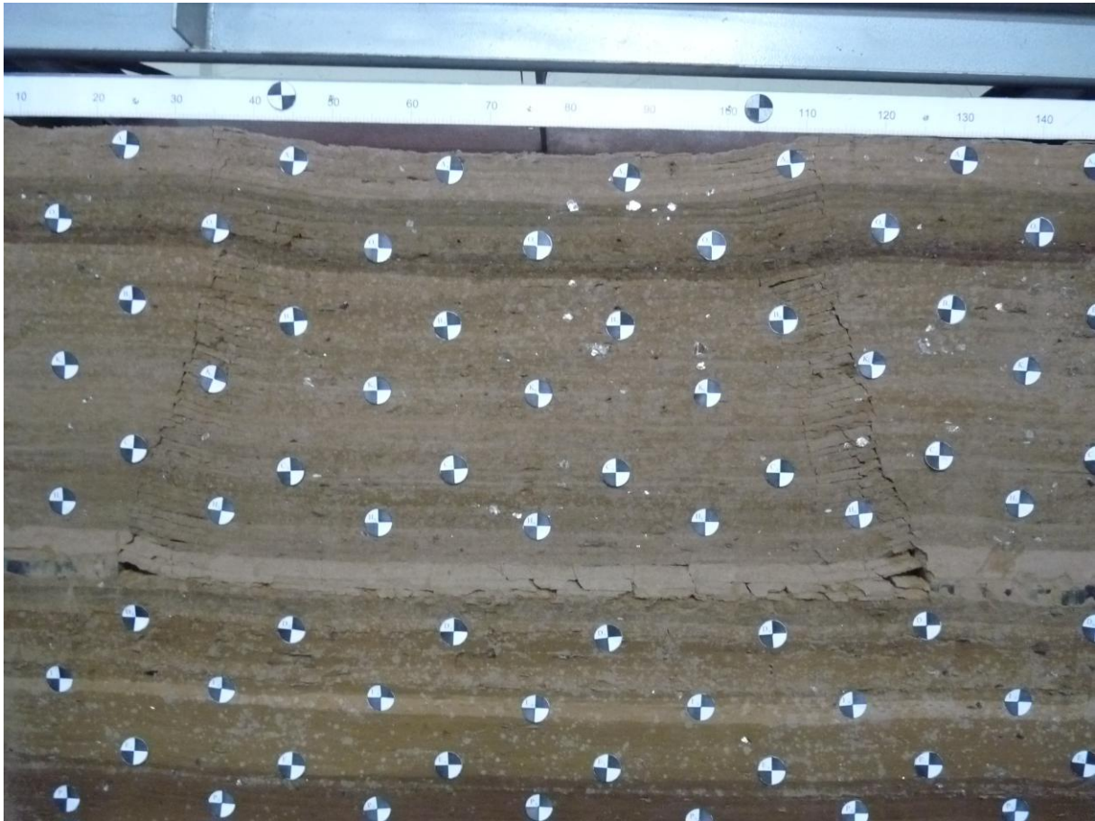
Fig. 3.2: Physical model prepared with point markers to monitor movements (China)
