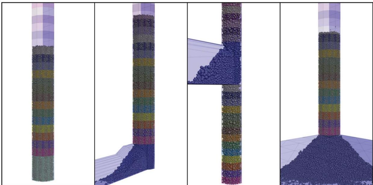
Fig. 5.2: Simulation of backfilling a shaft without and with connected drifts (Nguyen, 2016)
