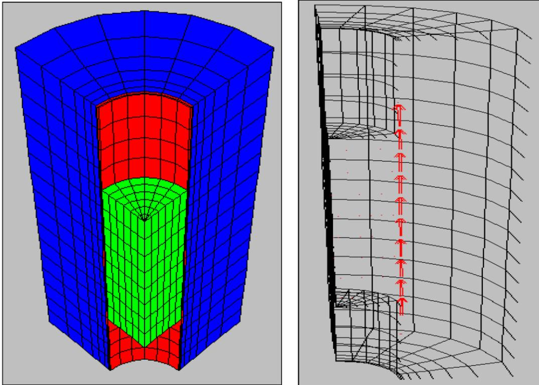
Fig. 6.2: Numerical model to investigate tightness of shaft sealing for compressed air storage in an abandoned salt mine (left: blue: salt rock mass, red: EDZ, green: sealing construction; right: flow vectors) (Hausdorf & Konietzky 2009)
