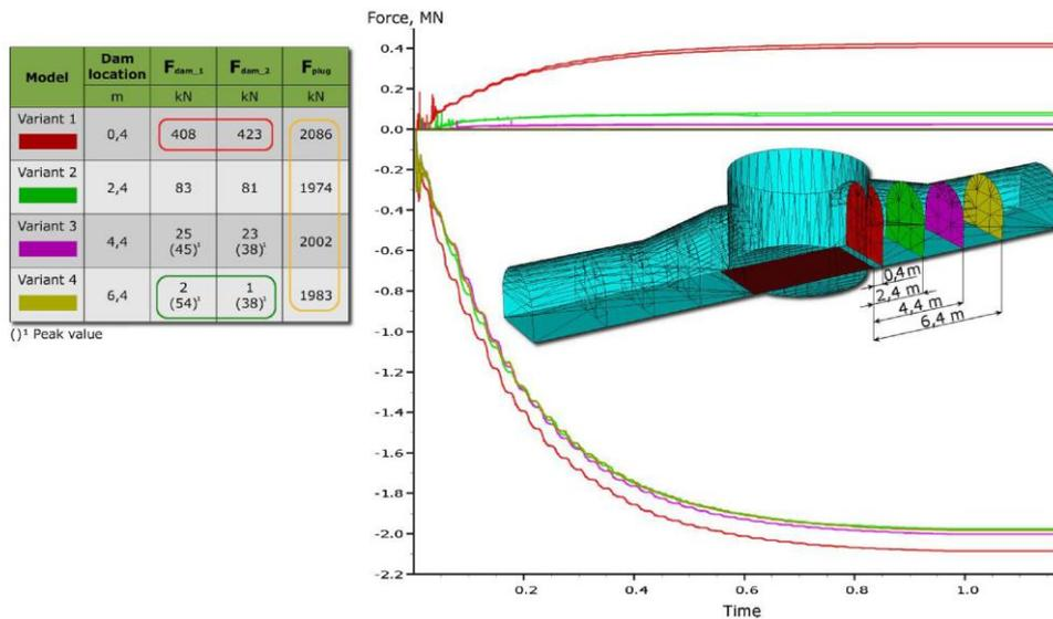
Fig. 5.6: Calculated forces on dams caused by ballast for dams at different locations (Bock & Prusek, 2015)
