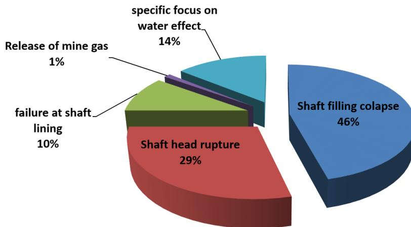
Fig. 1.2: Shaft failure analysis (after: Salmon et al., 2015)
