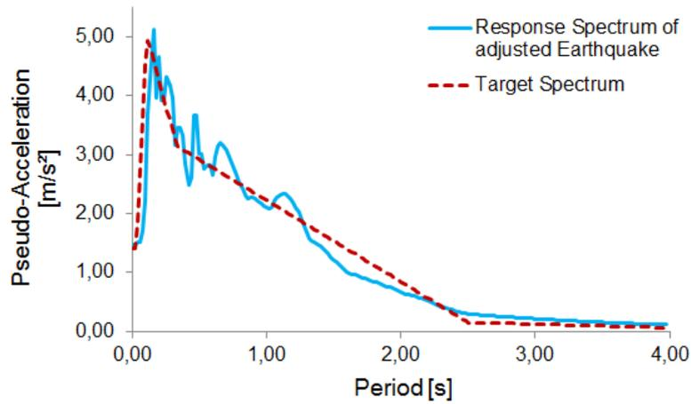
Fig. 6.10: Response spectrum for design earthquake (Neubert, 2014)
