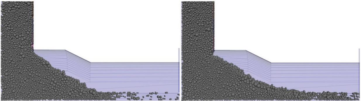
Fig. 5.3: Simulation of backfilling with lower (left) and higher (right) falling height of ballast (Nguyen, 2016)
