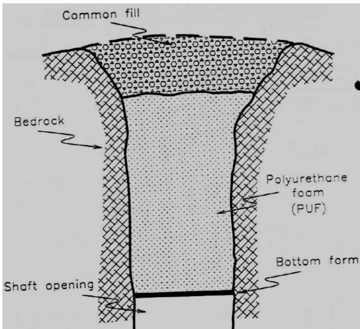
Fig. 4.2: Typical polyurethane plug (Heath, 2009)
