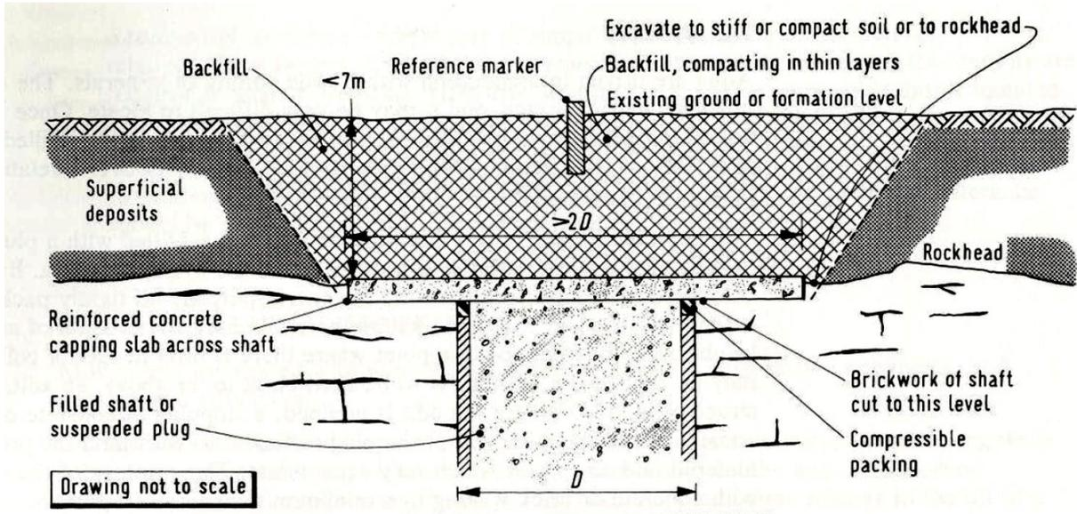
Fig. 4.1: Typical concrete cap (Heath, 2009)
