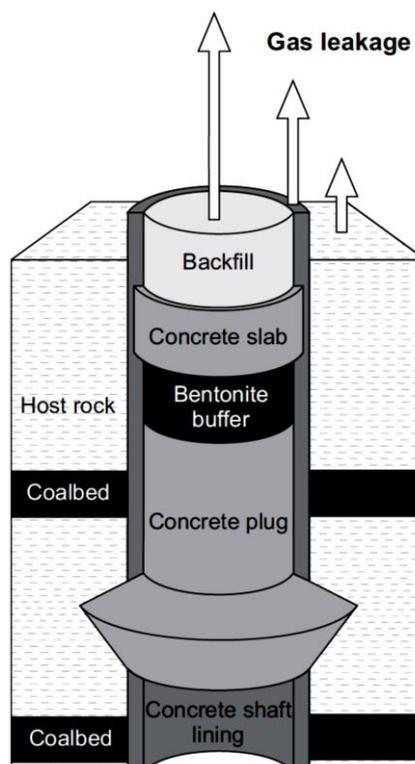
Fig. 6.1: Layout of coal shaft sealing (Bertrand et al., 2015; Dieudonne et al. 2015)
