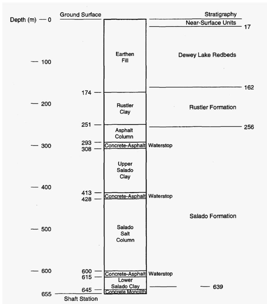
Fig. 6.9: Layout of the WIPP site air intake shaft sealing (Sandia, 1997)
