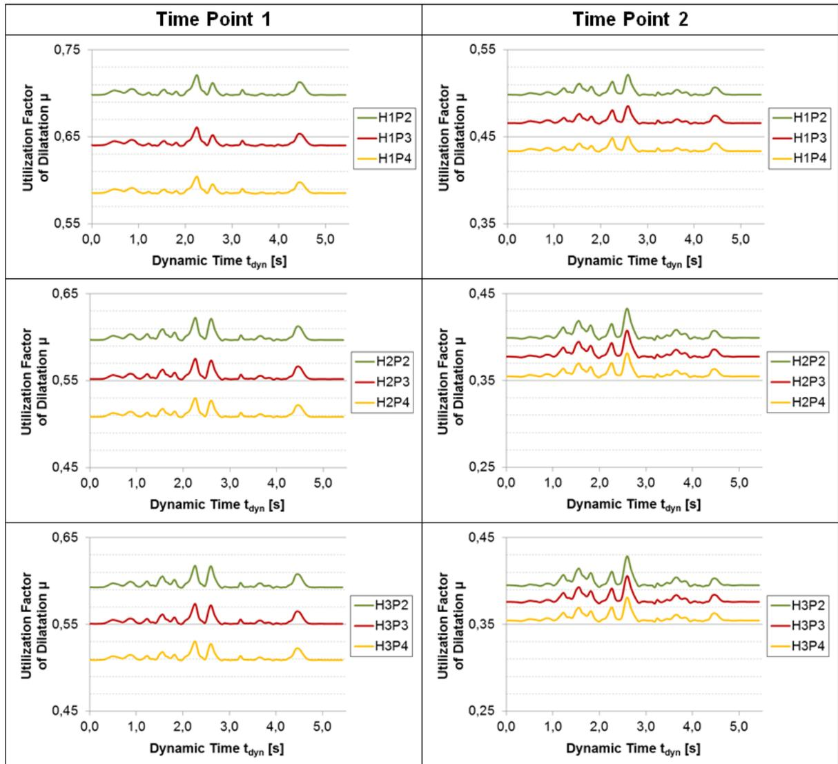
Fig. 6.14: Utilization factor according to Fig. 6.13 during earthquake impact 2 (time point 1) and 20 years (time point 2) after installation of the shaft sealing (Neubert, 2014)
