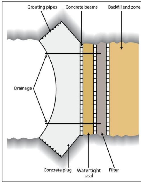
Fig. 6.8: SKB reference conceptual design for tunnel sealing (Hansen et al., 2016)
