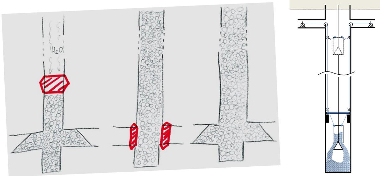
Fig. 4.4: Different shaft sealing options (red: dam), right: ballast filling procedure
