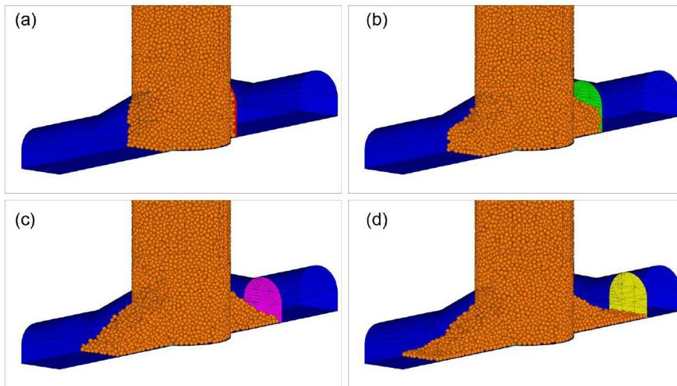
Fig. 5.5: Simulation of shaft sealing considering different positions of a dam (Bock & Prusek, 2015)
