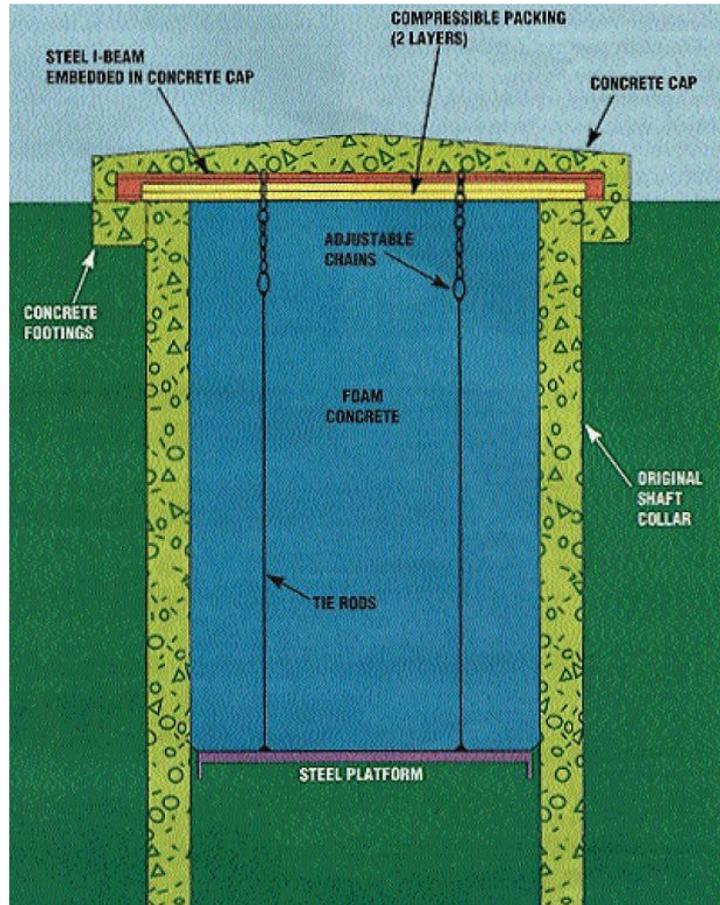
Fig. 4.5: Shaft sealing with foam-concrete plug and cap (Koski, 1994)
