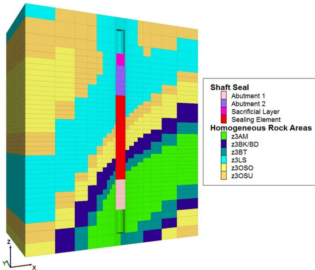
Fig. 6.12: 3-dimensional numerical model for dynamic visco-elasto-plastic simulations (Neubert, 2014)
