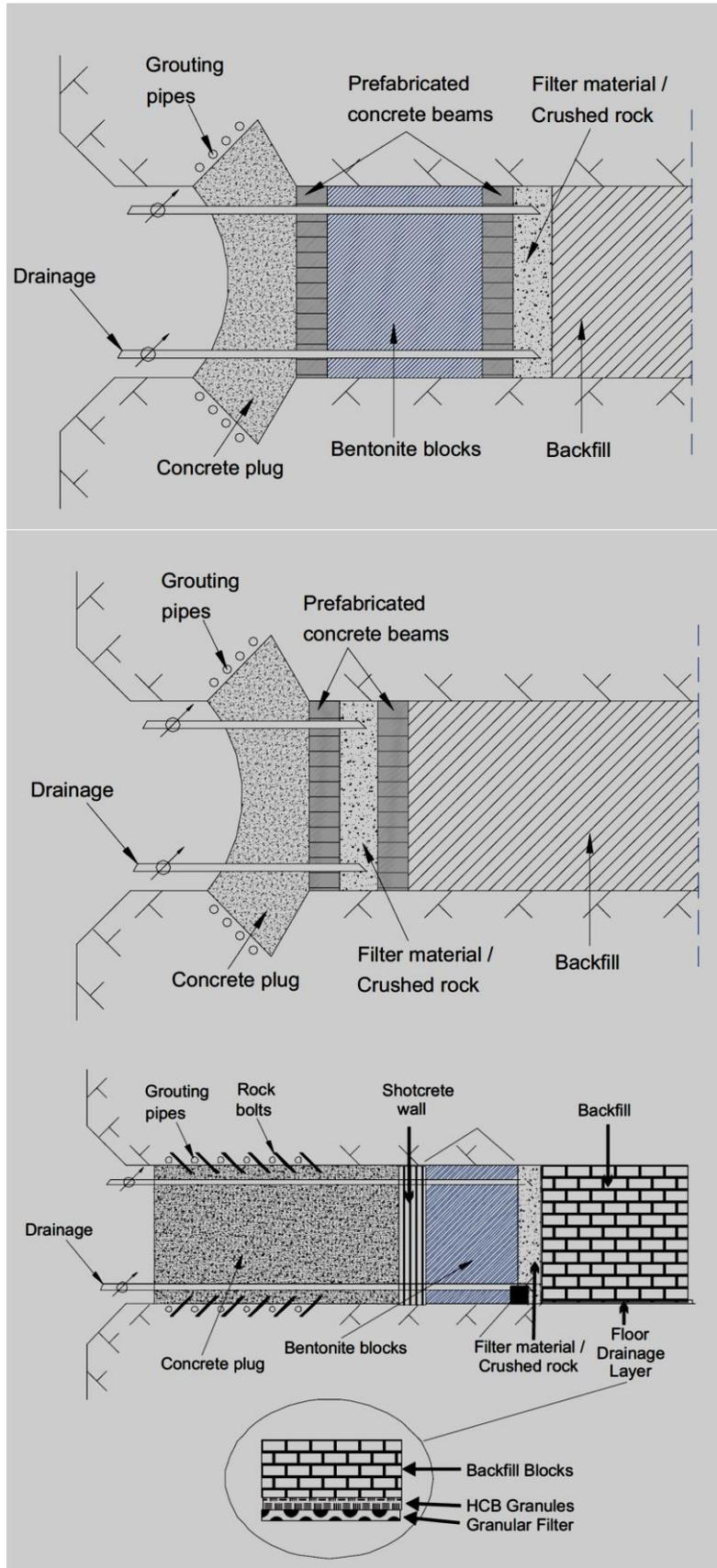
Fig. 6.7: Different tunnel (drift) sealing concepts (Dixon et al., 2009)
