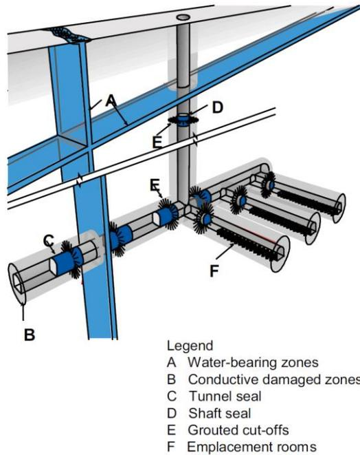
Fig. 6.5: General radioactive waste repository layout with indication of sealing constructions (Dixon et al., 2009)
