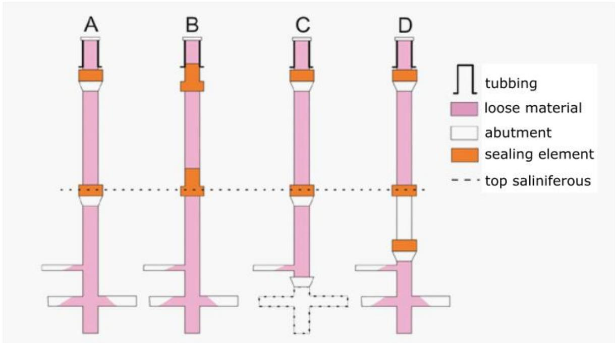
Fig. 6.3: Layout of salt mine shaft sealings (modified after Bartl, H. et al., 2003)
