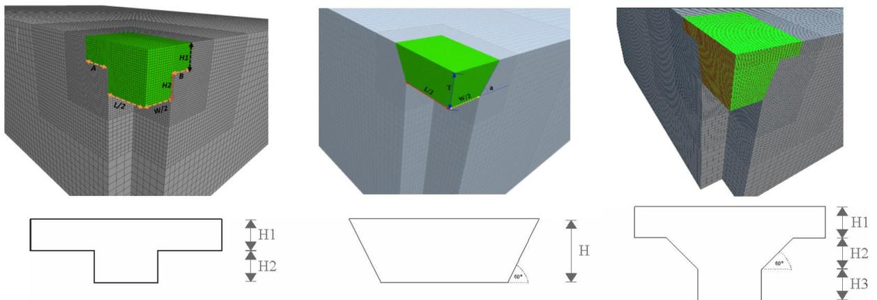
Fig. 4.6: Shaft concrete capping options investigated via numerical modelling (Konietzky et al., 2014)
