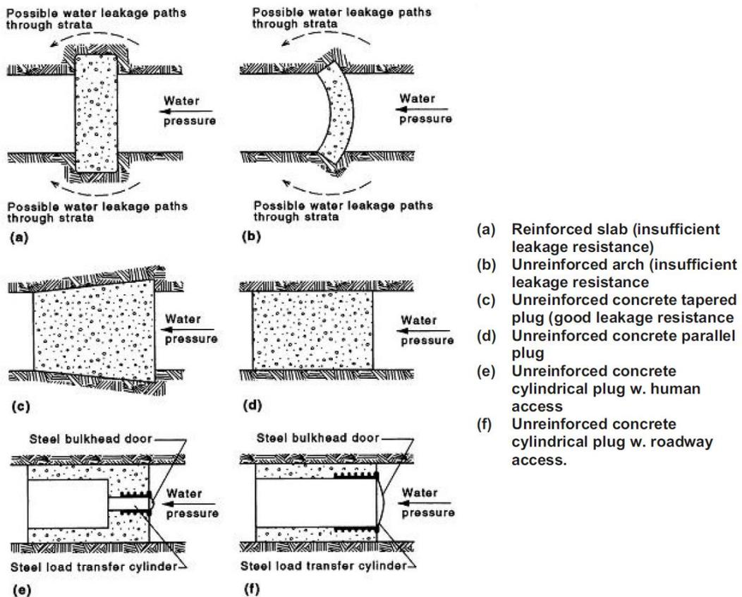
Fig. 6.6: Different plug types for tunnel (drift) sealings (Dixon et al., 2009)
