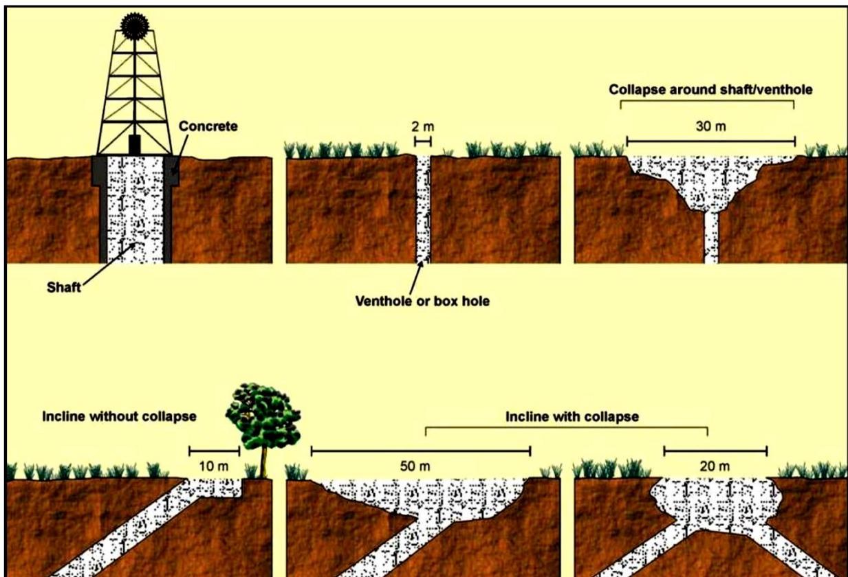
Fig. 1.1: Typical examples of openings which need sealing (Heath, 2009)
