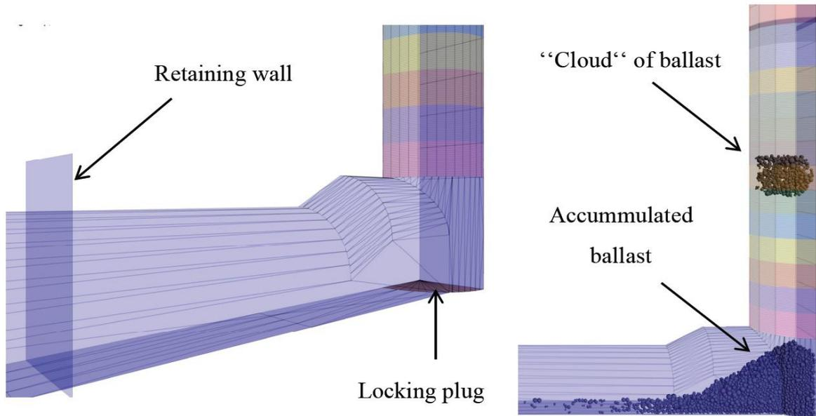
Fig. 5.1: Simulation of backfilling a shaft with connected drift (Nguyen, 2016)
