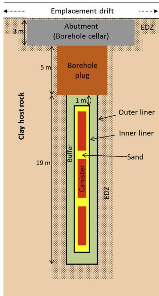
Fig. 6.15: Sealing concept for radioactive waste repository in clay (top: overview, bottom: sealing concept for emplacement borehole) (Jobmann et al., 2017)
