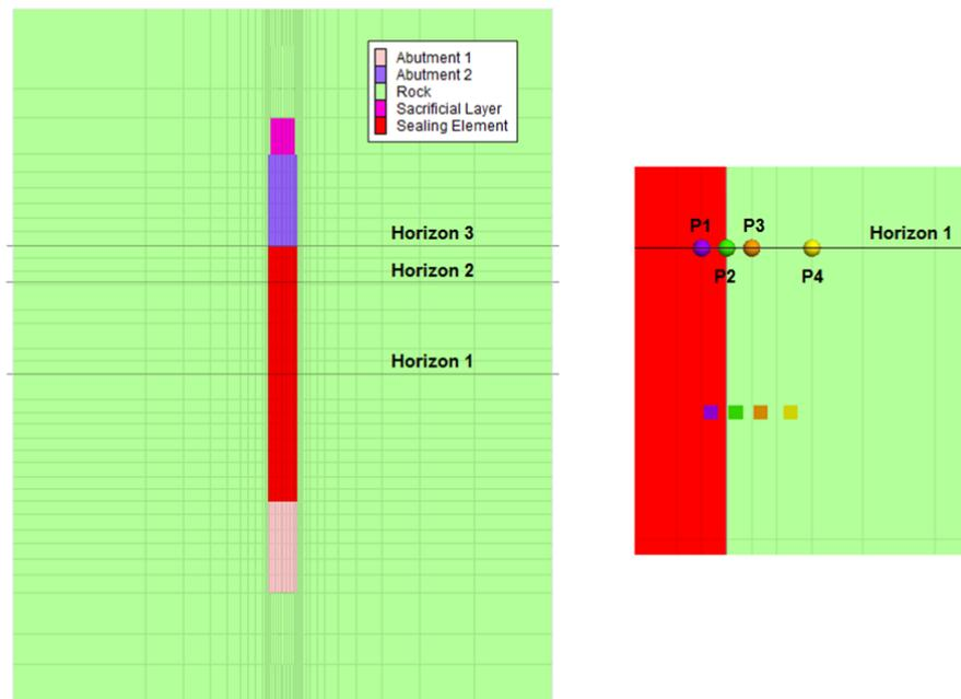
Fig. 6.13: Vertical cross section through numerical model with indication of observation points (Neubert, 2014)
