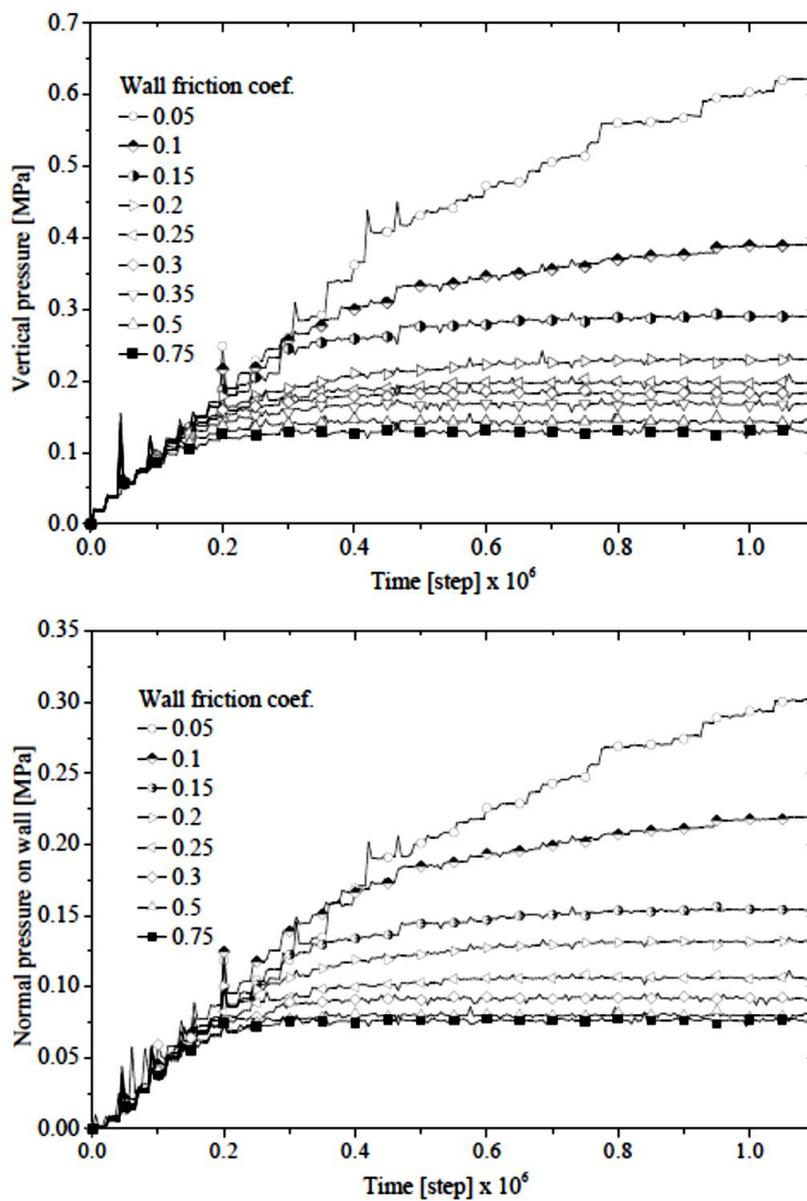
Fig. 5.4: Vertical and horizontal (wall) pressure as function of wall friction (Nguyen, 2016)
